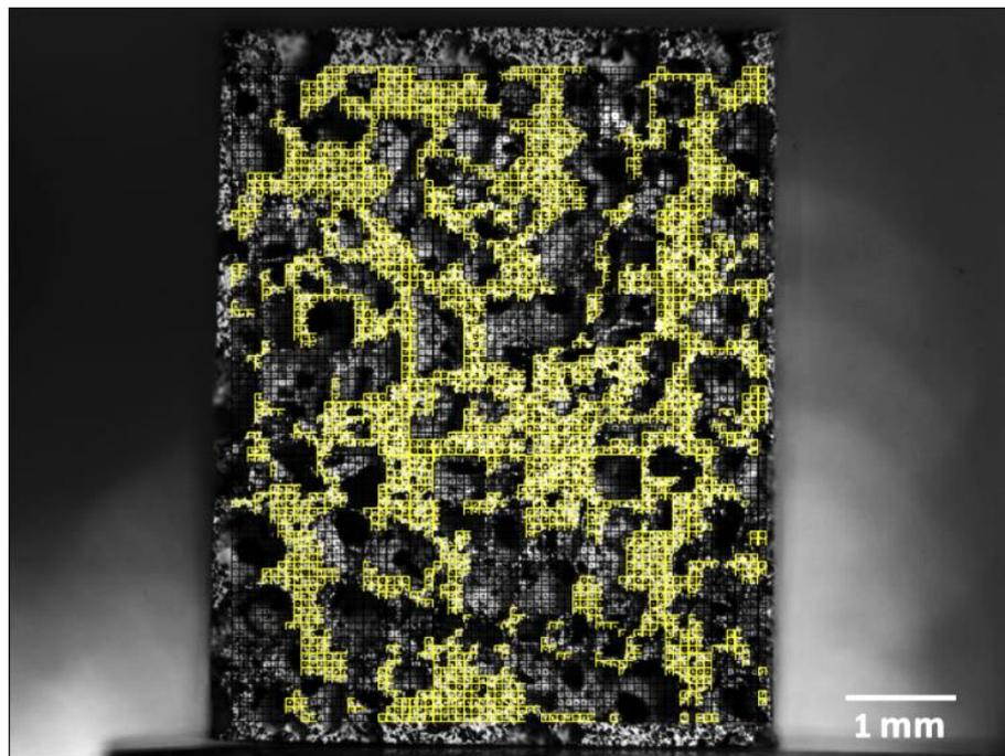
Fig. 2.65 Points and correlation domains defined on reference image for computing microscopic strain maps of aluminum foam sample Al01 under uniaxial compression.
