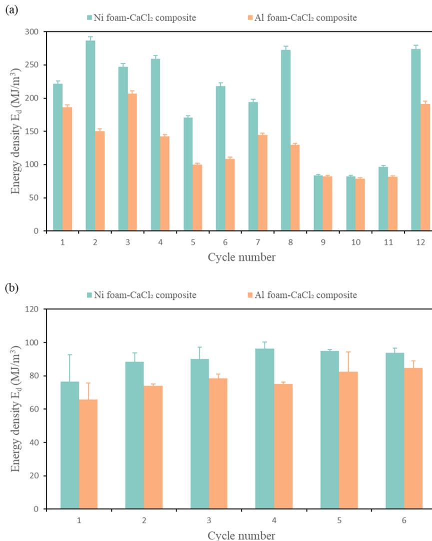
Fig. 3.19. The apparent energy density of nickel foam-CaCl<sub>2</sub> composite and aluminum foam-CaCl<sub>2</sub> composite in (a) 12 hydration/dehydration cycles of different hydration duration and in (b) 6 hydration/dehydration cycles of 45 min hydration duration.
