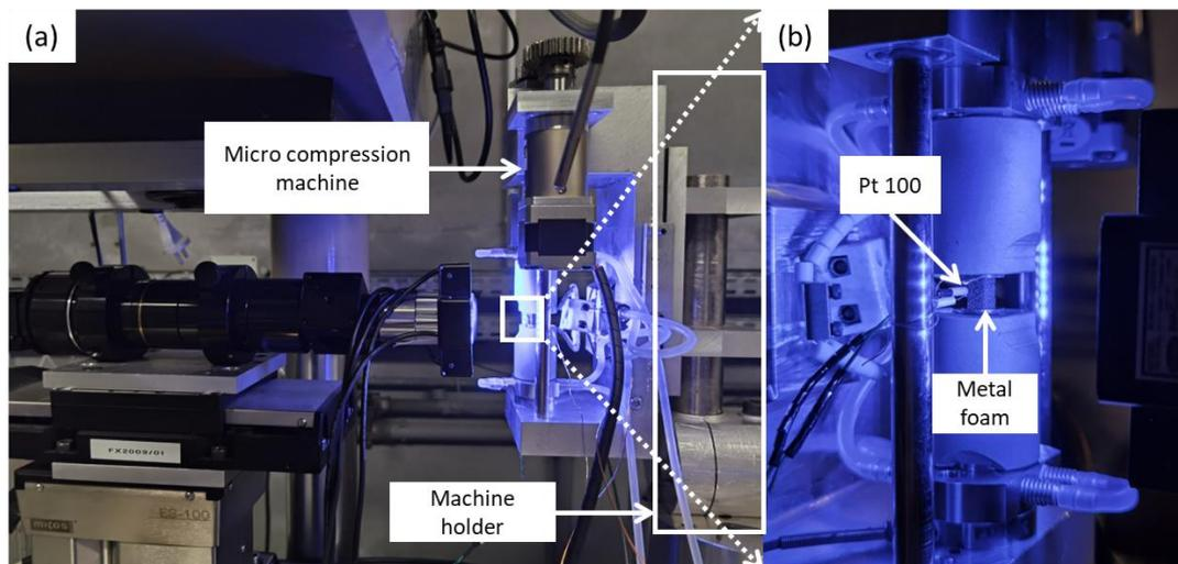
Fig. 2.12 Photo of (a) the global view of the in situ uniaxial compression test setup with an observation by optical microscopy and (b) zoom on the metal foam sample.
