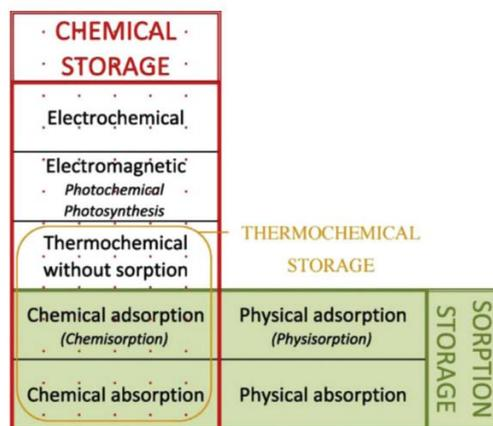
Fig. 1.6 Classification of chemical storage and sorption storage [38].
