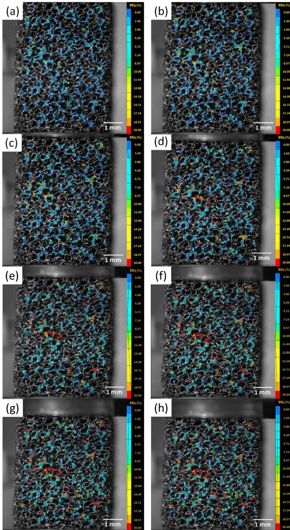
Fig. 2.55 Equivalent deformation maps at eight levels of macroscopic strain of the sample Cu<sub>2</sub>O during compression (vertical) at 150 degrees with (a) at 1% (b) at 2.4% (c) at 4% (d) at 7% (e) at 10% (f) at 12% (g) at 14% and (h) at 15%.
