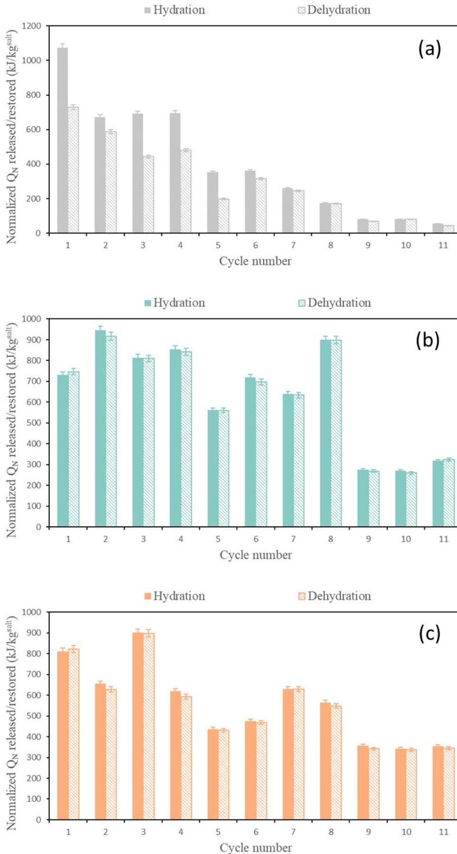
Fig. 3.17 Normalized thermal energy released/stored during long cyclic hydration/dehydration process of (a) bulk  $CaCl_2$  powder, (b) nickel foam- $CaCl_2$  composite and (c) aluminum foam- $CaCl_2$  composite.
