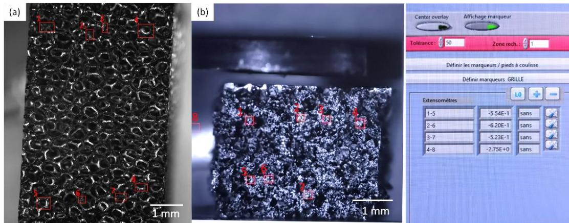
Fig. 2.13 (a) 8 square markers selected on the reference image of a copper foam sample. (b) 8 markers on the deformed image of an aluminum foam sample with mean strain during loading between markers 1-5, 2-6, 3-7 and 4-8 displayed on the right side of the software interface in real-time.
