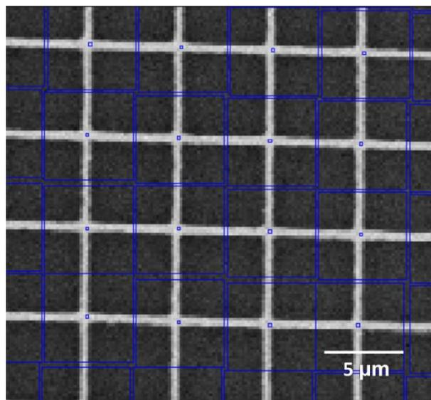
Fig. 2.84 The measurement points placed on the intersections of the grids, with small blue squares representing the measurement point and the big blue squares representing the correlation domain.
