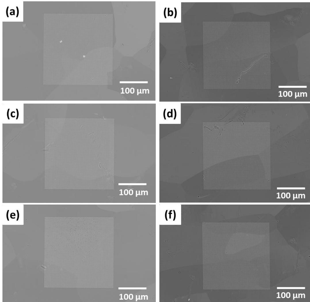
Fig. B.7. BSE images of pattern Diamonds (Fig. 2.22d) realized at accelerating voltage of 15 kV with dose factors of (a) 1.0, (c) 1.2, (e) 1.4, and at accelerating voltage of 25 kV with dose factors of (b) 1.0, (d) 1.2, (f) 1.4.
