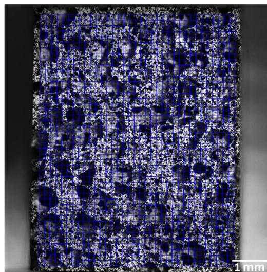
Fig. 2.62 Matrix of the measurement points defined and correlation domains in size of  $50 \times 50$  pixels for computing the strain field at the metal foam structural scale of pores of Al01.
