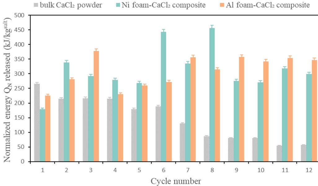
Fig. 3.11. Normalized thermal energy released during the first 45 min of each humidification process for 12 hydration/dehydration cycles of nickel foam- $\text{CaCl}_2$  composite, aluminum foam- $\text{CaCl}_2$  composite and bulk  $\text{CaCl}_2$  powder.
