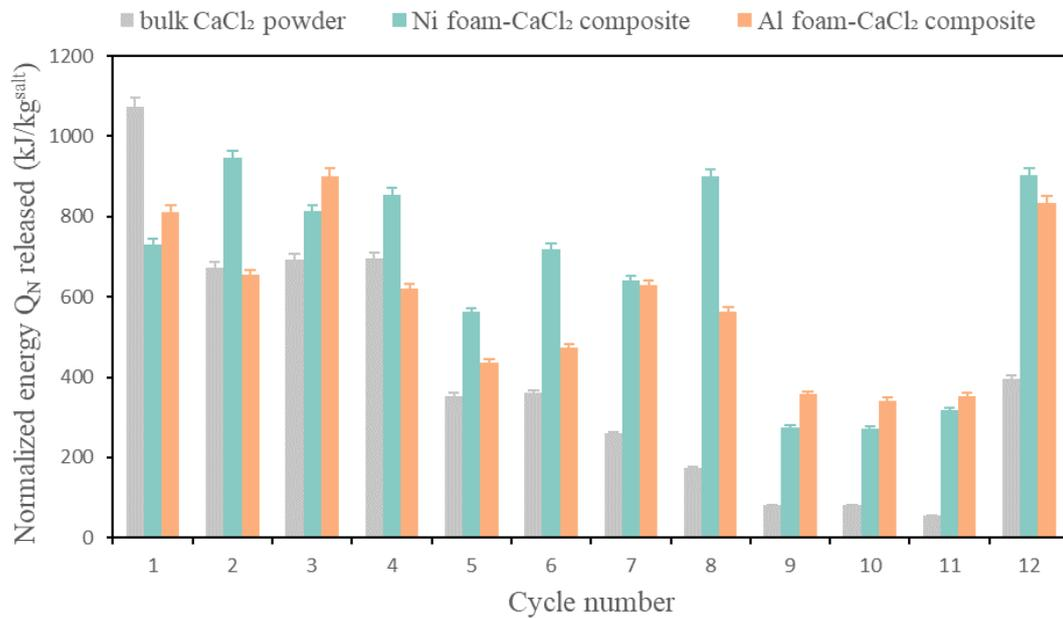
Fig. 3.10. Normalized thermal energy released during 12 cyclic hydration/dehydration processes of nickel foam-CaCl<sub>2</sub> composite, aluminum foam-CaCl<sub>2</sub> composite and bulk CaCl<sub>2</sub> powder.
