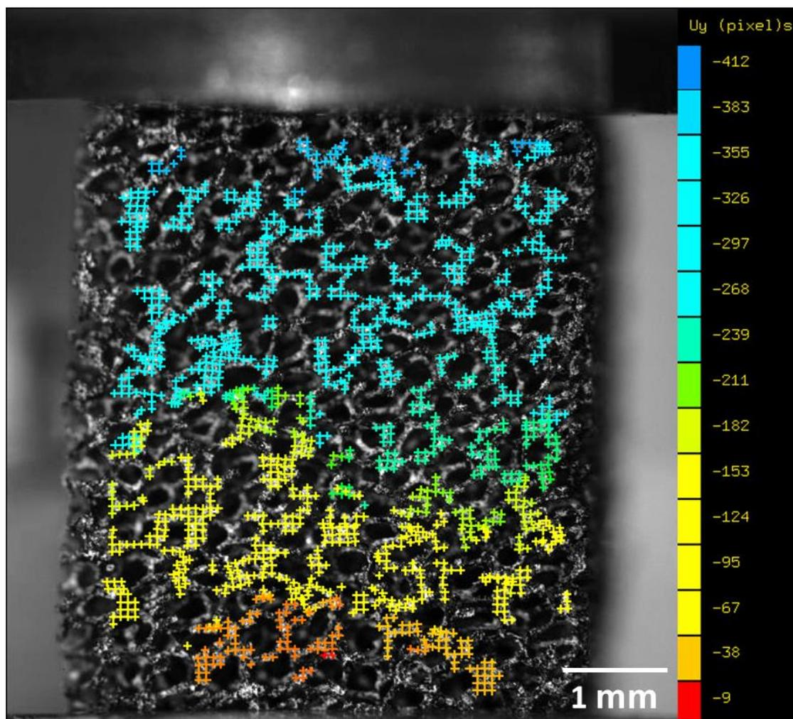
Fig. 2.56 Displacement map on the compression axis (vertical) of each correlation point of sample CuO<sub>2</sub> at macroscopic strain of 15%.
