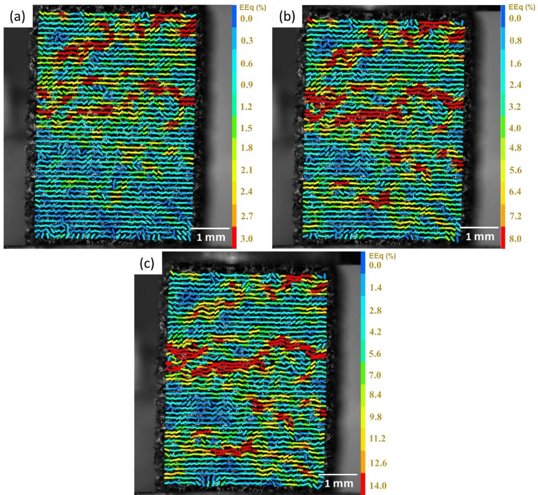
Fig. 2.53 Equivalent strain maps (correlation domain of  $50 \times 50$  pixels) for Cu<sub>2</sub>O during compression (vertical) at macroscopic strain levels of (a) 1% (b) 4% and (c) 7% with different color code scales adapted to each strain map.
