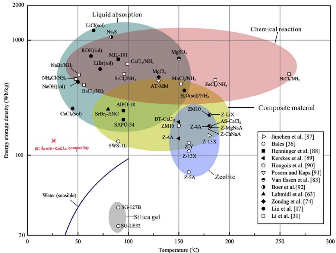
Fig. 3.20 Energy storage density of different TCMs [31] with the energy storage density of nickel foam-CaCl<sub>2</sub> composite studied in our work marked with a red cross. The horizontal axis represents the discharge temperature.
