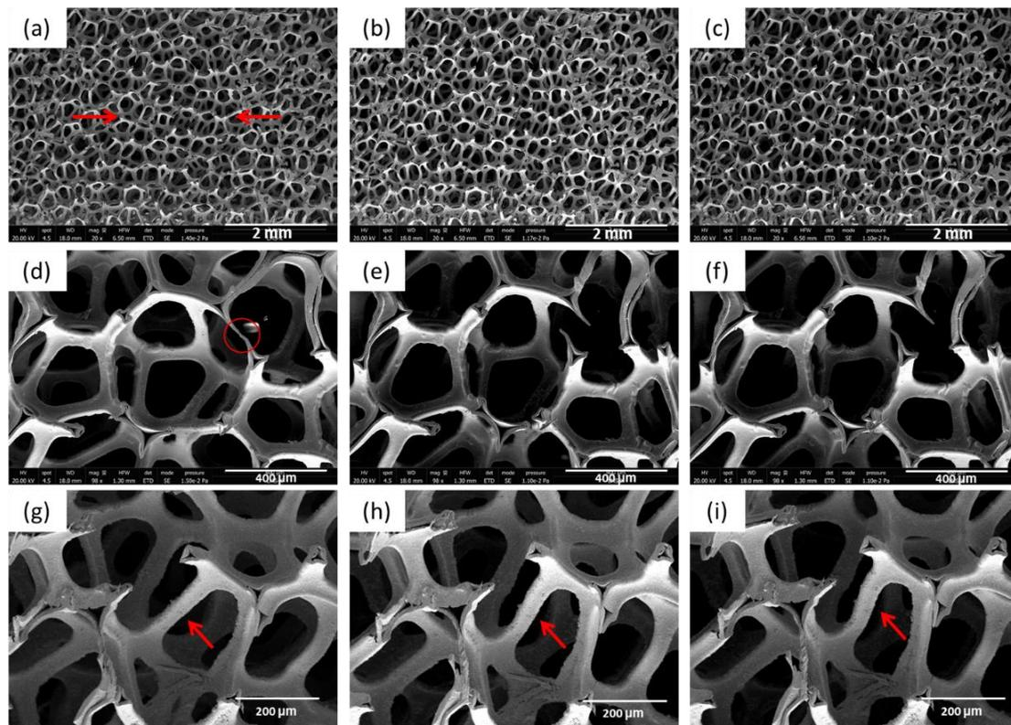
Fig. 2.57 SEM images of copper foam at the axial strain of (a) 0% (b) 4% and (c) 6% during compression test at 150 °C, with (d) to (f) zooming on one pore located in the center, and (g) to (i) zooming on one strut.
