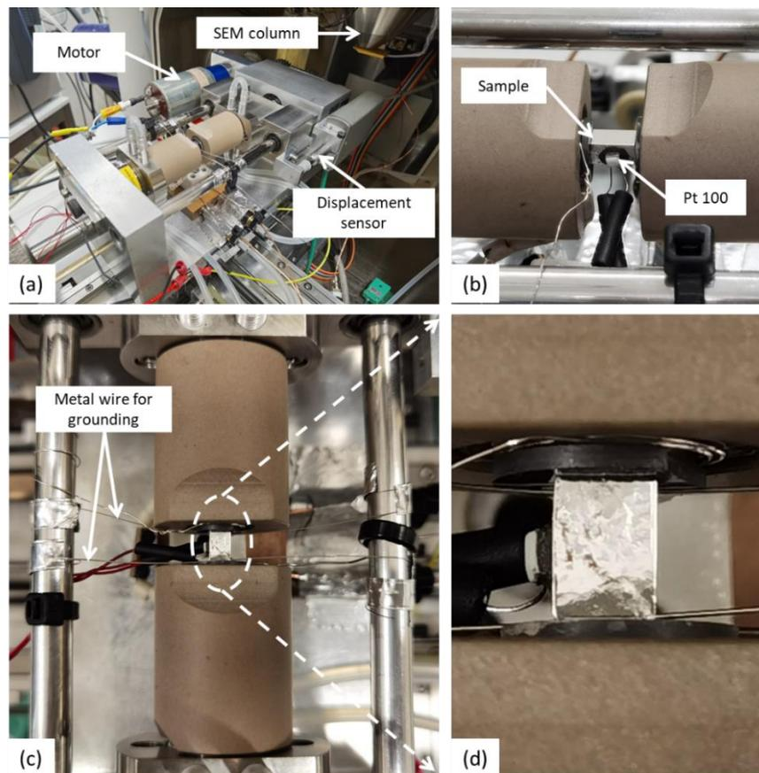
Fig. 2.29 Photos of in situ SEM uniaxial compression test setup for performing on  $\text{AlMn}_{0.1}$  massive sample. (a) The overview of the experimental setup with DC-motor and LVDT. (b) Zoom on the sample (before loading) with a Pt100 temperature sensor glued to the side of the sample. (c) Top view of the setup focusing on the sample and (d) zoom on the sample surface after loading.
