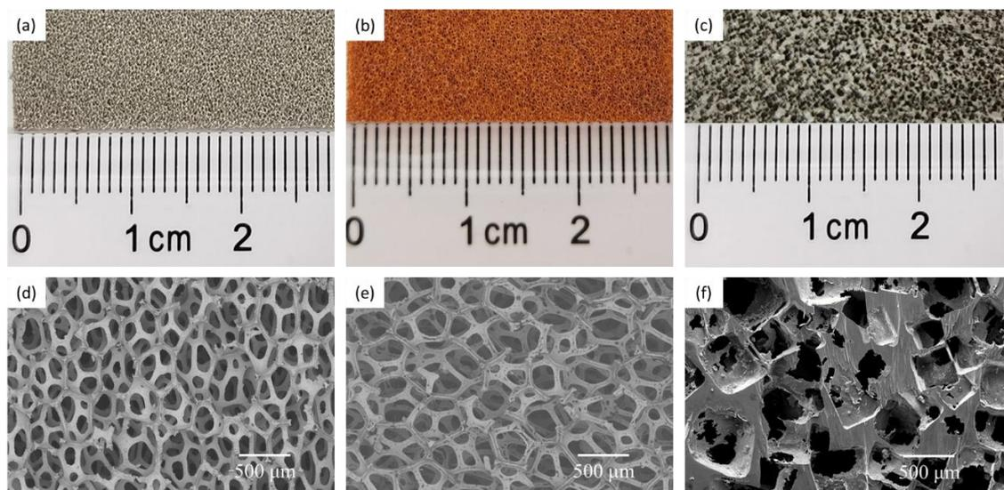
Fig. 2.31 Photo of (a) nickel foam (b) copper foam (c) aluminum foam and Backscattered Electron (BSE) image (x40 magnification) of (d) nickel foam ( $\rho/\rho_s = 0.04$ ) (e) copper foam ( $\rho/\rho_s = 0.04$ ) and (f) aluminum foam ( $\rho/\rho_s = 0.27$ ).
