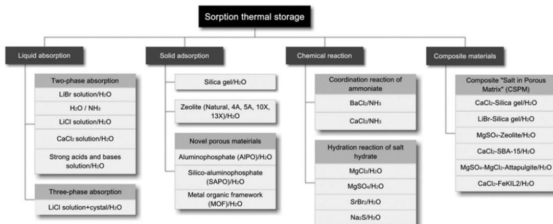
Fig. 1.7 Classification of sorption thermal storage [31].
