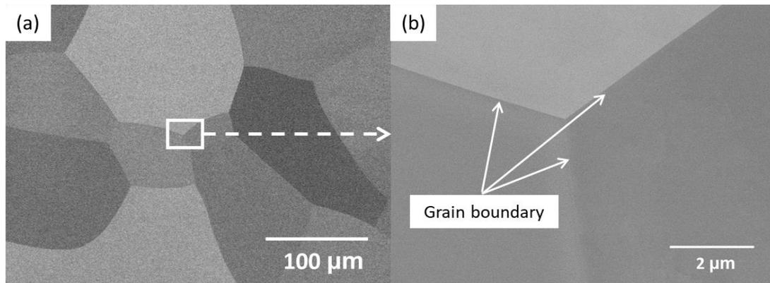
Fig. 2.18 Z-contrast SEM image of (a) (x131 magnification) AlMn<sub>0.1</sub> sample grain morphology with (b) zoom (x12700 magnification) on grain boundaries between 3 grains.
