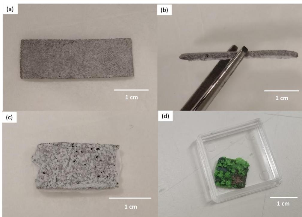
Fig. 3.2 Photo of (a) nickel foam- $\text{CaCl}_2$  composite with (b) its side view, (c) aluminum foam- $\text{CaCl}_2$  composite, and (d) the copper foam- $\text{CaCl}_2$  composite (after corrosion).
