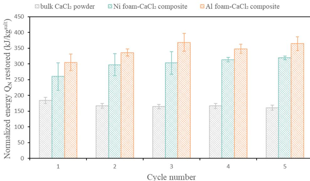
Fig. 3.16. Normalized thermal energy restored during short cyclic hydration/dehydration process of nickel foam- $\text{CaCl}_2$  composite, aluminum foam- $\text{CaCl}_2$  composite and bulk  $\text{CaCl}_2$  powder.
