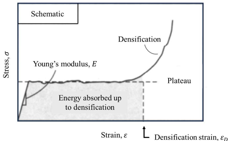
Fig. 2.2 Schematic stress-strain curve of metal foam in compression [130].
