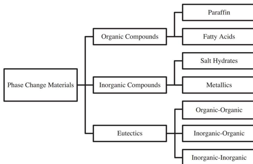
Fig. 1.5 Classification of solid-liquid phase change materials [23].
