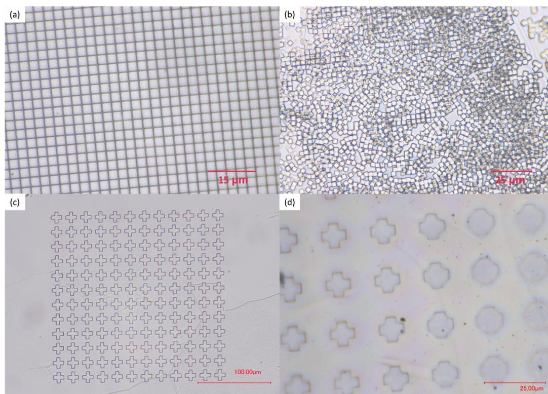
Fig. 2.23 Optical microscope image of successful (a) grids and (c) cross pattern after exposure and developing process, while unsuccessful patterns such as (b) the grids displaced after developing process and (d) the crosses with blurred and rounded boundaries.
