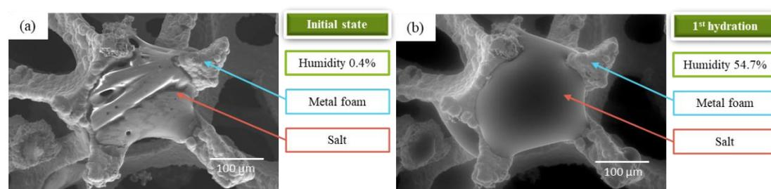
Fig. 3.23. GSED images ( $\times 254$  magnification) of the nickel foam- $\text{CaCl}_2$  composite sample surface focused on the interface of salt and metal foam with (a) the initial state (0.4% RH) and (b) after first hydration (54.7% RH).
