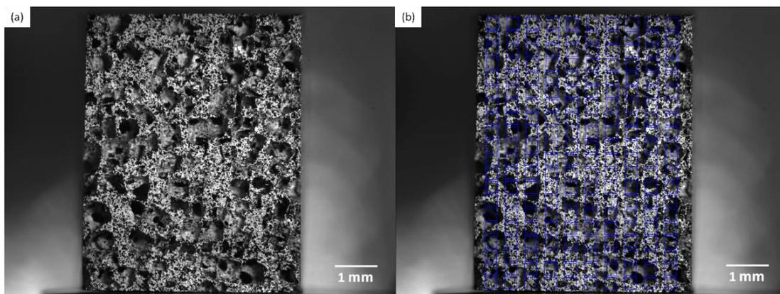
Fig. 2.59 (a) The initial state image of aluminum sample Al01 by optical microscope and (b) the same image serving as the reference image for computing the macroscopic strain maps using CMV with the matrix of points defined and the correlation domains shown in blue squares.
