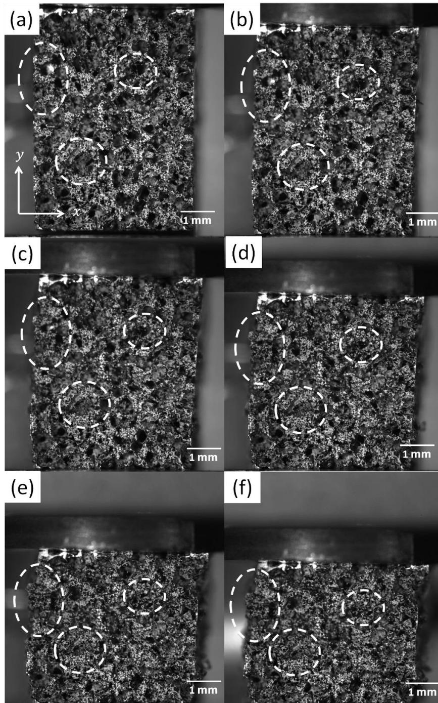
Fig. 2.70 Loaded open-cell aluminum foam sample Al02 at different strains of (a) 0%, (b) 2%, (c) 9%, (d) 16%, (e) 23% and (f) 30%.
