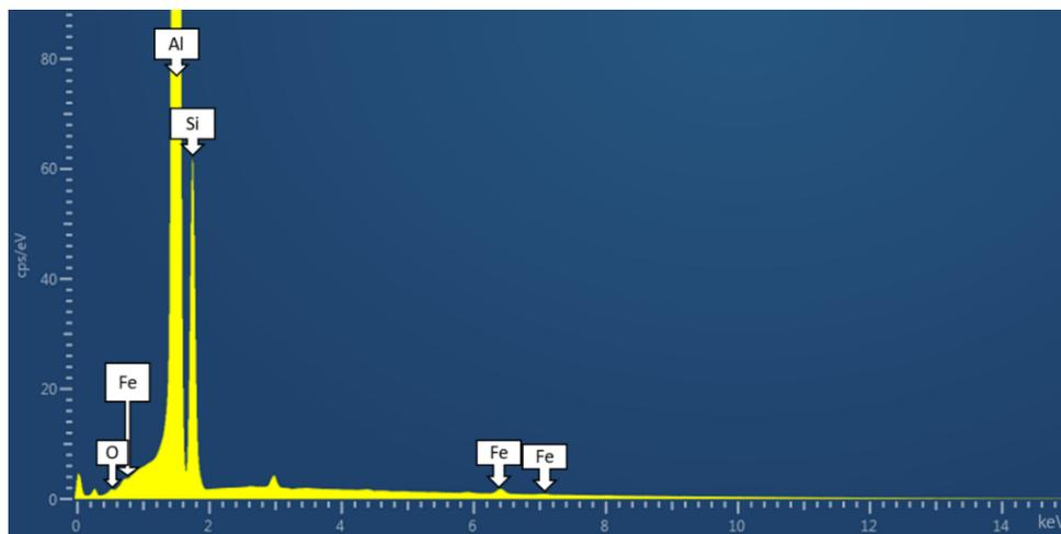
Fig. 2.35 EDX spectrum obtained for aluminum foam.
