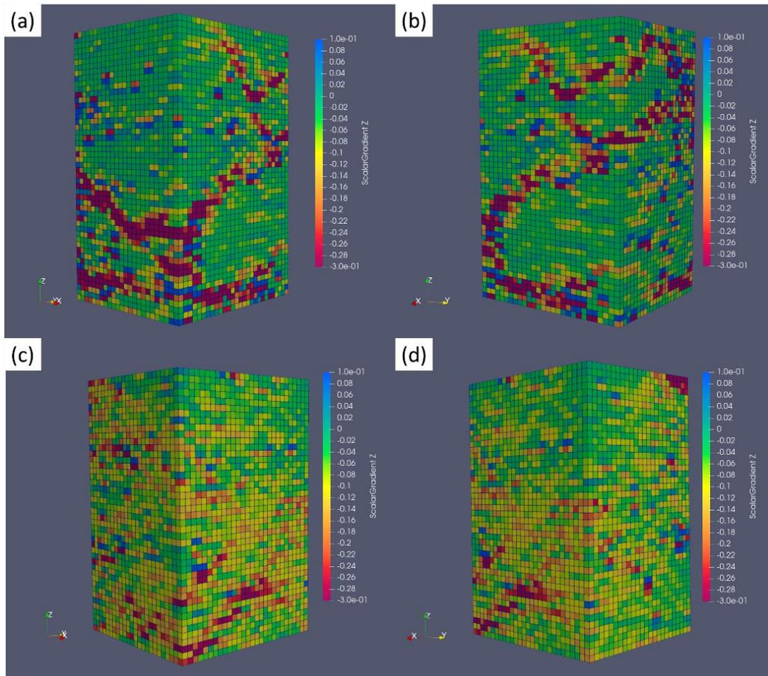
Fig. 2.80 Longitudinal deformation maps (strain gage length of 312  $\mu\text{m}$ ) at final macroscopic strain level of 9% for (a) (b) aluminum foam sample Al-to and (c) (d) copper foam sample Cu-to after uniaxial compression at 150  $^{\circ}\text{C}$ .
