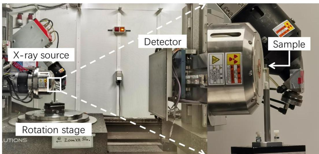
Fig. 2.9 Photo of X-ray microtomography system used for sample 2D projection image acquisition.
