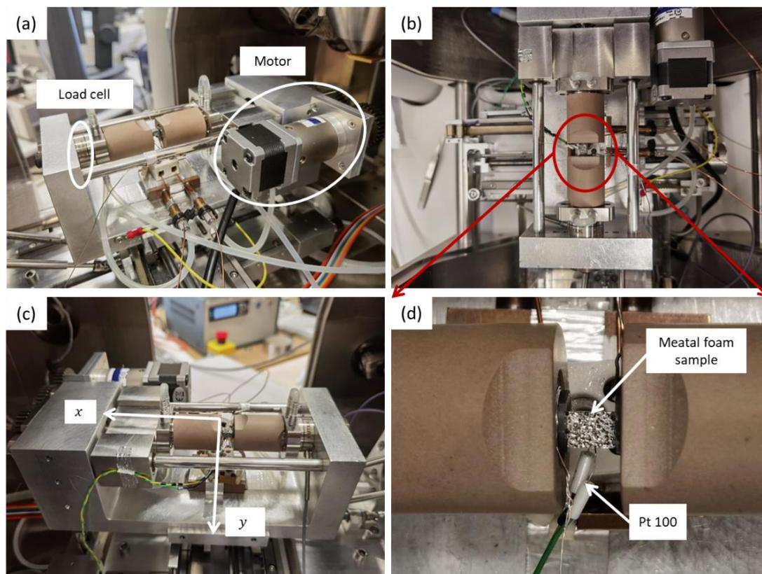
Fig. 2.10 (a) Right view, (b) top view, (c) left view of the custom-built micro compression machine for in situ SEM experiments with (d) zoom on the sample.
