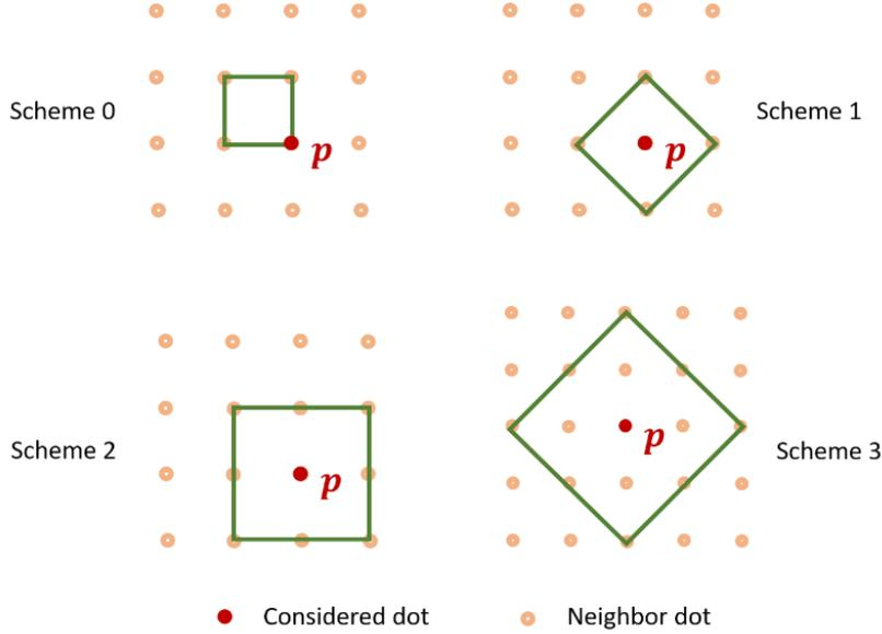
Fig. 2.6 Different schemas of possible integration domain for local gradient calculation.
