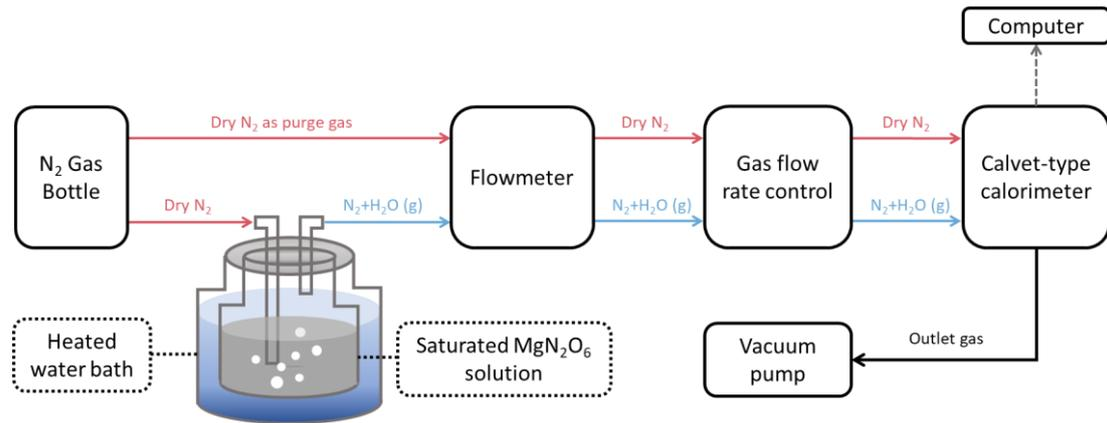
Fig. 3.5. Schematic diagram of the experimental setup.
