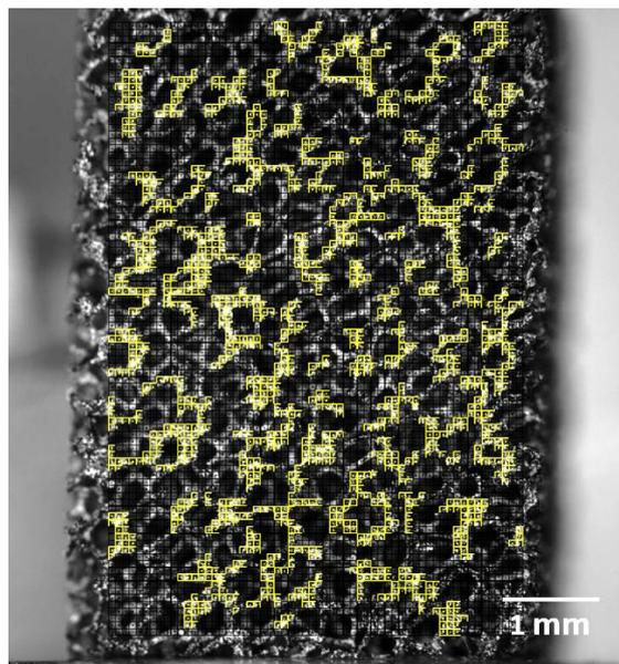
Fig. 2.54 Points and correlation domains defined on reference image for computing microscopic strain maps of copper foam sample Cu<sub>2</sub>O under uniaxial compression at 150 °C.
