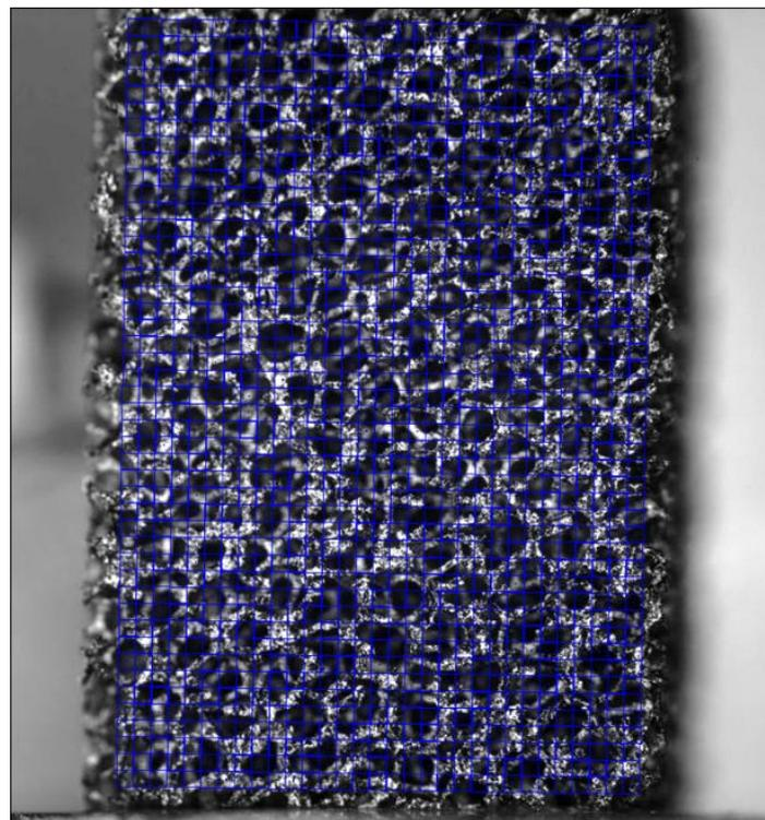
Fig. 2.51 Matrix of the measurement points defined and correlation domains in size of  $50 \times 50$  pixels for computing the strain field at the metal foam structural scale of pores of Cu02.
