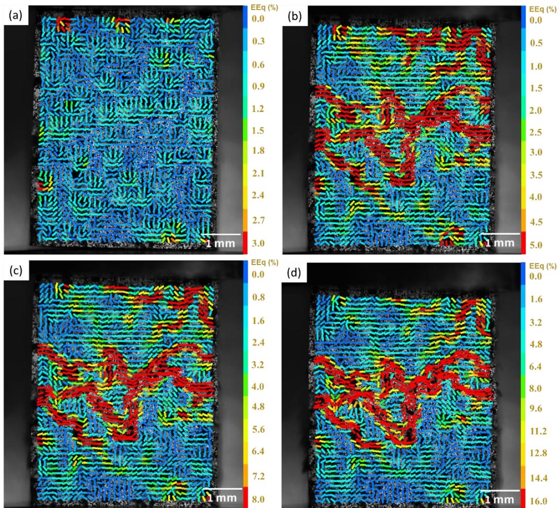
Fig. 2.64 Equivalent strain maps (correlation domain of  $50 \times 50$  pixels) for Al01 during compression (vertical) at macroscopic strain levels of (a) 1% (b) 2.4%, (c) 4% and (d) 8% with different color code scales adapted to each strain map.
