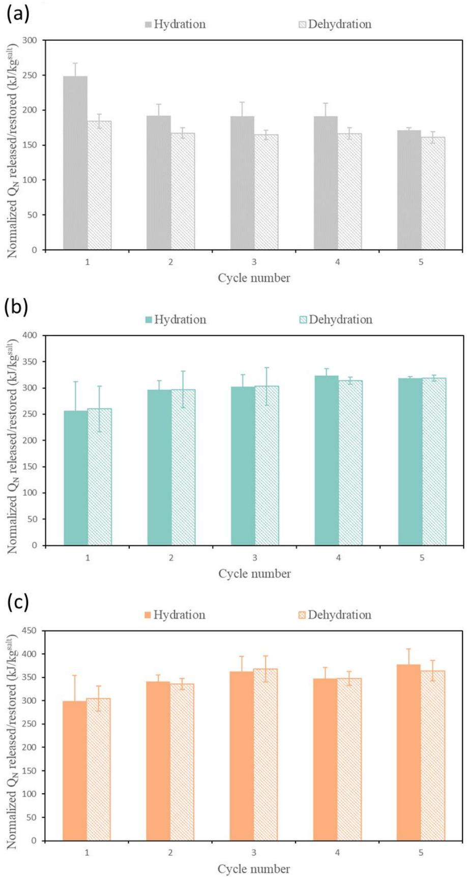
Fig. 3.18 Normalized thermal energy released/stored during short cyclic hydration/dehydration process of (a) bulk  $\text{CaCl}_2$  powder, (b) nickel foam- $\text{CaCl}_2$  composite and (c) aluminum foam- $\text{CaCl}_2$  composite.
