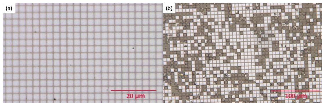
Fig. 2.27 Optical microscope images of (a) successful pattern of grids and (b) unsuccessful pattern of grids formed on the sample surface after Pt deposition and PMMA dissolution processes.
