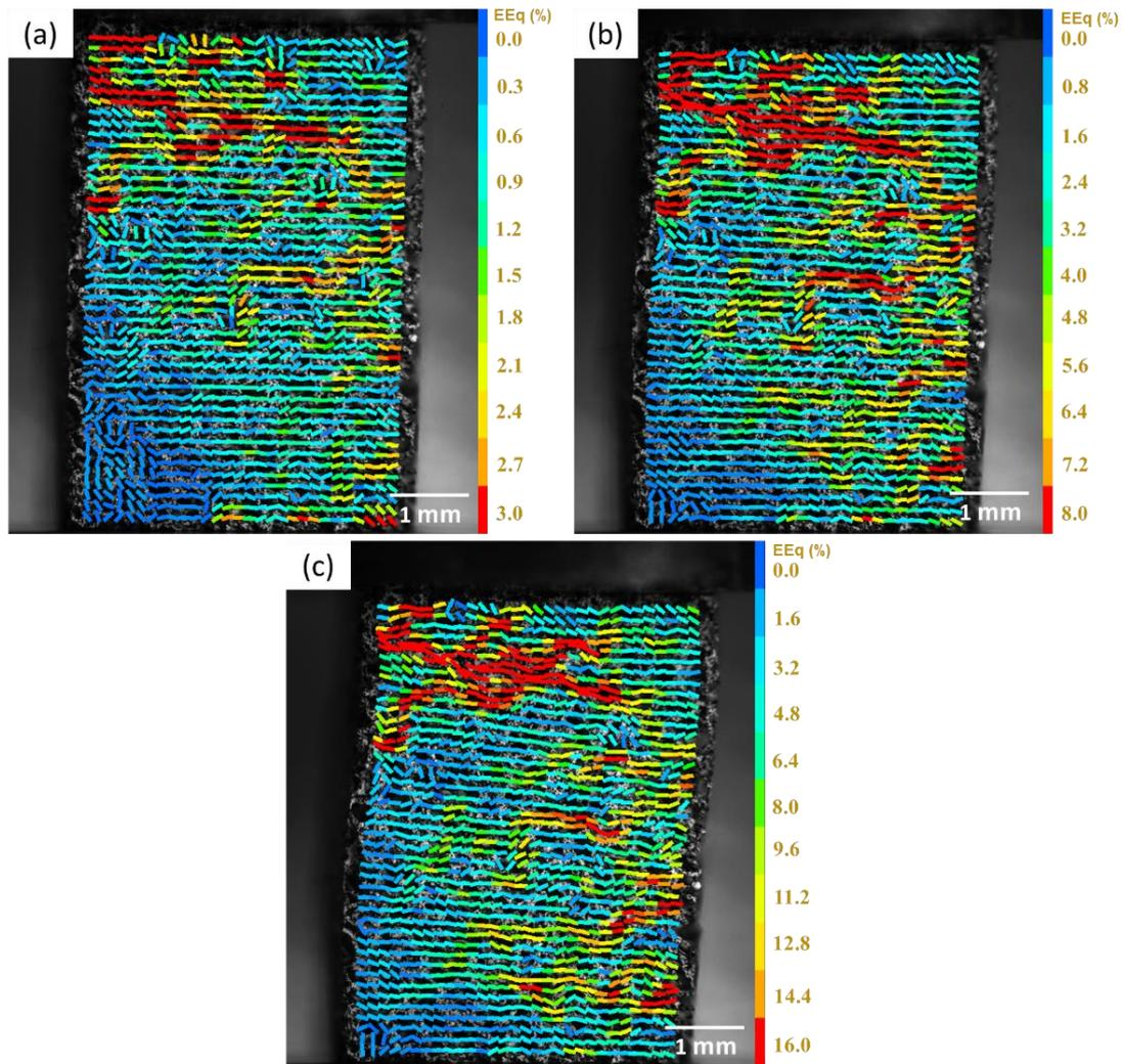
Fig. 2.44 Equivalent strain maps (correlation domain of  $50 \times 50$  pixels) for Cu01 during compression (vertical) at macroscopic strain levels of (a) 1% (b) 4% and (c) 8% with different color code scales adapted to each strain map.
