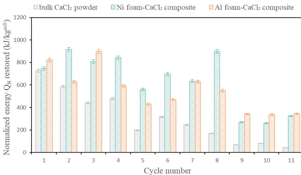
Fig. 3.12. Normalized thermal energy restored during long cyclic hydration/dehydration process of nickel foam- $\text{CaCl}_2$  composite, aluminum foam- $\text{CaCl}_2$  composite and bulk  $\text{CaCl}_2$  powder.
