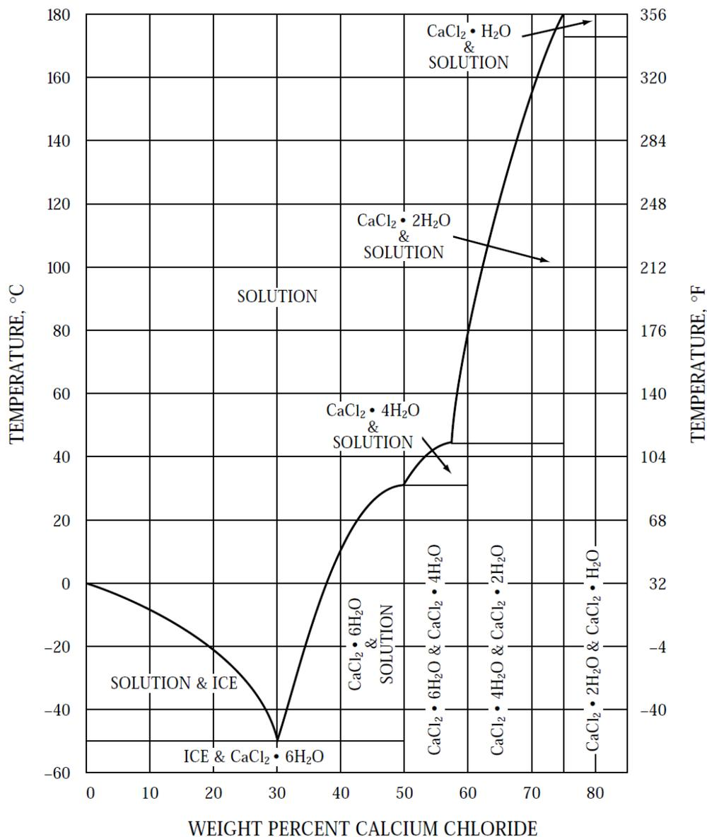
Fig. 1.12 Phase diagram for  $\text{CaCl}_2\text{-H}_2\text{O}$  system under pressure of 1 atm [104].
