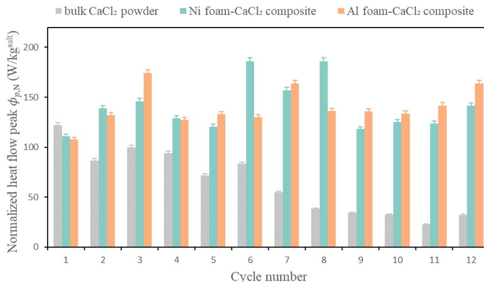
Fig. 3.13. Normalized maximum heat flow peak of hydration process during 12 hydration/dehydration cycles of nickel foam-CaCl<sub>2</sub> composite, aluminum foam-CaCl<sub>2</sub> composite and bulk CaCl<sub>2</sub> powder.
