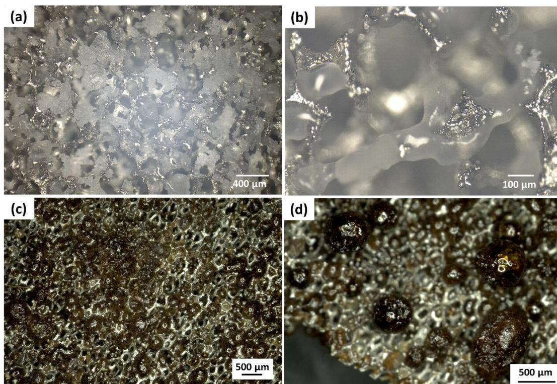
Fig. A.6. Optical microscopy image of (a) nickel foam- $\text{CaCl}_2$  composite with sugar film as binder and (b) zooming on one of the struts of the composite. (c) Nickel foam- $\text{CaCl}_2$  composite with sugar film as binder after heated to  $100\text{ }^\circ\text{C}$  and (d) zooming on the sample after heated to  $100\text{ }^\circ\text{C}$ .
