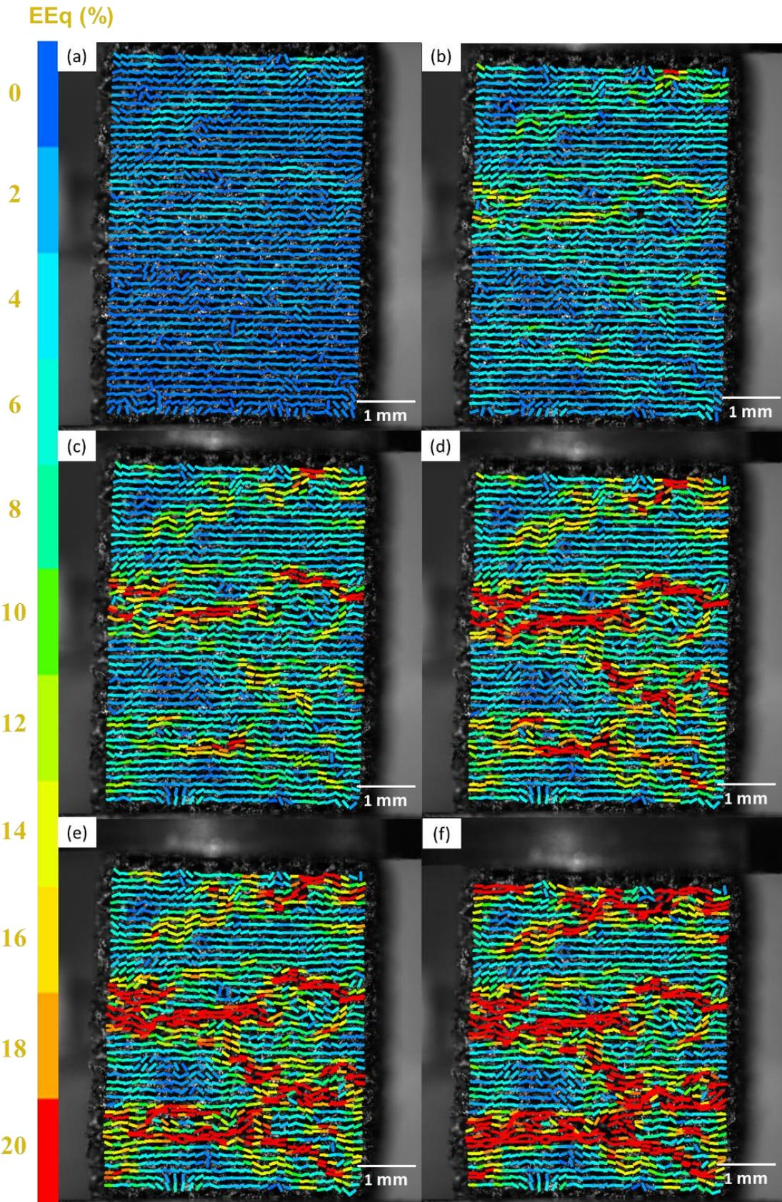
Fig. 2.52 Equivalent strain maps (correlation domain of  $50 \times 50$  pixels) at different levels of the macroscopic strain of sample Cu02 during compression (vertical) with (a) at 1% (b) at 4% (c) at 7% (d) at 10% (e) at 12% and (f) at 15%.
