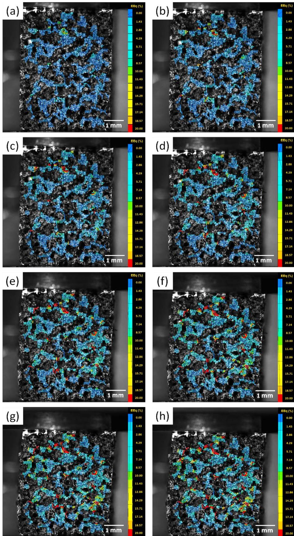
Fig. 2.75 Equivalent deformation maps at eight levels of macroscopic strain of the sample AlO<sub>2</sub> during compression (vertical) at 150 degrees with (a) at 1% (b) at 2.4% (c) at 4% (d) at 7% (e) at 10% (f) at 12% (g) at 14% and (h) at 15%.
