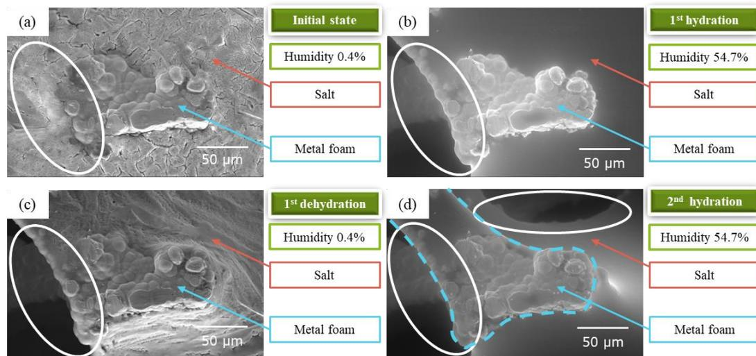
Fig. 3.22. GSED images (x508 magnification) of the nickel foam- $\text{CaCl}_2$  composite sample surface during 2 hydration/dehydration cycles with (a) the initial state (0.4% RH), (b) after the first hydration (54.7% RH), (c) after the first dehydration (0.4% RH) and (d) after second hydration (54.7% RH) under isothermal condition. Redistribution of salt during the hydration/dehydration cycles is marked in circle.
