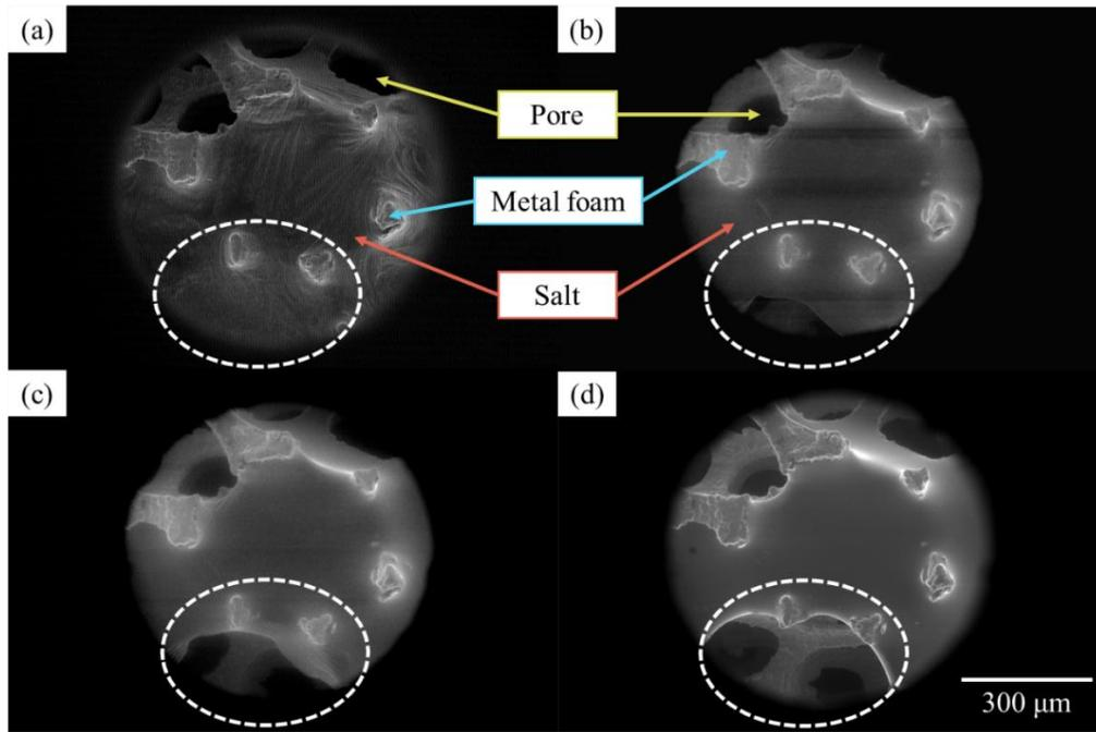
Fig. 3.21. GSED images (x107 magnification) of the nickel foam- $\text{CaCl}_2$  composite sample surface with the relative humidity increasing from (a) 0.4%, (b) 45.3%, (c) 51.4%, to (d) 54.7% under isothermal condition.
