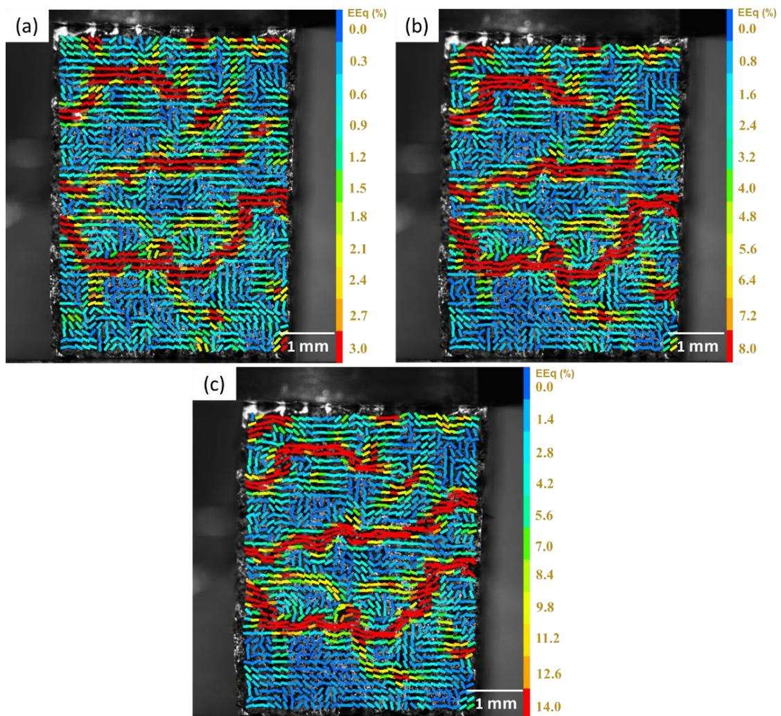
Fig. 2.73 Equivalent strain maps (correlation domain of  $50 \times 50$  pixels) for Al02 during compression (vertical) at macroscopic strain levels of (a) 1% (b) 4% and (c) 8% with different color code scales adapted to each strain map.
