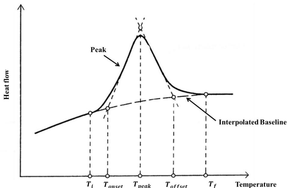
Fig. 3.3 Definition of characteristic terms of DSC curves [203].
