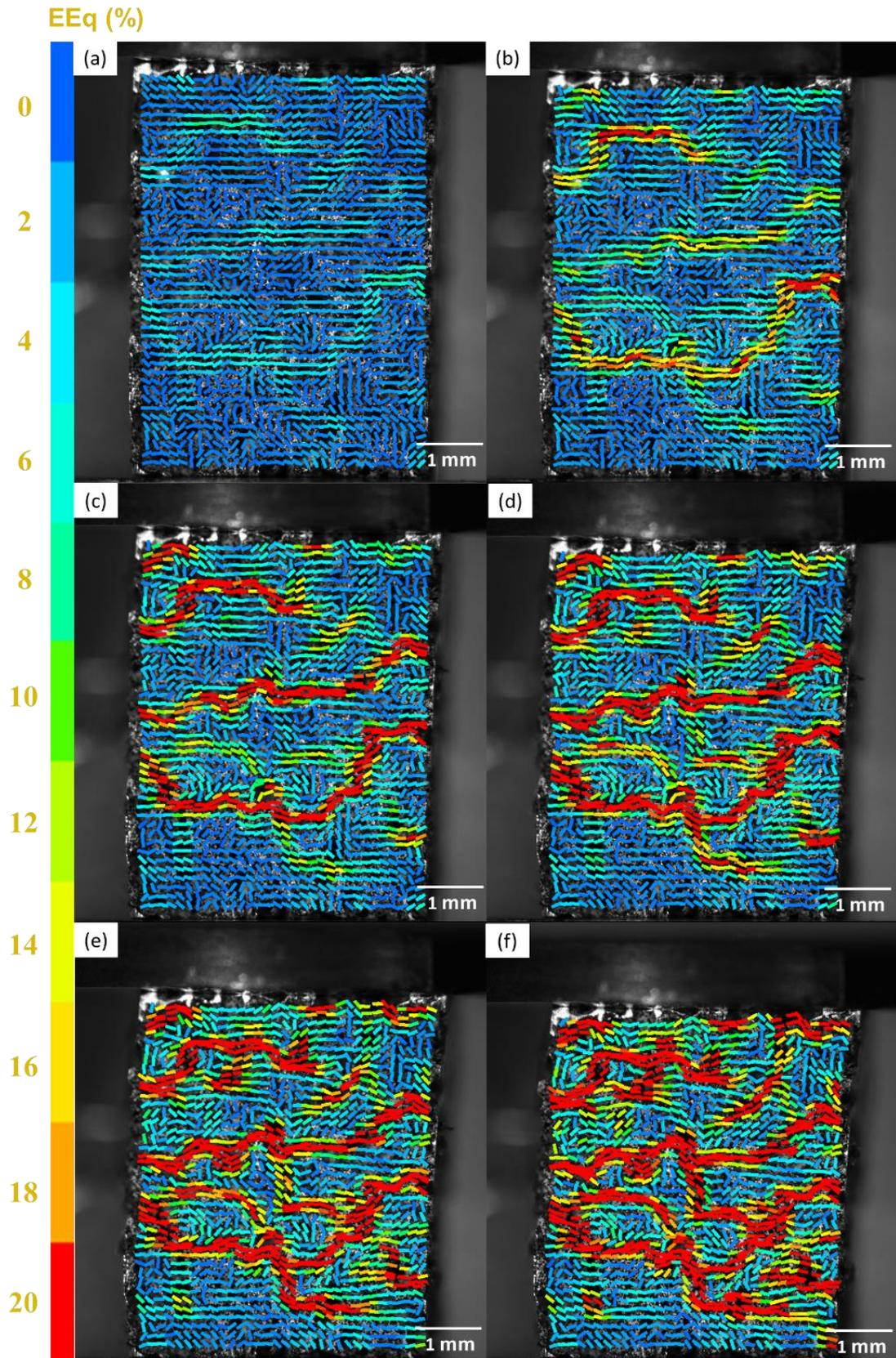
Fig. 2.72 Equivalent strain maps (correlation domain of  $50 \times 50$  pixels) at different levels of the macroscopic strain of sample AlO<sub>2</sub> during compression (vertical) with (a) at 1% (b) at 4% (c) at 7% (d) at 10% (e) at 12% and (f) at 15%.
