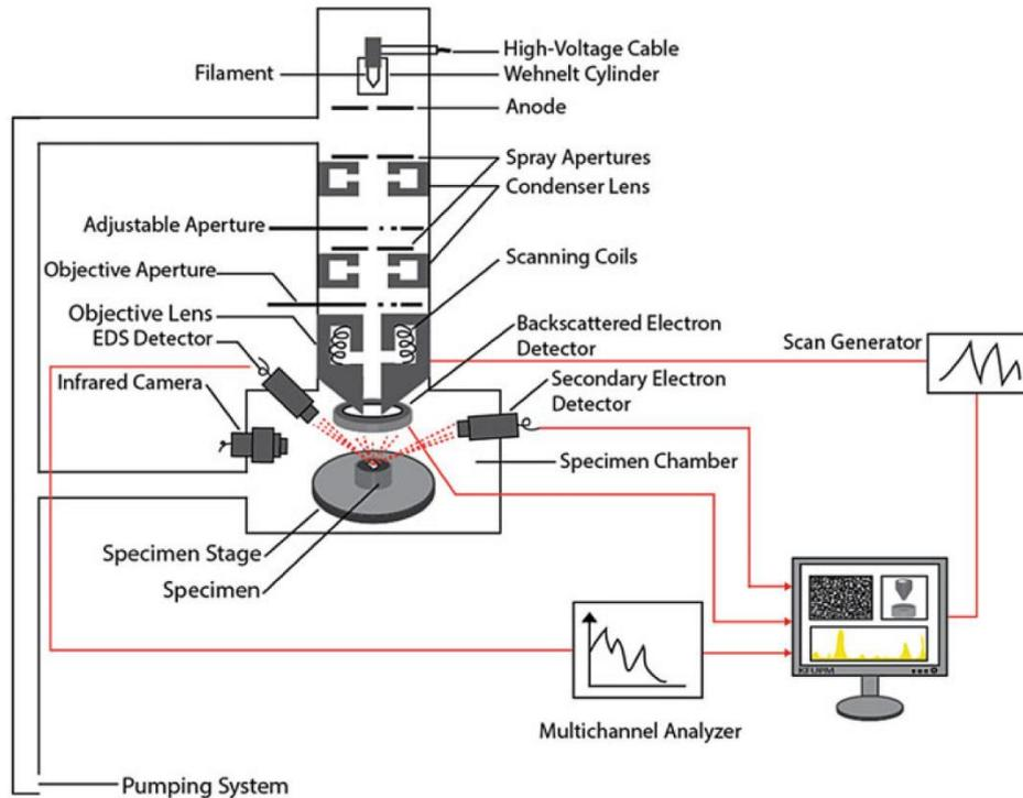
Fig. 2.3 Schematic of the SEM components [164].
