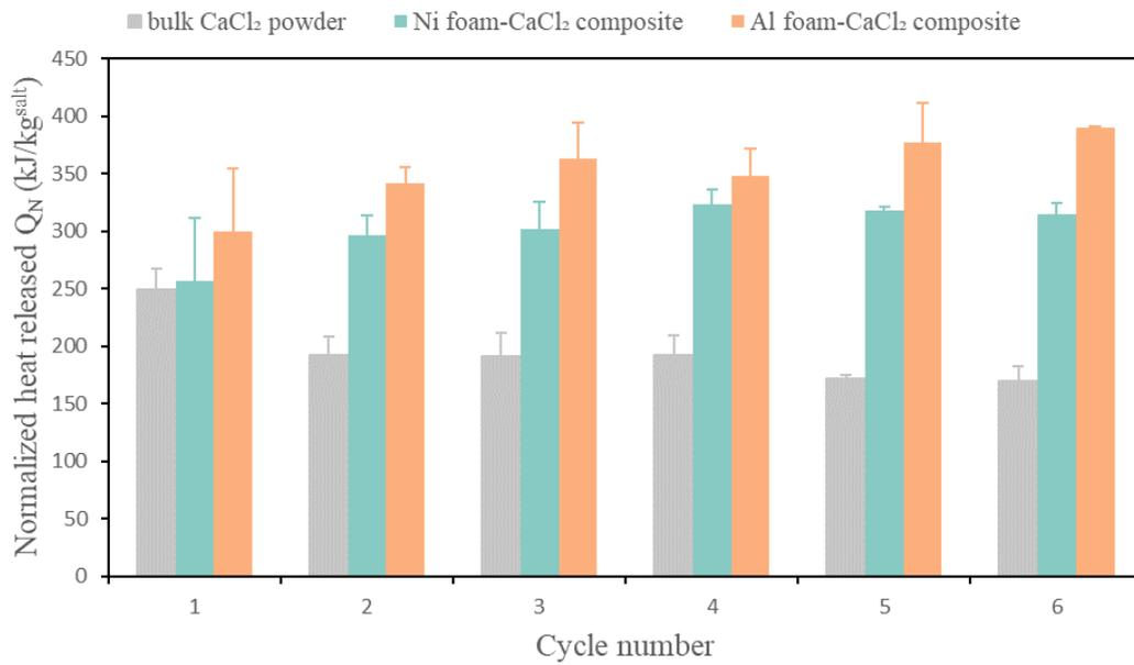
Fig. 3.14. Normalized thermal energy released during 6 hydration/dehydration cycles of nickel foam- $\text{CaCl}_2$  composite, aluminum foam- $\text{CaCl}_2$  composite and bulk  $\text{CaCl}_2$  powder.
