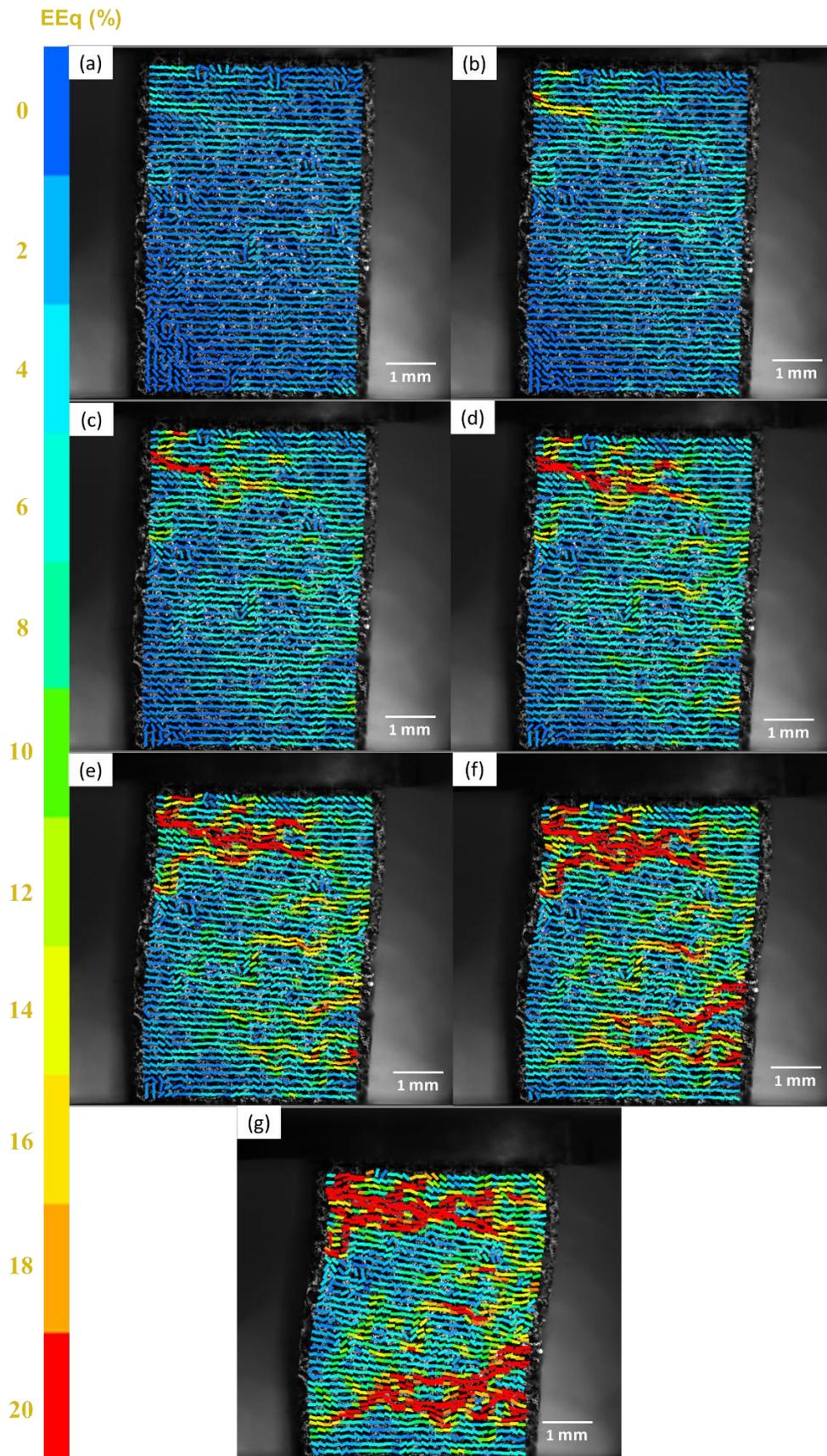
Fig. 2.43 Equivalent strain maps (correlation domain of  $50 \times 50$  pixels) at different levels of macroscopic strain of sample Cu01 during compression (vertical) with (a) at 1% (b) at 2.4% (c) at 4% (d) at 6% (e) at 8%, (f) at 10% and (g) at 14%.
