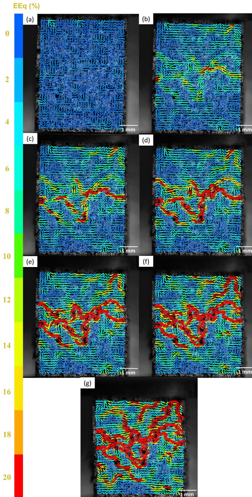
Fig. 2.63 Equivalent strain maps (correlation domain of  $50 \times 50$  pixels) at different levels of the macroscopic strain of sample Al01 during compression (vertical) with (a) at 1% (b) at 2.4% (c) at 4% (d) at 6% (e) at 8%, (f) at 10% and (g) at 14%.
