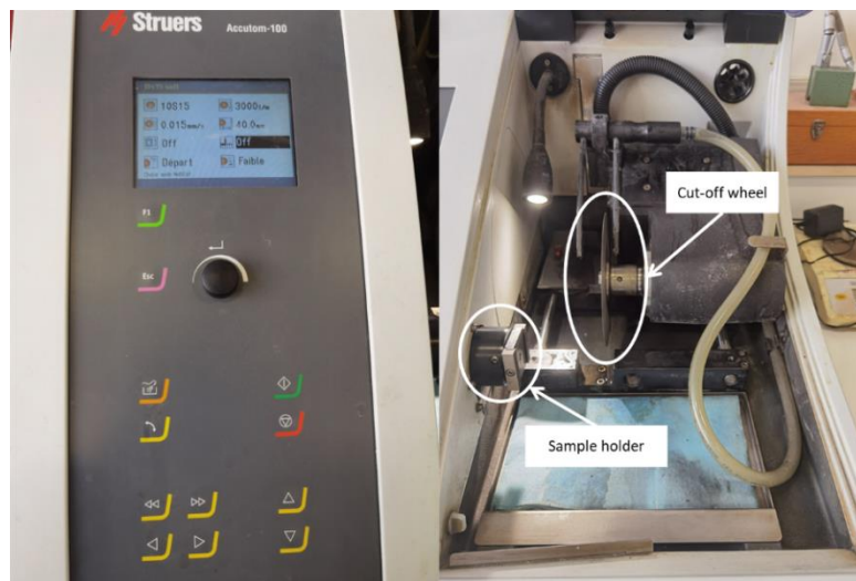
Fig. 2.15 Cut-off machine used for cutting massive aluminum sample in cuboid.
