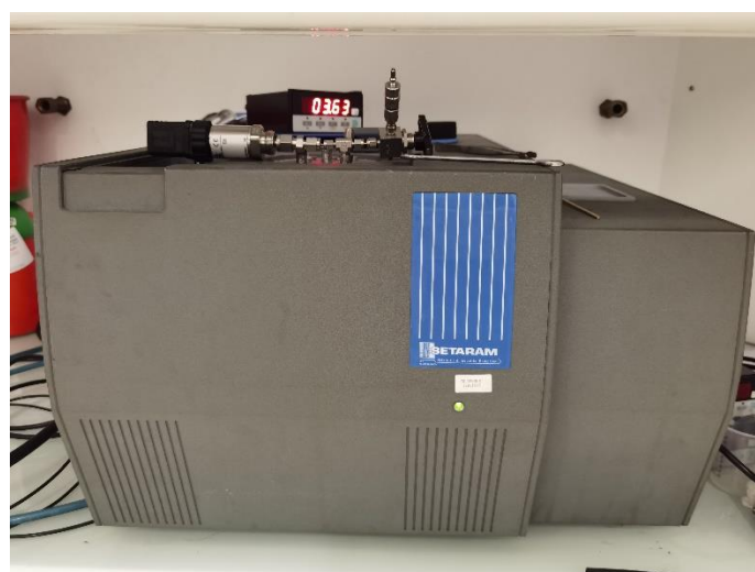
Fig. 3.4 Photo of the Micro-DSC VII device used for thermal properties analysis of composite.
