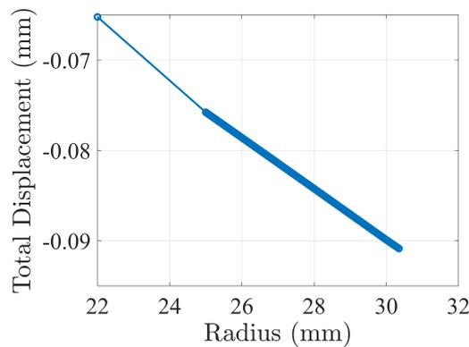
Figure 4.27 – MI CuBe<sub>2</sub>/SS304 total analytic displacement (290 K - 80 K)
