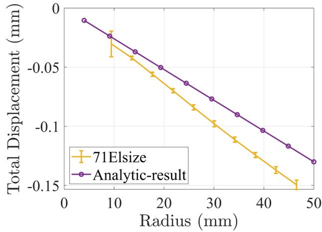
(b) Total displacement magnitude of SS304 disc with setup contraction of  $\alpha_T = -12.9 \times 10^{-4}$  mm/mm, with plexiglass covered heat shields
