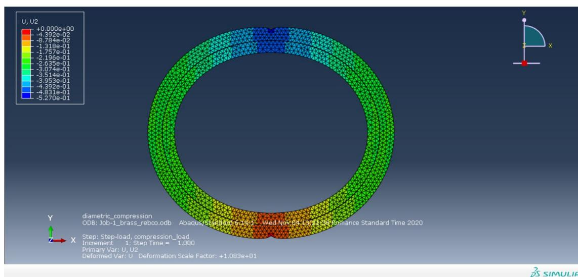
Figure 3.34 – Abaqus model of Brass+REBCO sample in diametric compression (vertical displacement, meters)
