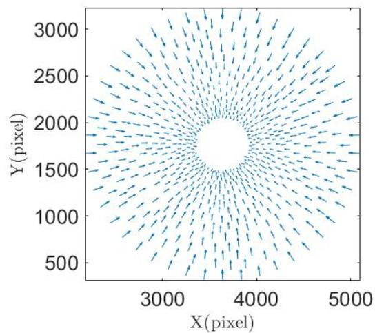
(c) Displacement vectors of mesh Elsize 71 pixels
