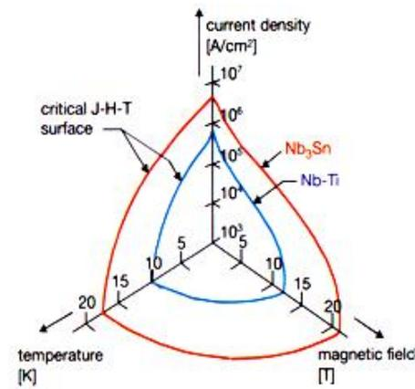
Figure 1.3 – Critical surface of common superconductors [7]
