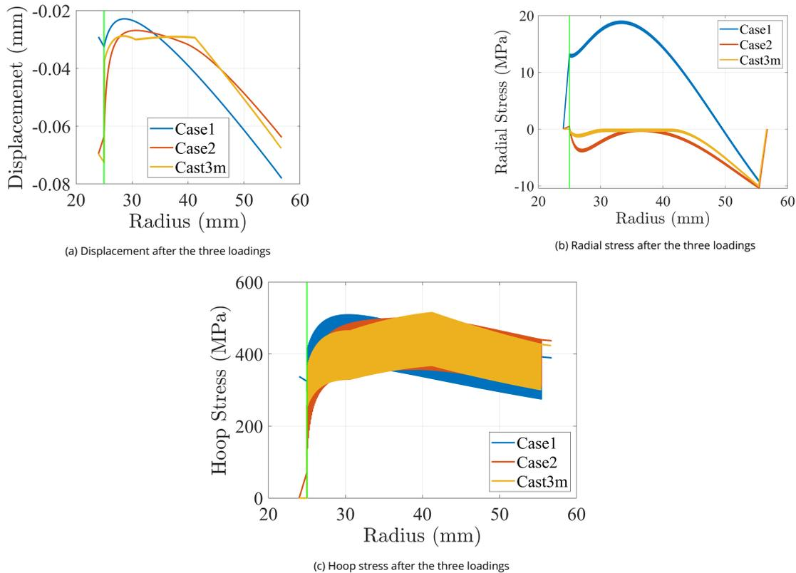
Figure 2.22 – Plane stress formulation calculation while considering de-bonding effect as a decrease of radial young modulus to negligible value in Nougat 30 T calculation (Case1: reference material properties, Case2: radial modulus becomes negligible as a de-bonding effect)
