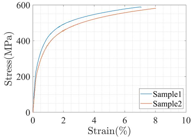
Figure 3.14 – Brass stress-strain curve (at 293 K)
