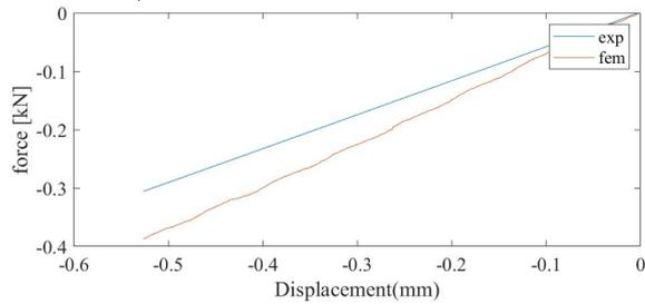
(b) FEMU-F / Experimental forces at the 20<sup>th</sup> iteration of the FEMU-F calculation
