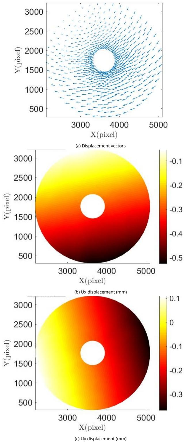
Figure 4.16 – Displacement measured by DIC without rigid body motion elimination of SS304 disc
