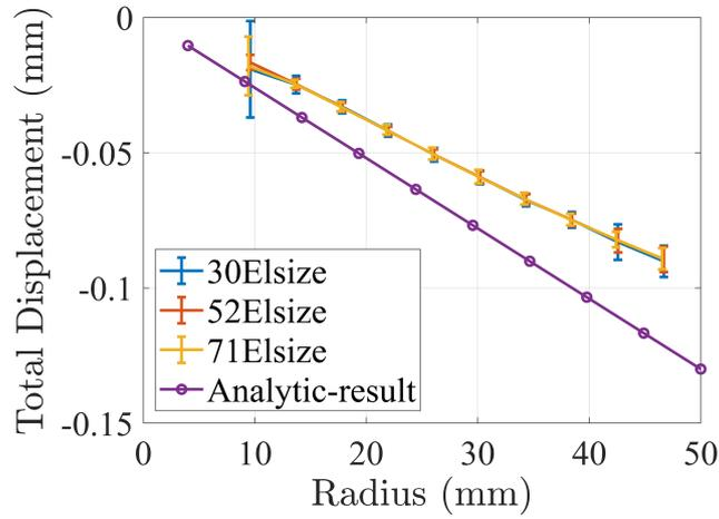
(a) Total displacement magnitude of SS304 disc without setup contraction with plexiglass covered heat shields
