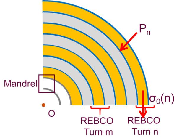
Figure 2.2 – Multi-turn magnet (orange: REBCO, grey: stainless steel)
