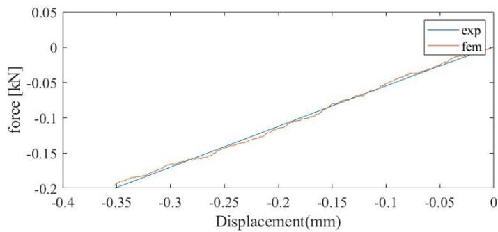
(c) FEMU-UF / Experimental forces at the 20<sup>th</sup> iteration of the FEMU-UF calculation
