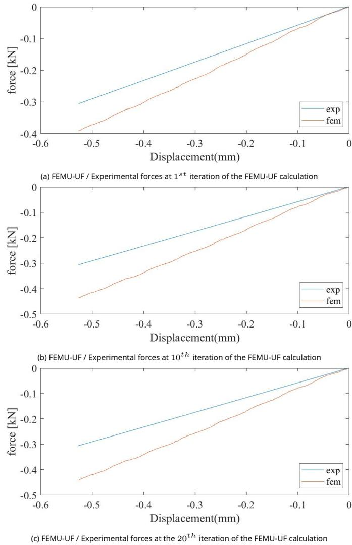
Figure 3.29 – Evolution of FEMU-UF force with calculation iteration
