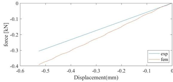
(a) FEMU-F / Experimental forces at the 1<sup>st</sup> iteration of the FEMU-F calculation
