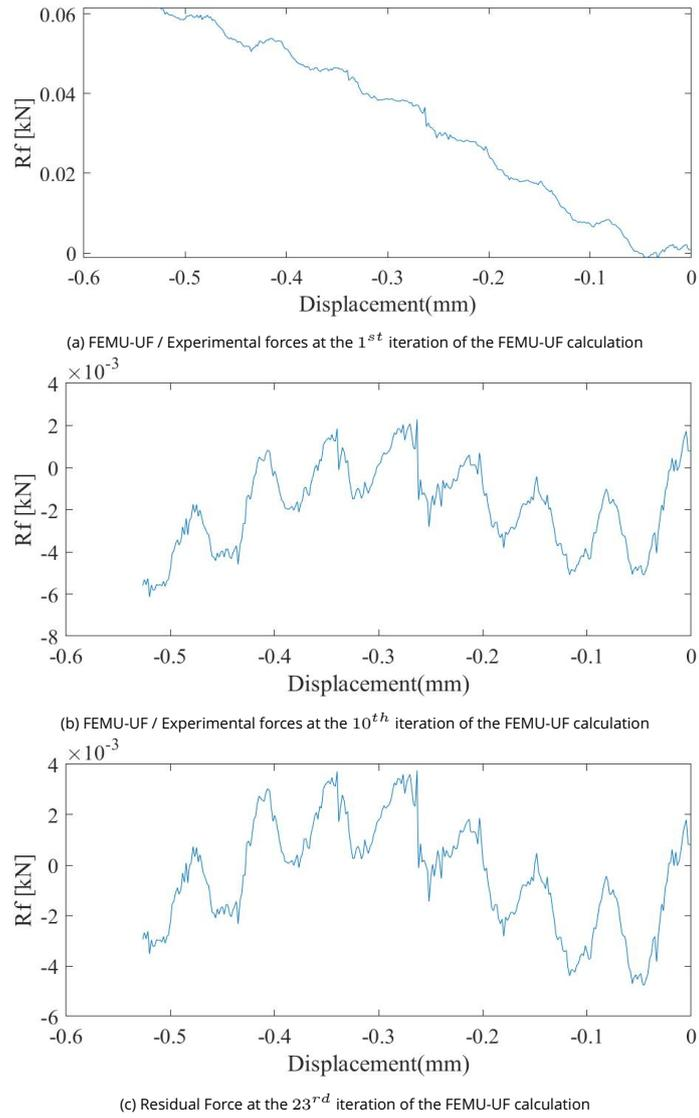
Figure 3.32 – Evolution of the residual force at different iterations - diametric compression of mandrel + REBCO - considering free brass elastic constants
