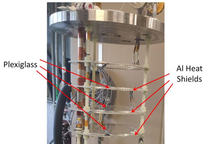
Figure 4.22 – Aluminium heat shields covered with plexiglass
