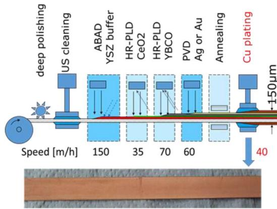
Figure 1.7 – PLD manufacturing process, Burker Manufacturer [32]
