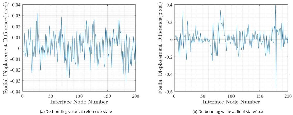
Figure 3.28 - De-bonding values at the contact nodes (Nodes 1-200 are clockwise positioned from mid top of circle position, node positions (Appendix D))
