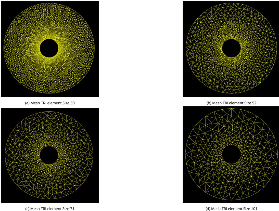
Figure 4.13 – Mesh TRI of different sizes of SS304 disc
