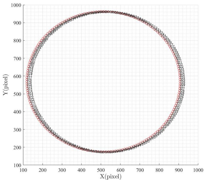
Figure D.2 – Nodes of the REBCO part at the interface between Brass/REBCO (200 Nodes, numbered(101 - 200) - (301 - 400), clockwise numbered from mid-top of circle, numbered as (101 , 301 ...))
