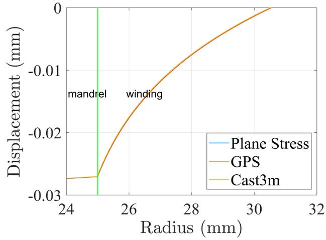
Figure 2.4 - Pre-tension radial displacement
