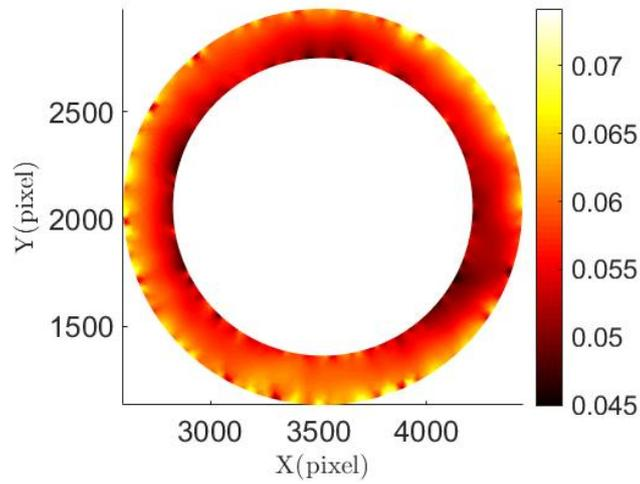
(b) Total displacement magnitude (mm) of mesh Elsize 22 pixels
