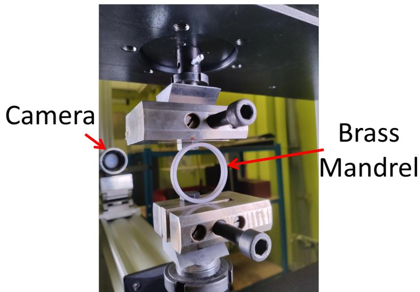
Figure 3.18 – Diametric compression of the brass mandrel
