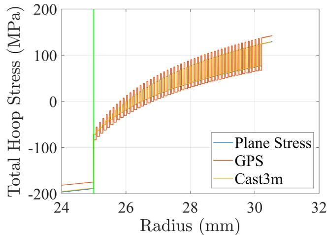
Figure 2.16 - Hoop stress after winding, cooling, and energizing
