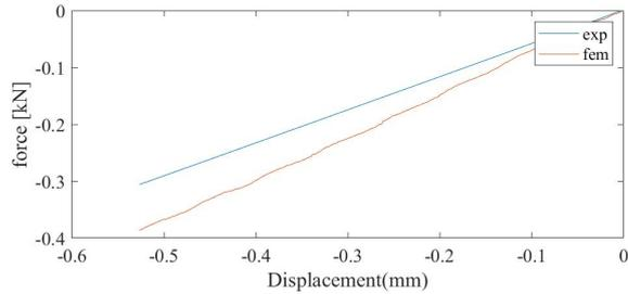
(c) FEMU-F / Experimental forces at the 38<sup>th</sup> iteration of the FEMU-F calculation
