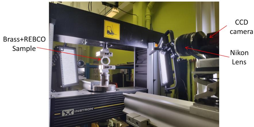
Figure 3.25 – Diametric compression setup of Brass+REBCO
