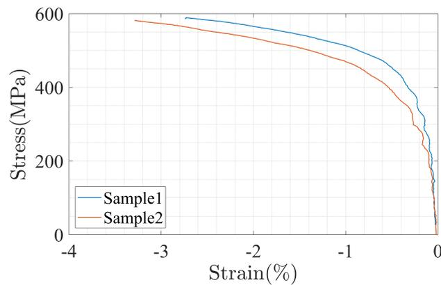
Figure 3.15 – Brass stress-strain curve (at 293 K)
