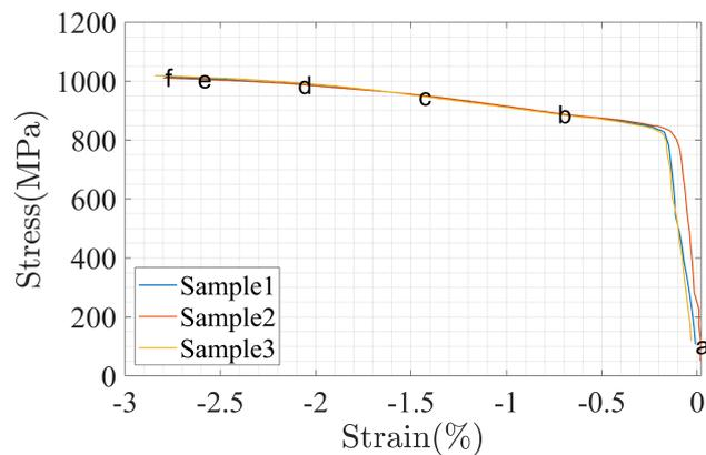
Figure 3.11 – REBCO stress-transverse strain curve (at 293 K)
