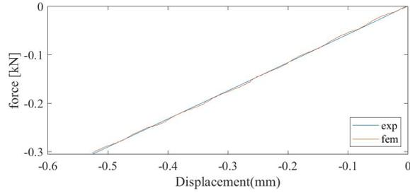
(b) FEMU-F / Experimental forces at the 10<sup>th</sup> iteration of the FEMU-F calculation
