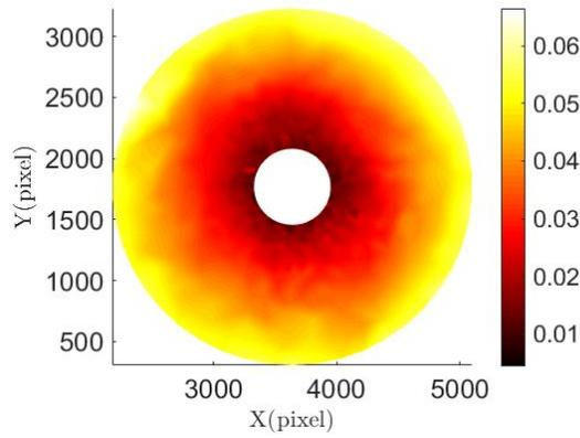
(c) Total displacement magnitude (mm) of mesh Elsize 71 pixels
