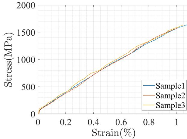
Figure 3.12 - Stainless Steel (SS) stress-strain curve (at 293 K)
