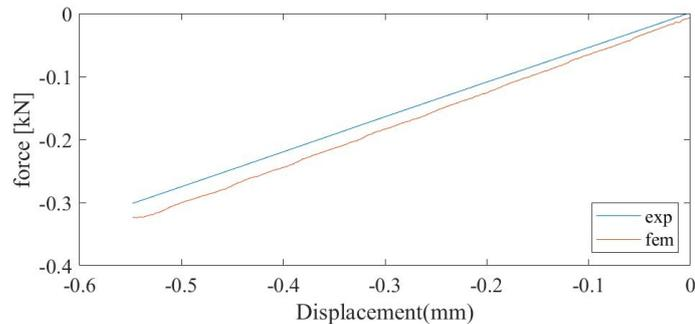
(a) FEMU-UF / Experimental forces at the 1<sup>st</sup> iteration of the FEMU-UF calculation
