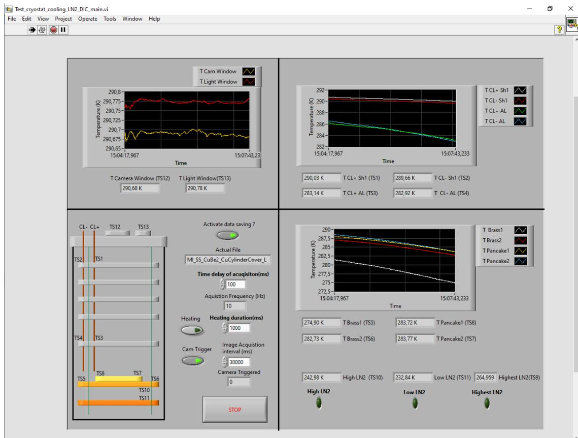
Figure 4.9 – Liquid Nitrogen Cooling LABView program
