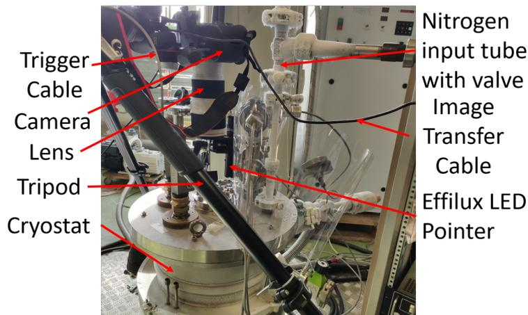
Figure 4.7 - DIC-setup mounted
