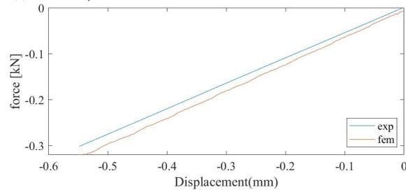
(c) FEMU-F / Experimental forces at the 6<sup>th</sup> iteration of the FEMU-F calculation
