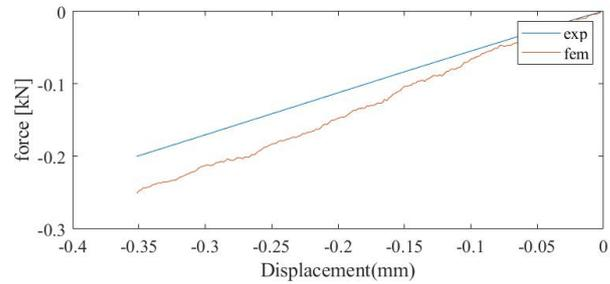
(a) FEMU-UF / Experimental forces at the 3<sup>rd</sup> iteration of the FEMU-UF calculation
