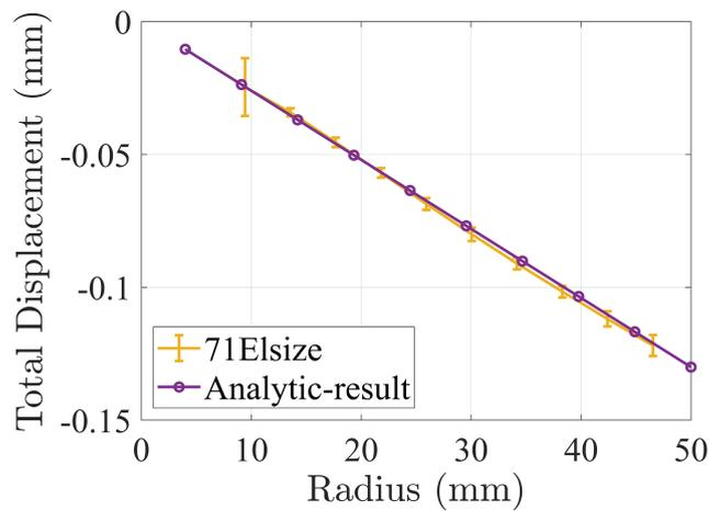
(c) Total displacement magnitude of SS304 disc with setup contraction of  $\alpha_T = -7 \times 10^{-4}$  mm/mm, with plexiglass covered heat shields
