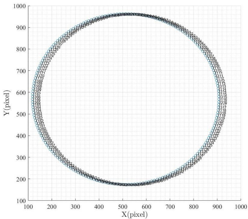
Figure D.1 – Nodes of the Brass mandrel at the interface between Brass/REBCO (200 Nodes, numbered(1091 - 1190) - (1291 - 1390), clockwise numbered from mid-top of circle, numbered as (1091 ,1291 ...))
