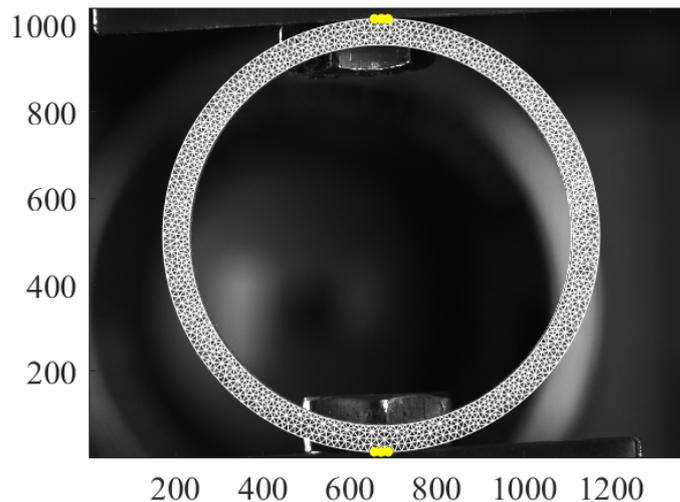
Figure 3.20 – FEMU-UF mesh, contact points (Yellow)
