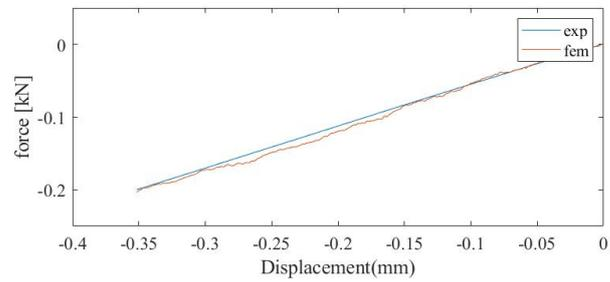
(b) FEMU-UF / Experimental forces at the 5<sup>th</sup> iteration of the FEMU-UF calculation
