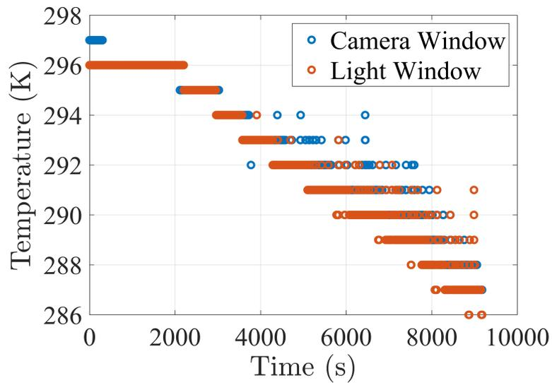
Figure H.1 - Window temperature during cooling test
