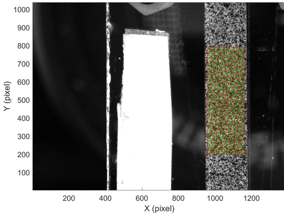
Figure 3.7 - Mesh of ROI with 30 pixel mesh size
