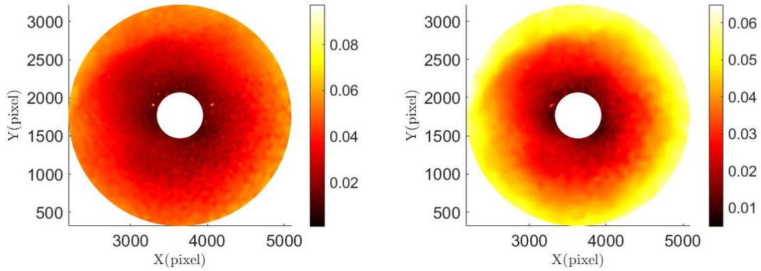
(a) Total displacement magnitude (mm) of mesh Elsize 30 pixels
