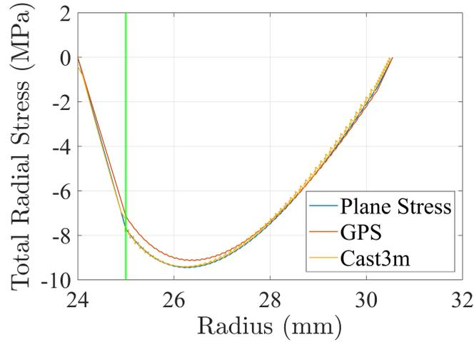
Figure 2.15 - Radial stress after winding, cooling, and energizing
