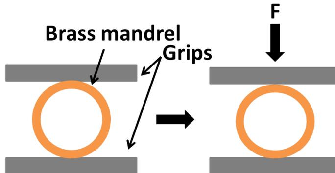
Figure 3.16 – Brass diametric compression test scheme
