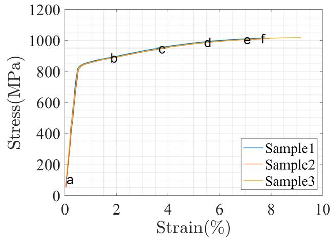
Figure 3.10 – REBCO stress-strain curve (at 293 K)
