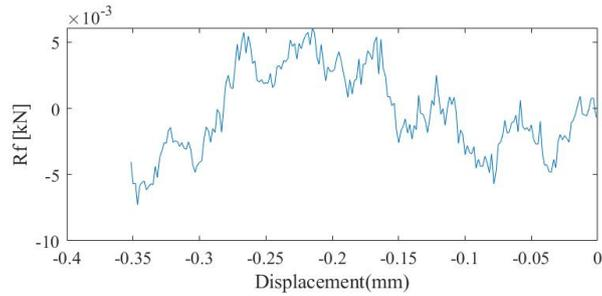
(c) Residual force at the 20<sup>th</sup> iteration of the FEMU-UF calculation
