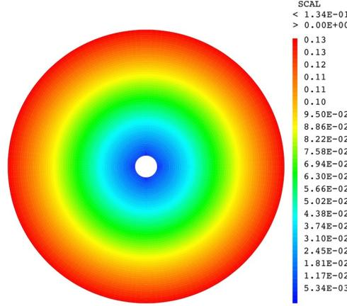
Figure 4.15 – Total thermal contraction (mm) in absolute value of SS304 disc from 300 K to 80 K by Cast3m FEM code
