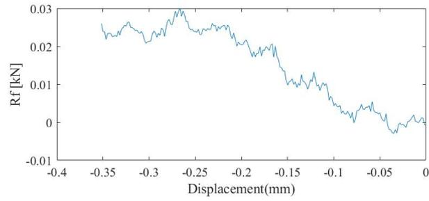
(a) Residual force at the 3<sup>rd</sup> iteration of the FEMU-UF calculation
