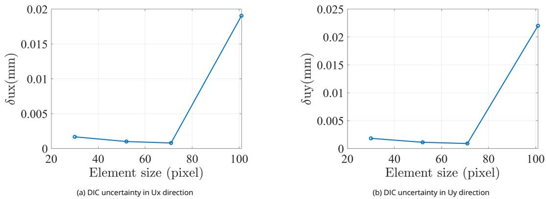
Figure 4.14 – DIC uncertainty of SS304 disc test
