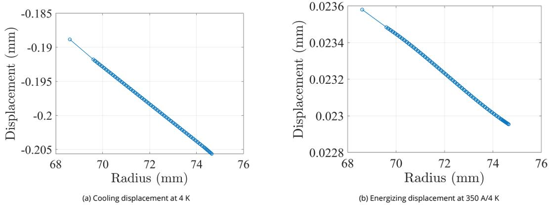
Figure 4.6 - MI REBCO inner pancake displacement
