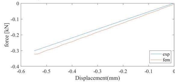
(b) FEMU-F / Experimental forces at the 3<sup>rd</sup> iteration of the FEMU-F calculation
