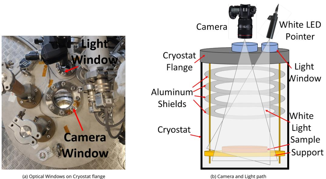
Figure 4.2 – Optical windows configuration for pancake viewing
