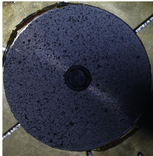
(b) Light dimmed significantly because of water vapor on light window
