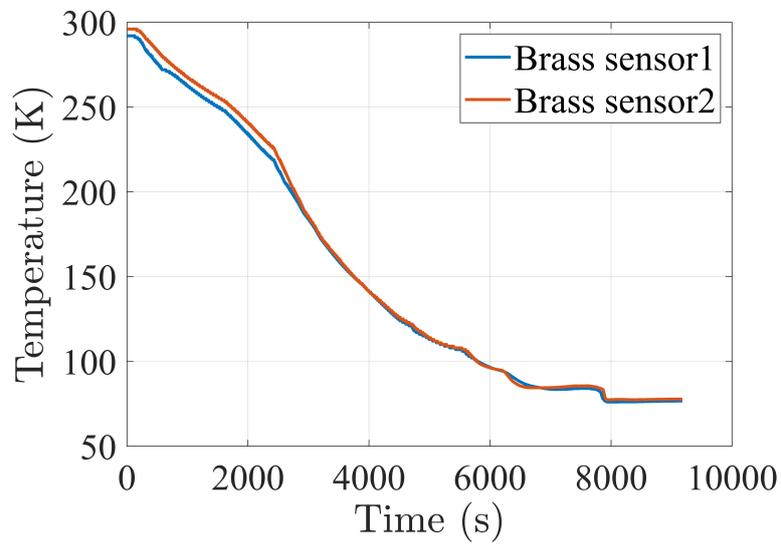
Figure H.4 - Temperature of the brass support
