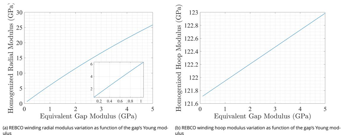
Figure 3.44 – The gap’s effect on the homogenized properties of the winding in Brass+REBCO sample
