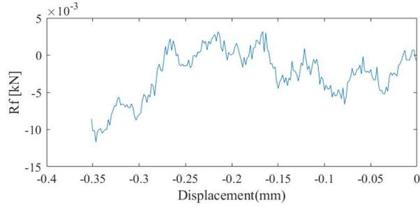
(b) Residual force at the 5<sup>th</sup> iteration of the FEMU-UF calculation
