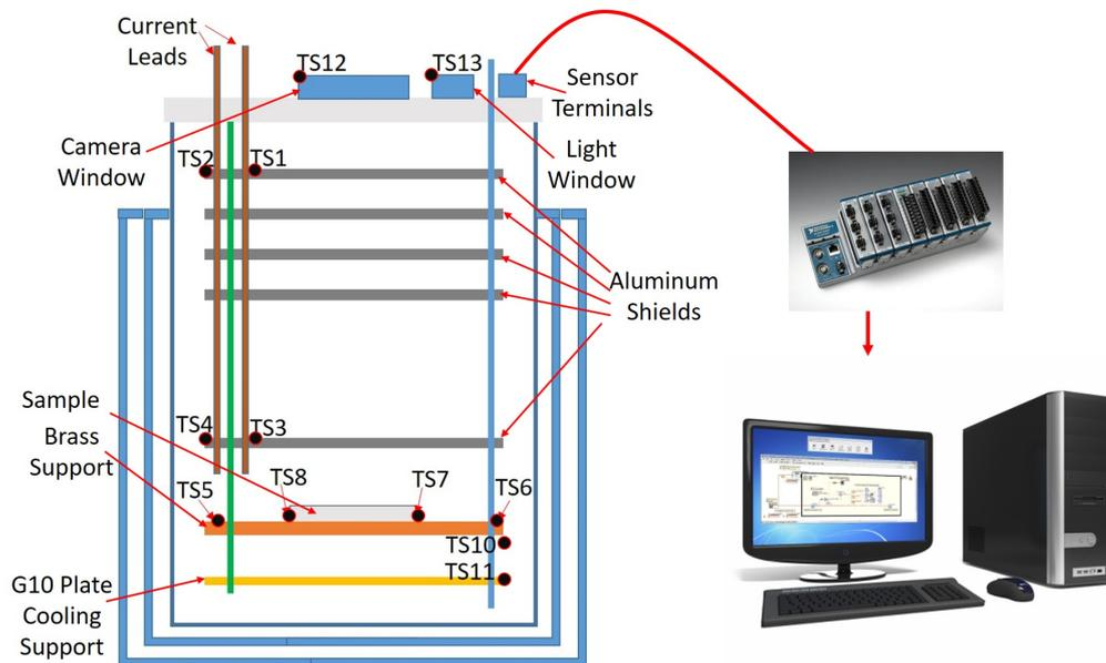
Figure 4.8 – Cooling Setup Instrumentation (TS: Temperature Sensor)
