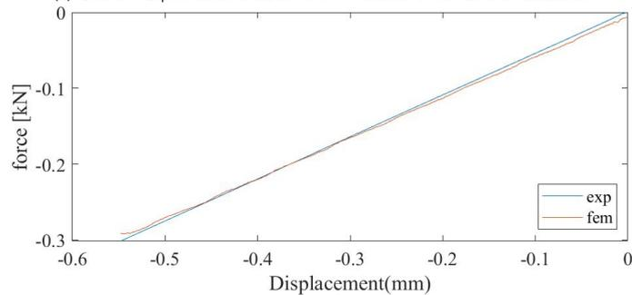
(c) FEMU-UF / Experimental forces at the 64<sup>th</sup> iteration of the FEMU-UF calculation
