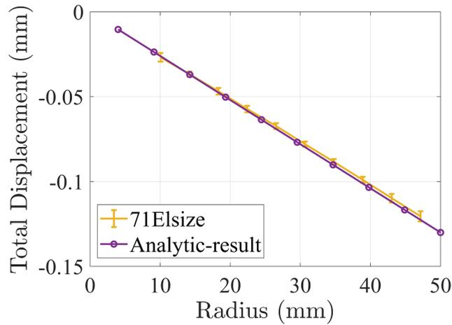
Figure 4.21 – Total displacement magnitude with setup contraction of SS304 disc,  $\alpha_T = -13.86 \times 10^{-4}$  mm/mm
