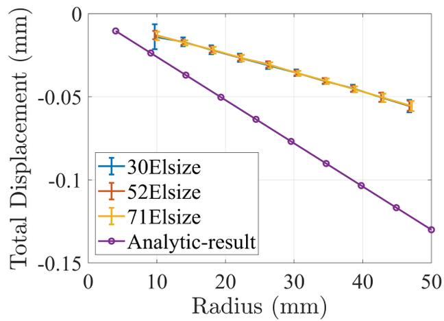
(d) Total displacement (mm) of mesh Elsize 30-52-71 pixels benchmarked with analytic result
