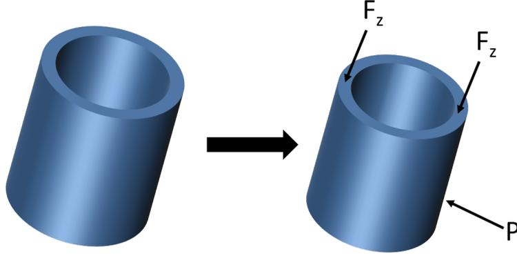
Figure 2.3 - Generalized plane strain deformation scheme
