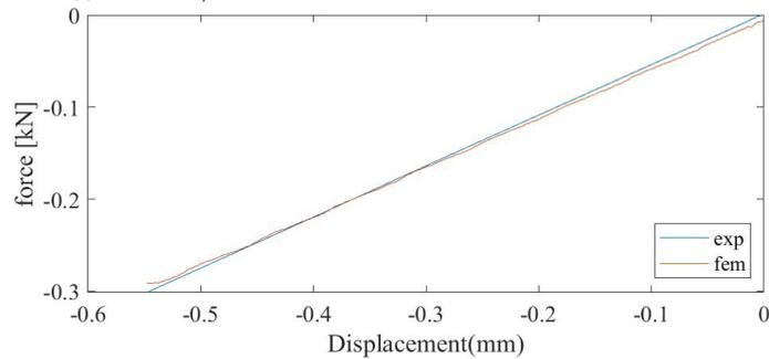
(b) FEMU-UF / Experimental forces at the 30<sup>th</sup> iteration of the FEMU-UF calculation
