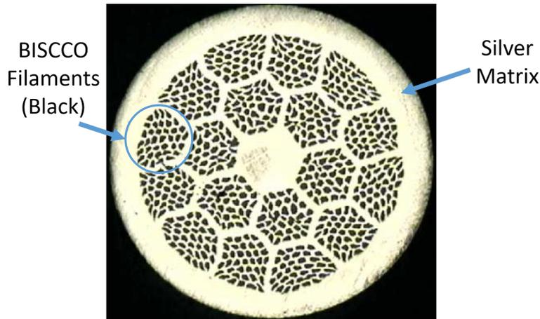
Figure 1.5 – BSCCO 2212 round wire cross section [23]
