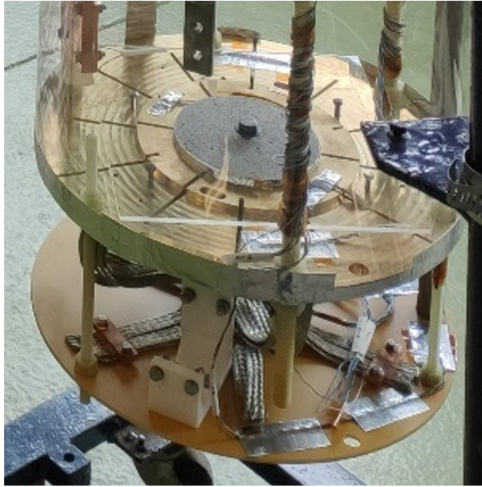
Figure 4.11 – SS304 disc mounted
