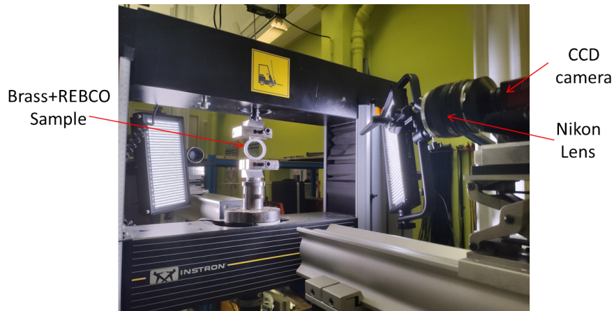
Figure 3.25 – Diametric compression setup of Brass+REBCO
