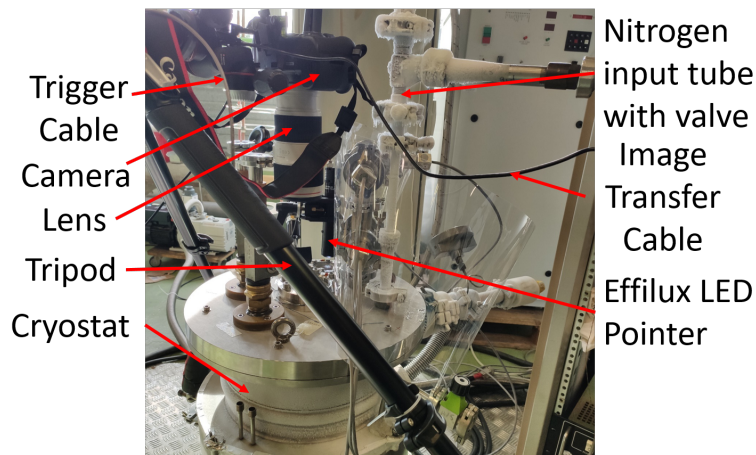
Figure 4.7 - DIC-setup mounted
