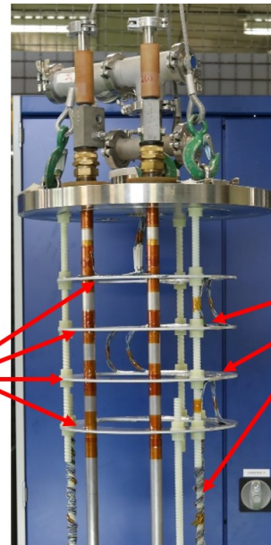
(b) Sensor's wires thermal shielding
