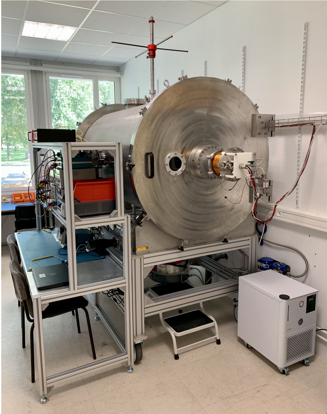
Figure 3.4: The testing facility of LPC2E. The cylindrical vacuum chamber is held by a metallic support frame. The pumping system is installed below the chamber, while the plasma source is attached to the middle of the chamber's door.
