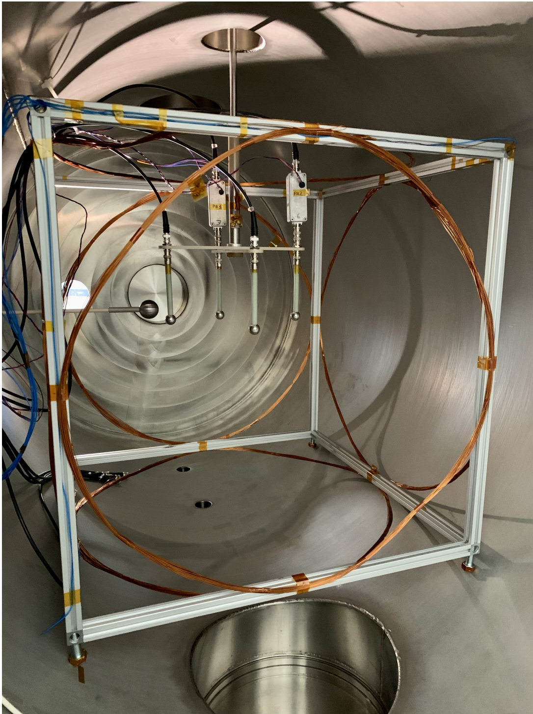
Figure 3.10: Mutual impedance spherical electric sensors inside the plasma chamber, surrounded by the magnetic field compensation system.
