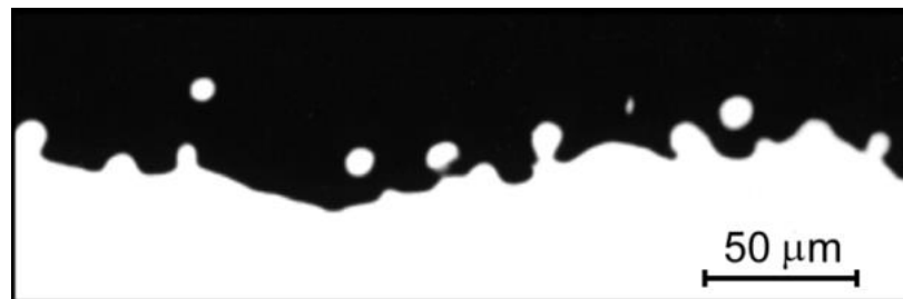
Figure. 1.9 - Correlated nucleation - the formation of a domain chain during switching from a polydomain state in lead germanate in a strong field [35].
