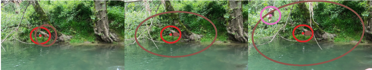
Figure 3.1: Our method: one object (red dot) is correctly detected at every frame and given a consistent identity throughout the sequence with low location uncertainty (red ellipse). Next to it, a false positive detection is generated at the first frame (brown dot) but immediately lost in the following frames: the associated uncertainty grows fast (brown ellipse). In our solution, this type of track will not be counted. A third correctly detected object (pink) appears in the third frame and begins a new track.
