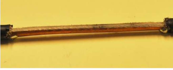
Fig. 3. A two port a vector network analyzer (VNA) is connected to a faulty line through the fixtures A and B .
