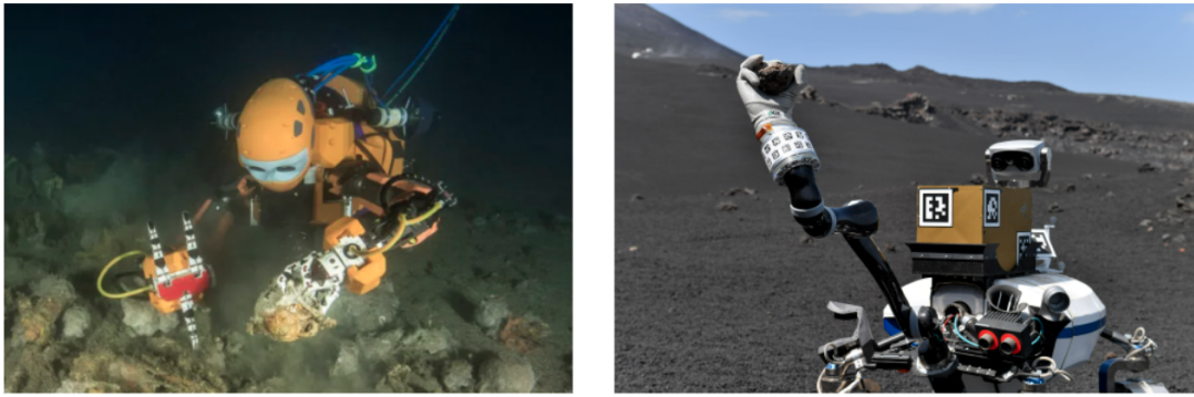
Figure 1.2: Examples of potential applications of tactile exploration of unknown objects. Left: Submarine humanoid handling archaeological object (© https://spectrum.ieee.org/ ). Right: Moon exploring robot taking a rock (© https://www.dlr.de/ )
