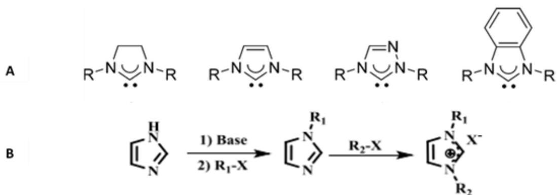
Scheme I-2: [A] Scheme of common NHC structures imidazolin-2-ylidene, imidazole-2-ylidene, triazole-2-ylidene, and benzimidazole-2-ylidene. [B] Synthesis pathway of an imidazolium salt by quaternization of the nitrogen atoms of the imidazole ring with primary alkyl-/aryl- halides in presence of a strong base.
