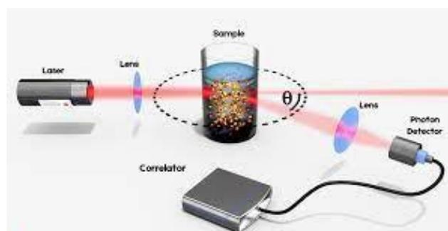
Figure 133. Working principle of dynamic light scattering
