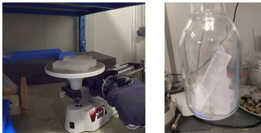
Figure 5.8: Ice samples for Ar dating performed with copper method. Left: Ice weighing in the cold room. Right: Ice in the glass flask ready to be evacuated.
