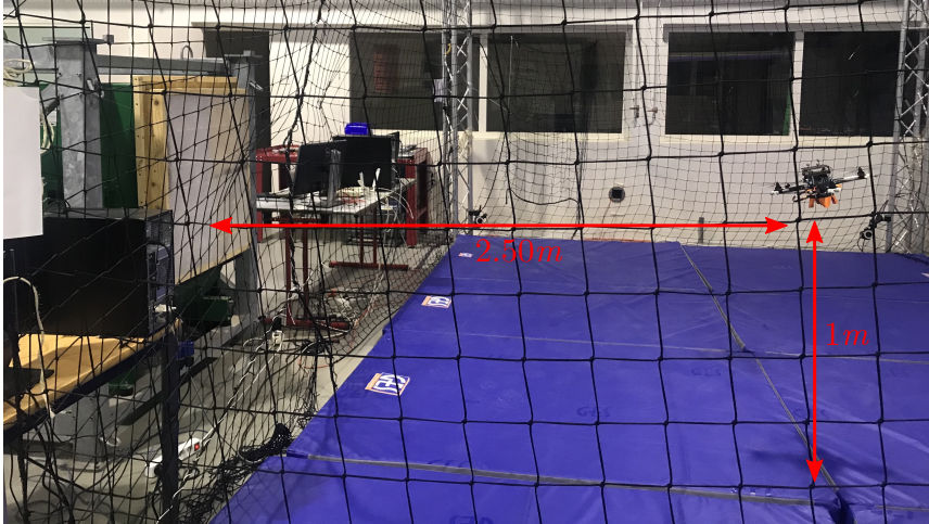
Figure I.4.4: Wind force estimation: quadrotor windswept during the experimental estimation of the aerodynamic force.
