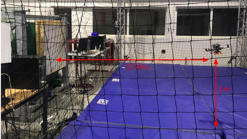
Figure I.4.4: Wind force estimation: quadrotor windswept during the experimental estimation of the aerodynamic force.
