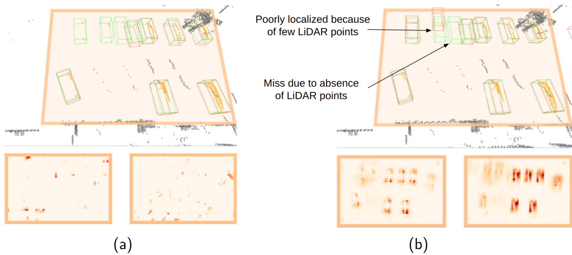
Figure 1.17 – Comparison between BEV images made by SECOND (a) and by SECOND enhanced by Sparse-to-Dense (b). The upper row shows the detected objects colored in red and ground truth colored in green. This image is in the custody of [115].
