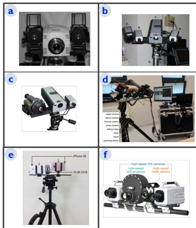
Figure 5.6: Stationary thermal 3D model systems. Images obtained from [92] (a), [89] (b), [23] (c), [93] (d), and [94] (e), [95] (f).
