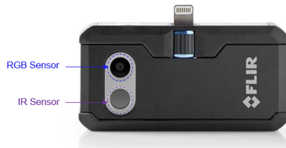
Figure 5.3: FlirOne Pro thermal camera. In this camera, RGB and IR sensors are in fixed relative positions.
