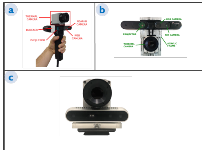
Figure 5.7: Portable thermal 3D model creation systems. Device images obtained from [96] (a), [97] (b), and [98] (c).
