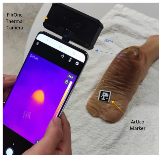
Figure 6.10: Illustration of handheld image acquisition using portable devices in clinical settings for creating thermal 3D models of wounds.
