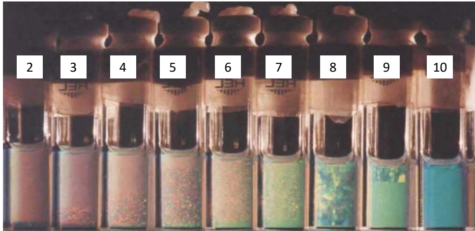
Figure 2: [Pusey and Van Megen (1986)]: Suspension of nearly hard sphere colloids 4 days after preparation. The volume fraction of colloids increases from left to right, from \phi = 0.393 to \phi = 0.52 . The sample are illuminated from behind with bright light such to visualize the Bragg reflection for the crystalline phase. The cross section of the vial is 1 \text{ cm} \times 1 \text{ cm} .
