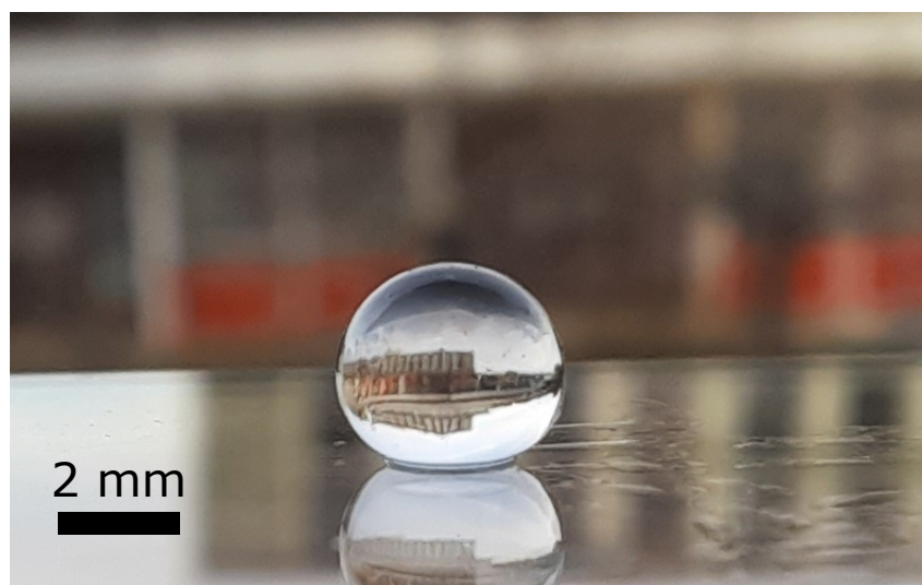
Figure 38: Image of a colloidal bead of gel on the top of a glassy slide prepared at volume fraction \varphi = 10\% . The scale bar is the same for all images
