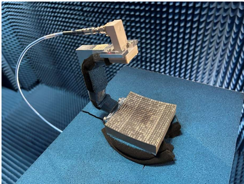
Fig.3.48 Photographs of manufactured MORRA and its measurement setup.
