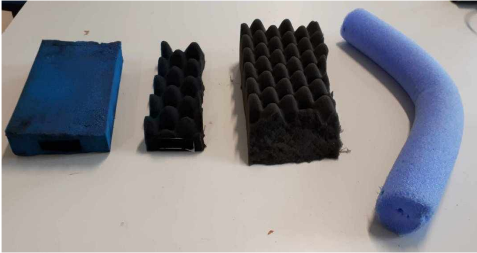
Figure 4.16: Different foam objects used during the experiments. From left to right: sponge, thin convoluted foam, convoluted foam, foam noodle.
