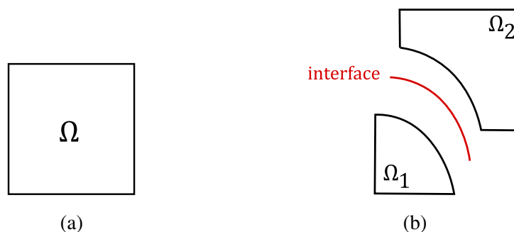
Figure 1.2: Example of Schur domain decomposition of the global domain \Omega (a) into two subdomains \Omega_1 and \Omega_2 (b).
