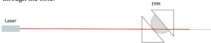
Figure A.3: The laser beam must pass through the hole of the FPM mask.
