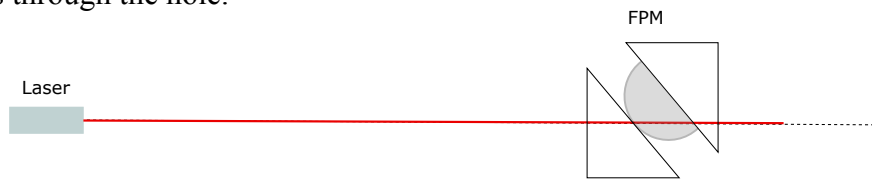
Figure A.3: The laser beam must pass through the hole of the FPM mask.
