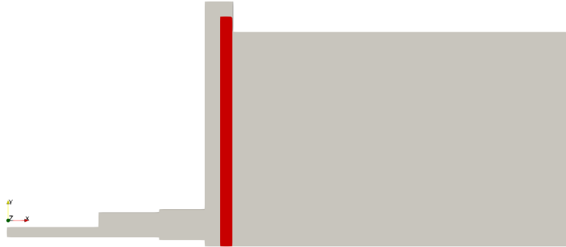
Figure 6.2: CAD model of the cavity (grey) and rotor disk (red).
