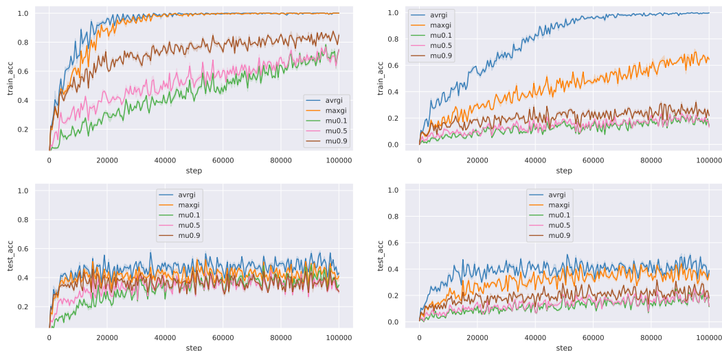
Figure 2.4: CIFAR100: Training (top) and test (bottom) accuracies for adagrad -like ( \mu \in (0.1, 0.5, 0.9) ), maxgi and avrgi variants with \alpha = 5.10^{-4} (left) and \alpha = 5.10^{-5} (right) on the resnet18 architecture
