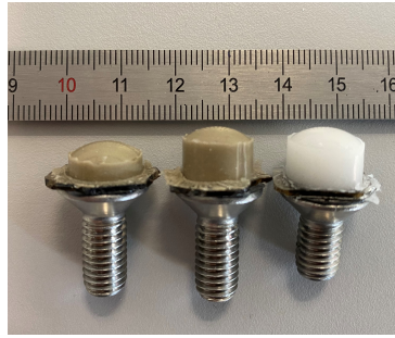
Figure 2.8: Picture of some of the used samples. From left to right a 6 mm high 10:1 PDMS filled with aluminium particles (B-10-A), a 9 mm high 10:1 PDMS filled with aluminium particles (A-10-A) and a 9 mm high 20:1 PDMS filled with glass particles (A-20-G).
