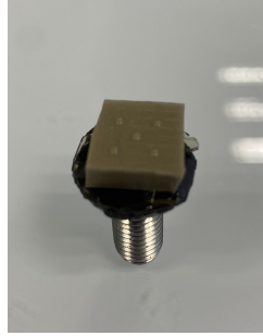
Figure 5.1: Picture of a multi-asperity specimen used for XRCT experiments. The specimen in the photo is composed of a PDMS bulk filled with aluminium particles.
