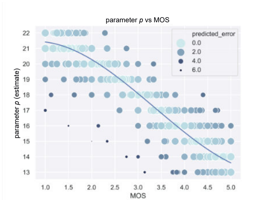
Figure 5.12: Polynomial regressions for estimating the visual security parameter p .
