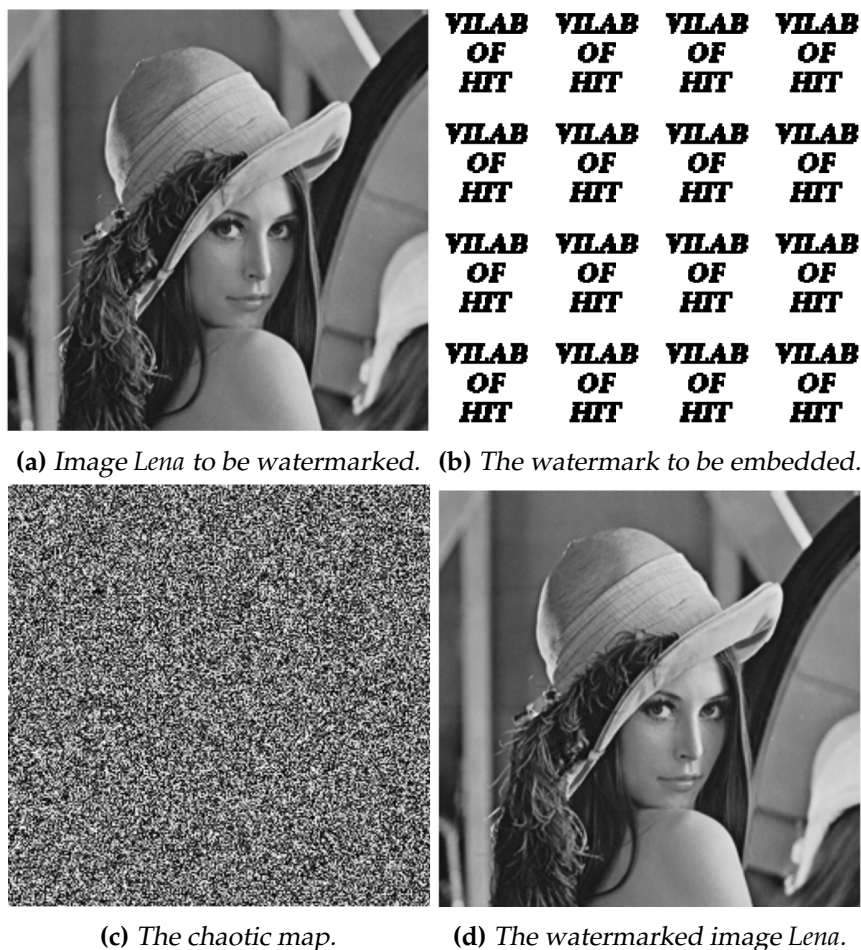
Figure 2.8: An illustration of (88): a) The original 256 \times 256 size image Lena , b) The watermark to be embedded, c) The chaotic map, d) The resulting watermarked image Lena with a PSNR of 51.13 dB.
