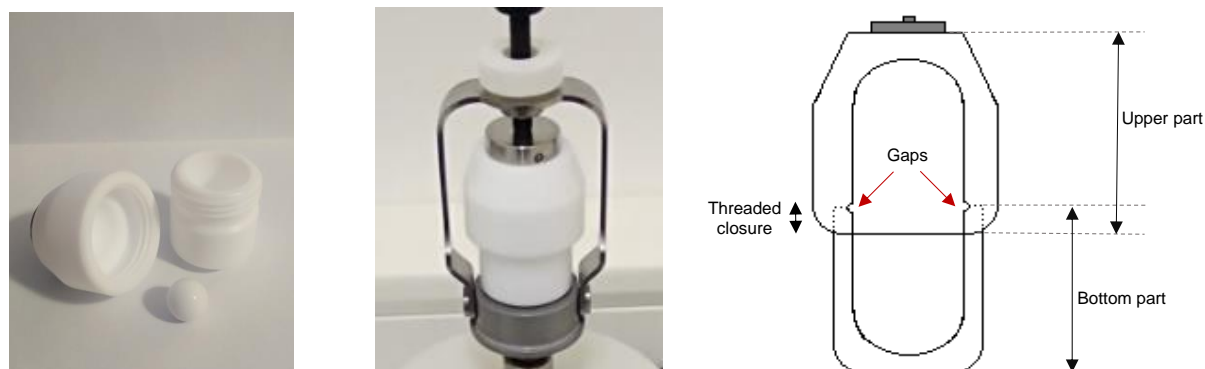
Figure II-45: Photos and a scheme of PTFE (5 mL inner volume, Fritsch) jar used for enrichment of unsaturated FAs (LA, ALA, AA). Due to the beveled edge at the contact planes of both parts of the jar, a gap is created where the two parts of the jar meet. During the milling experiments, small portion of a reaction mixture remains stuck in this gap and cannot interact with the labeled water, thus remains not labeled. During the work-up, this non-labeled portion is included into the final product and very probably causes a decrease of the overall enrichment of isolated products.
