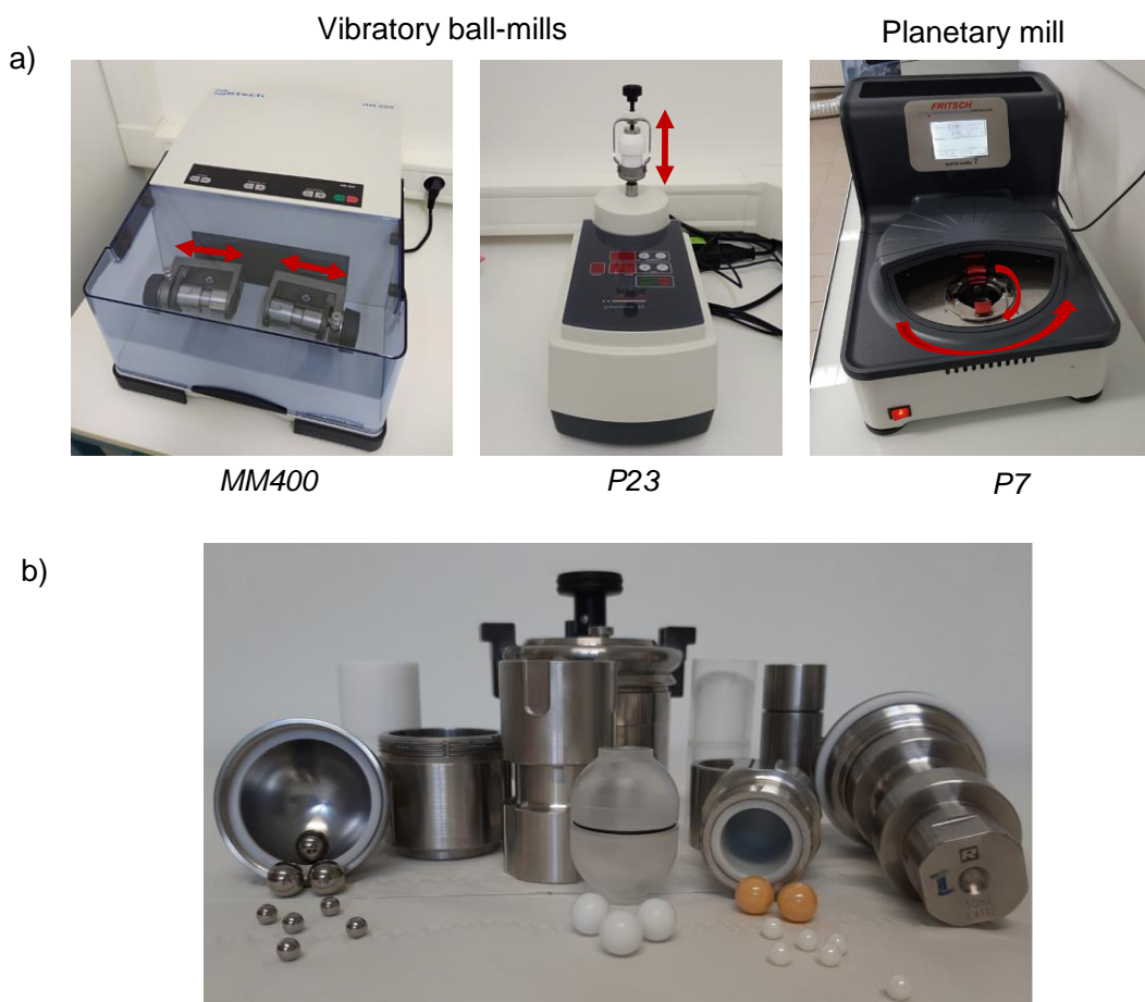
Figure 1.7: a) Commercial ball-mill machines used during this thesis, with the red arrows symbolizing the induced movement, and the product brand names indicated below the instruments, i.e. MM400 (horizontal shaking), P23 (vertical shaking), P7 (planetary movement). b) Examples of mechanochemical equipment available at the laboratory during the course of this thesis: reaction vessels (jars) and milling beads of different size, and made of different materials.
