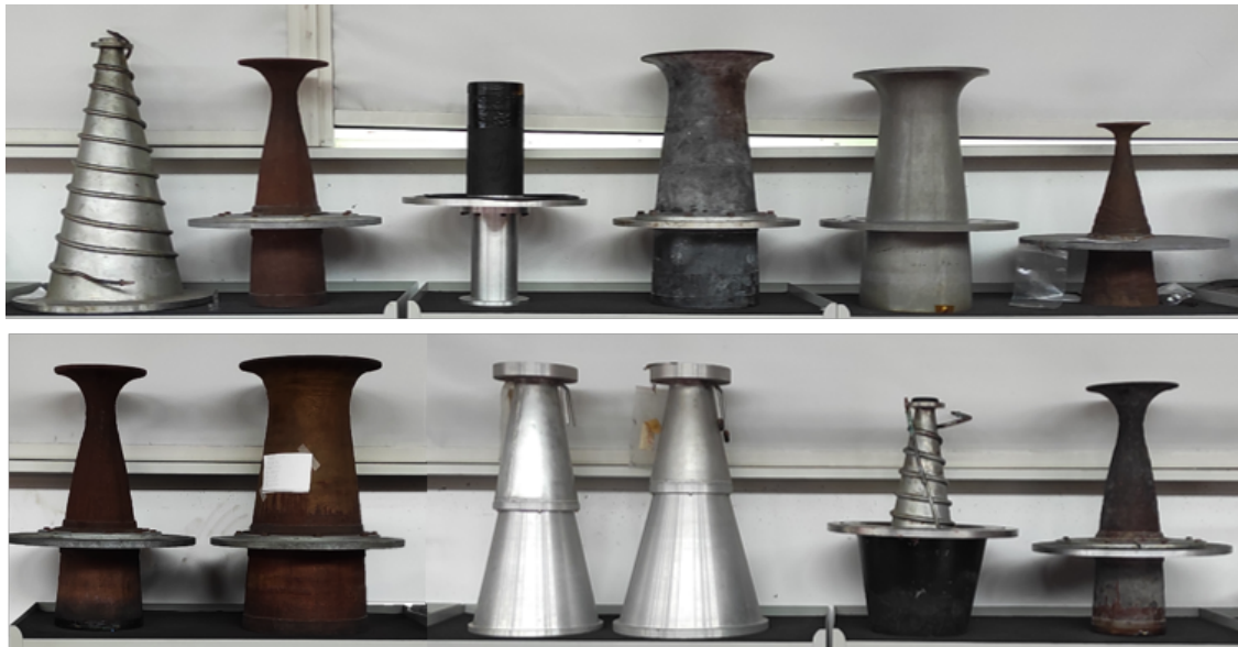
Figure 4.3: Pictures of some nozzles of the MARHy wind tunnel.
