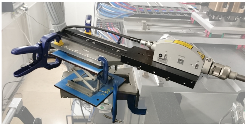
Figure C.1 | System used to support the laser vibrometer installed on ID19 beamline in ESRF synchrotron.
