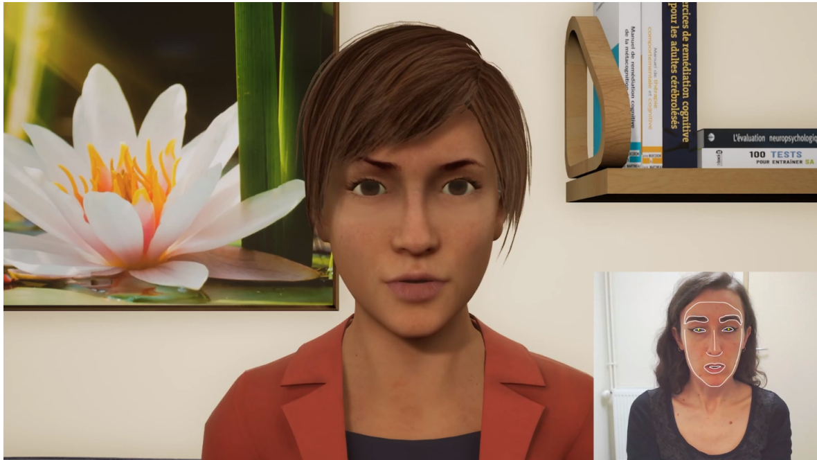
Figure A.1: Animation of the virtual agent by the tracking of visual features on the video recording.
