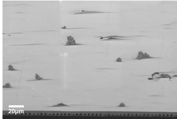
**Figure 4- 8:** A tilted SEM image after 1h of GaN coalescence growth for a sample having 100nm SiO<sub>2</sub> thickness and 50nm AlN.
