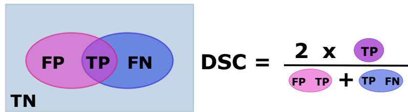
Figure 2.1: Representation of Dice similarity coefficient. TP represents the number of true positives predictions, FP and FN the number of false positives and false negatives, respectively
