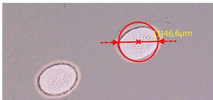
Figure 92. Smallest observed crystallized zone using the VarioSCAN system.
