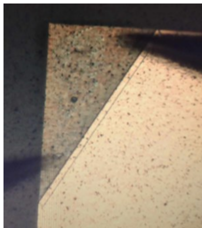
Figure 154. Optical image of the irradiated GeTe edge of the array of antennas. The black features are the out-of-focus probes.
