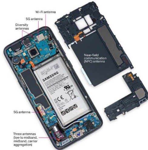
Figure 4. Typical distribution of the different antennas in a smartphone. Taken from [16].
