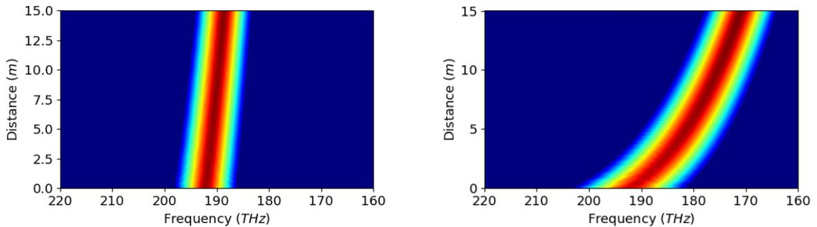
(a) Spectra of a 120 fs soliton pulse as a function of length. (b) Spectra of a 60 fs soliton pulse as a function of length.
