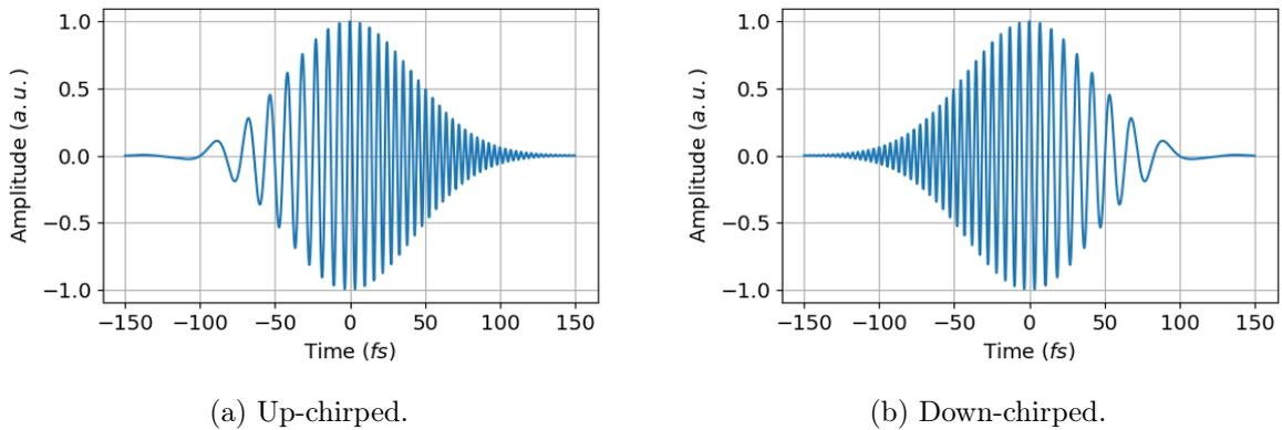
Figure 1.3: Electric field of a chirped Gaussian pulse.
