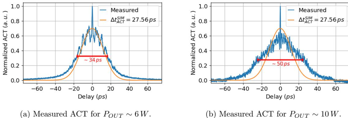
Figure 4.10: Measured ACT out of the second Tm:Ho 6/130 pre-amplifier. Dispersion mismatch between CVBGs and dispersion due to fiber amplifiers have not been compensated with PM2000D fiber.
