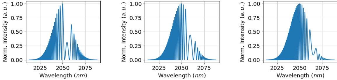
(a) Simulated spectrum of a pair of identical pulses with delay  $\phi_1 = 4 \text{ ps}$
