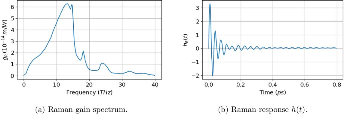
Figure 1.8: Raman gain spectrum and Raman response. Data taken from [101].
