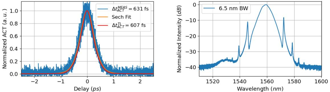
(a) Measured autocorrelation trace.  $\Delta t_{FWHM}^{SECH} = 402$  fs
