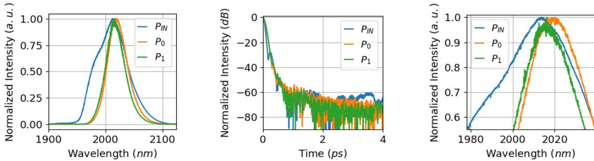
(a) Measured amplified ASE in Tm 6/130 doped fiber amplifier. (b) FFT of the measured amplified ASE in Tm 6/130 doped fiber amplifier for time scale below  $4\ \text{ps}$  (c) Measured amplified ASE zoomed image.
