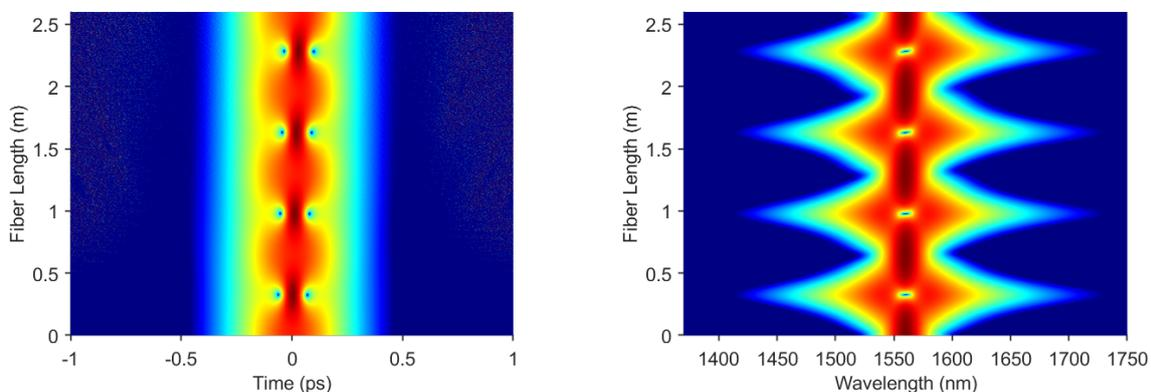
(a) Pulse shape as function of propagation length. (b) Spectrum as a function of propagation length.
