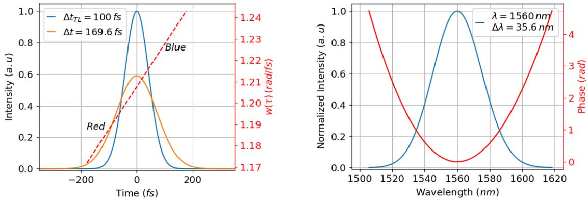
(c) Normal dispersion with  $\phi_2(w) = +5000 \text{ fs}^2$ . Red spectral components travel faster than blue. (d) Normal dispersion with  $\phi_2 = +5000 \text{ fs}^2$ ,  $\lambda_0 = 1560 \text{ nm}$  and  $\Delta\lambda = 35 \text{ nm}$ .
