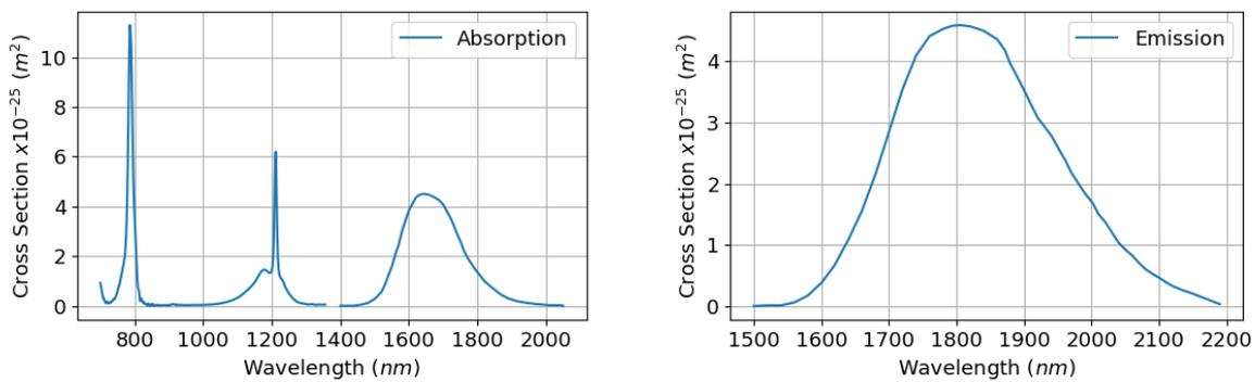
(a) Tm absorption cross section.
