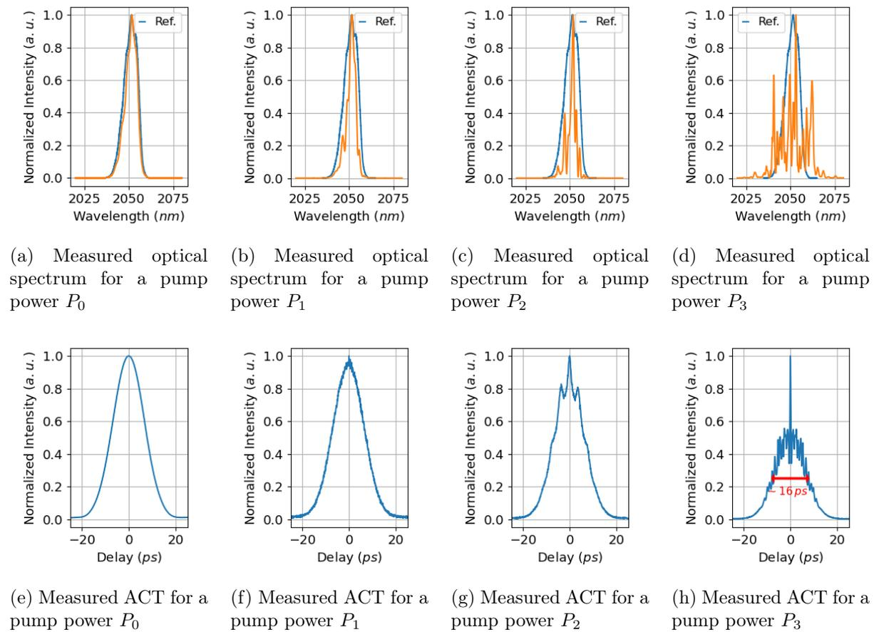
Figure 4.18: Measured optical spectra and ACT out of the Tm:Ho amplifier for different pump powers ( $P_0 < P_1 < P_2 < P_3$ ). The CFBG was used pulse stretcher and Ref. states for the input spectrum to be amplified.
