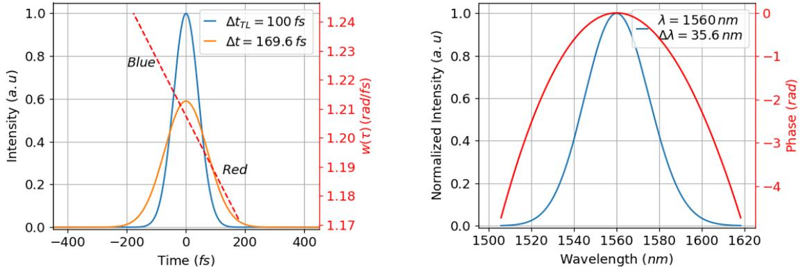
(a) Anomalous dispersion with  $\phi_2(w) = -5000 \text{ fs}^2$ . Blue spectral components travel faster than red. (b) Anomalous dispersion with  $\phi_2 = -5000 \text{ fs}^2$ ,  $\lambda_0 = 1560 \text{ nm}$  and  $\Delta\lambda = 35 \text{ nm}$ .
