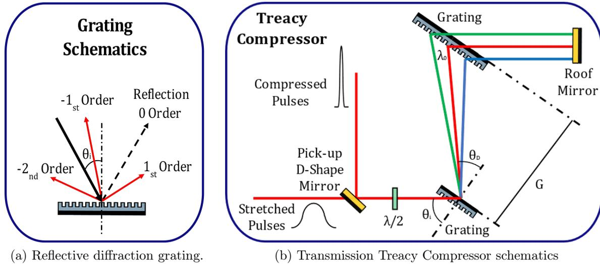
Figure 3.4: Diffraction grating and Treacy compressor schematics.
