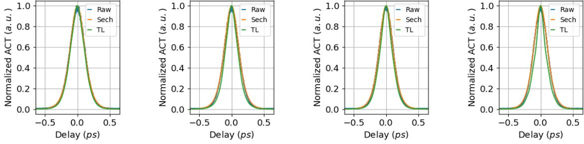
(a) ACT  $\lambda_0 = 2050 \text{ nm}$   $\Delta t_{ACT} = 265 \text{ fs}$   $\Delta t_{PULSE}^{sech} = 171 \text{ fs}$
