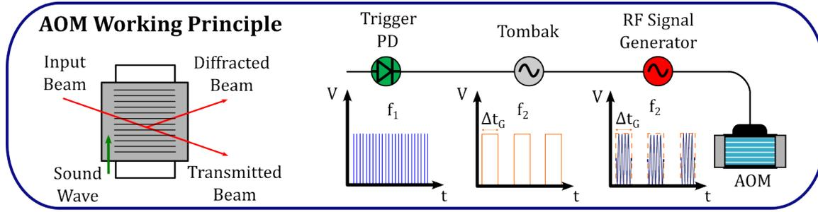
Figure 3.22: AOM working principle and configuration.
