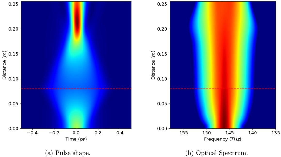
Figure 2.28: Simulated temporal and spectral pulses at  $2050\text{ nm}$  along the spectral broadening and compression stage. Fiber splice location is dashed in red.
