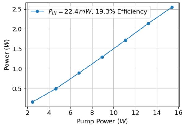
Figure 4.6: Measured output power out of the Tm:Ho 6/130 doped fiber for  $22.4\text{ mW}$  input power.
