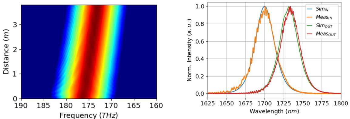
(a) Simulated spectrum as function of the fiber length.
