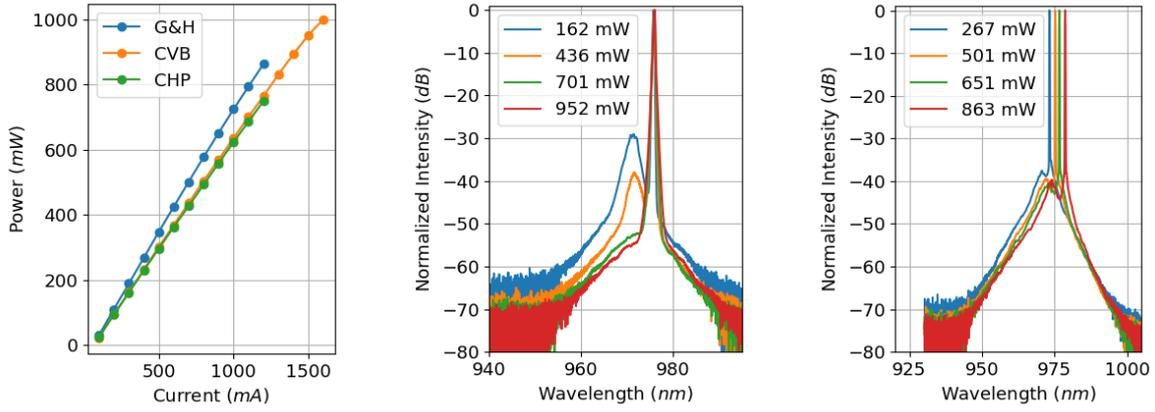
(a) Pump power as function of current. (b) Optical spectrum of CVB pump diode. (c) Optical spectrum of G&H diode.
