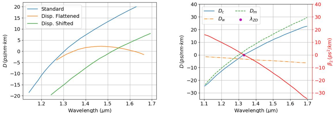
(a) Dispersion for standard, dispersion flattened and dispersion shifted optical fibers
