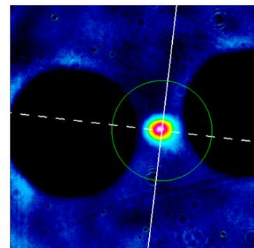
(b) Image of the injected Tm:Ho 6/130 active fiber.
