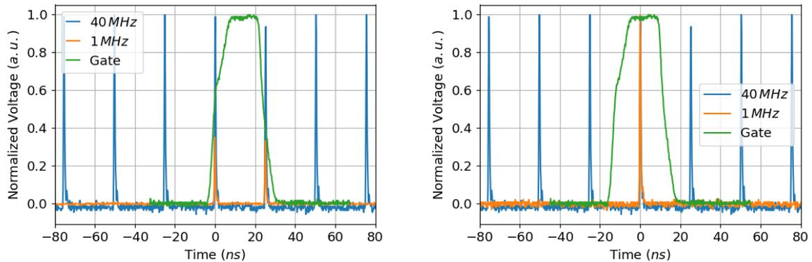
(a) Photodiode signal after pulse picking with gate that is not centered with the picked pulse. (b) Pulse picked photodiode signal with high adjacent pulse suppression.
