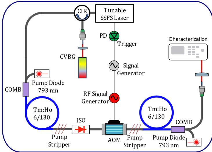
(a) Experimental setup for pre-amplification of the pulse-picked stretched  $ns$  pulses.
