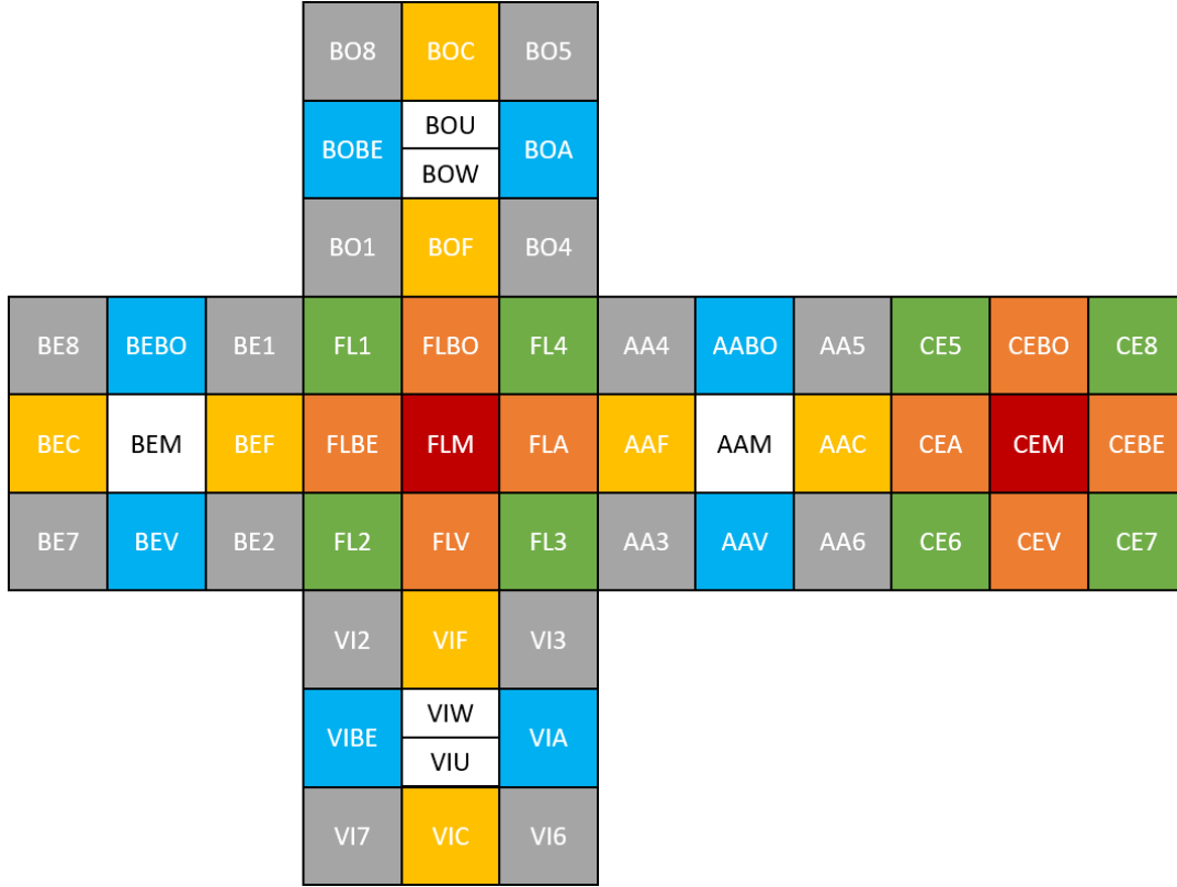
FIGURE 9.10: Flattened representation of the trim coil array. Each color corresponds to an invariant set of coils under the ideal coil symmetries. Only the white coils are not invariant. Around each colored coil, a current flows in either the clockwise or counter-clockwise direction. Note that the grey coils have not been entirely mapped and are therefore not used in the analysis.
