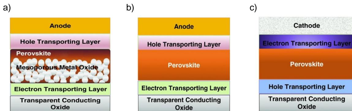
Figure I.14: Schematic of perovskite optoelectronics for different architectures<sup>[57]</sup> a) mesoporous, b) planar, and c) inverted planar structure
