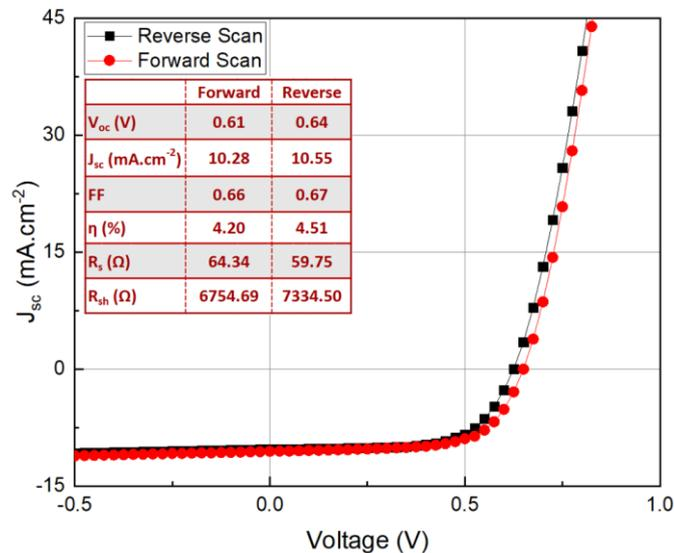
Figure IV.19 : J-V characteristic of the device with evaporated-PC<sub>61</sub>BM as the ETL
