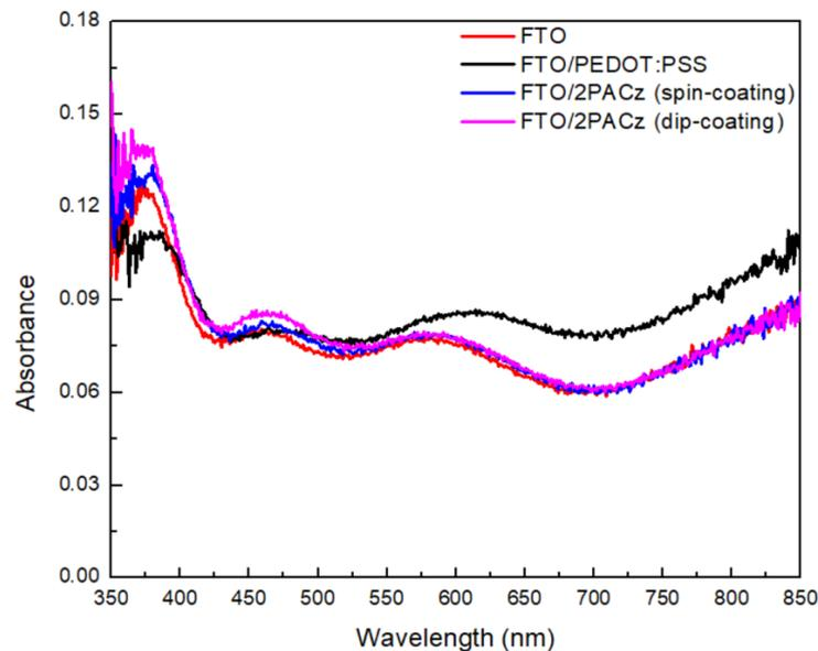
Figure IV.11: Absorbance spectra of PEDOT:PSS and 2PACz (spin-coating and dip-coating)
