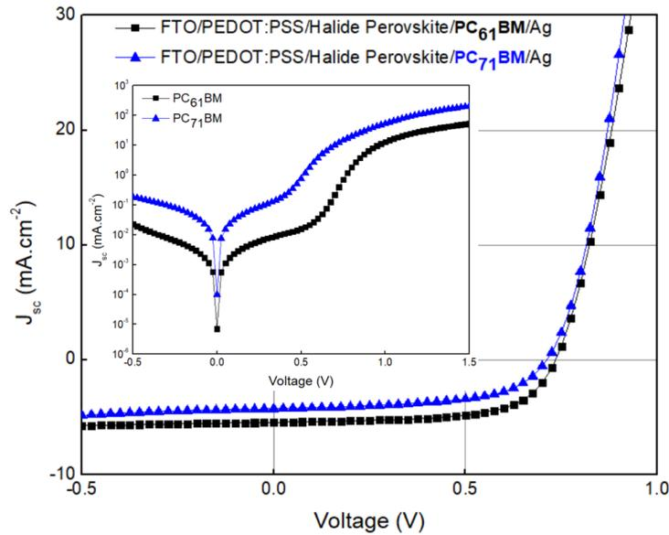
Figure IV.18: J-V characteristic of devices with PC<sub>61</sub>BM and PC<sub>71</sub>BM as the ETL, Inset: dark current in semi-log scale
