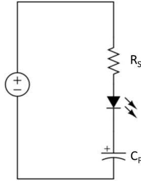
Figure I.12: The equivalent circuit of LED
