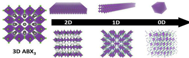
Figure I.2: 3D and low-dimensional hybrid perovskites<sup>[16]</sup>
