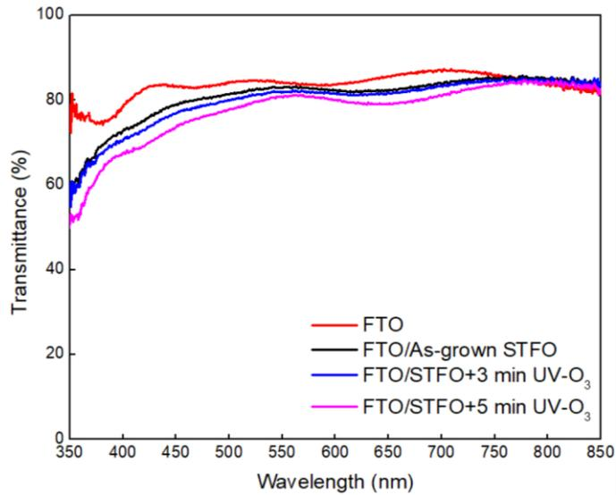
Figure V.3: The effect of UV-O<sub>3</sub> treatment on the optical transparency of as-grown STFO thin film
