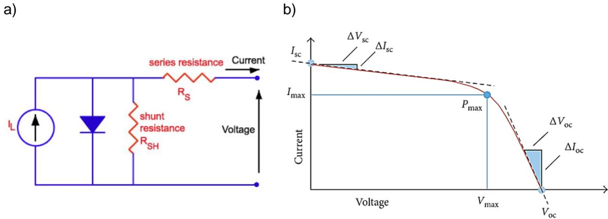
Figure I.11 : Solar cell a) equivalent circuit<sup>[51]</sup> and b)  $R_{sh}$  and  $R_s$  extraction from the I-V curve<sup>[54]</sup>
