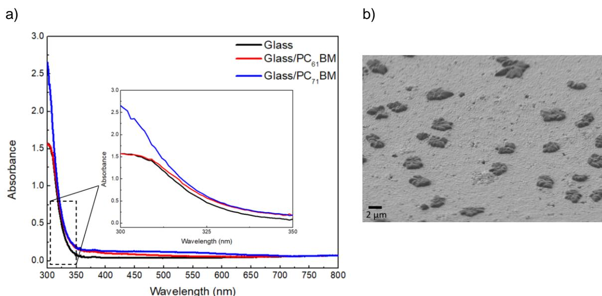
Figure IV.17 : a) Absorbance spectra of PC<sub>61</sub>BM and PC<sub>71</sub>BM, and b) PC<sub>71</sub>BM morphology on top of CsFAPbI<sub>3</sub> perovskite
