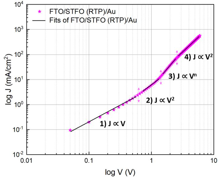
Figure III.16: Log-log scale J-V characteristics of STFO (RTP)
