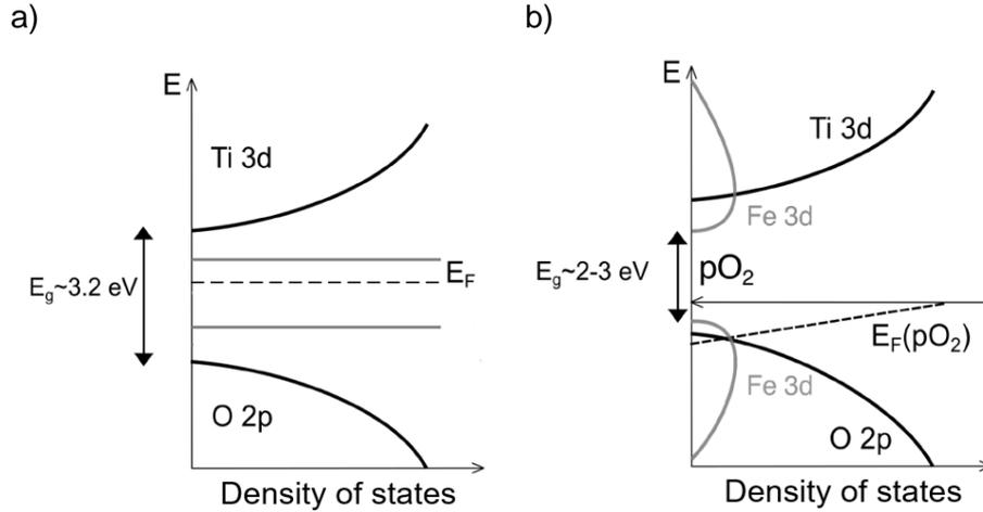
Figure II.3 : The schematic of changing bandgap of STO a) pre-doping and b) post-doping of Fe<sup>[203]</sup>
