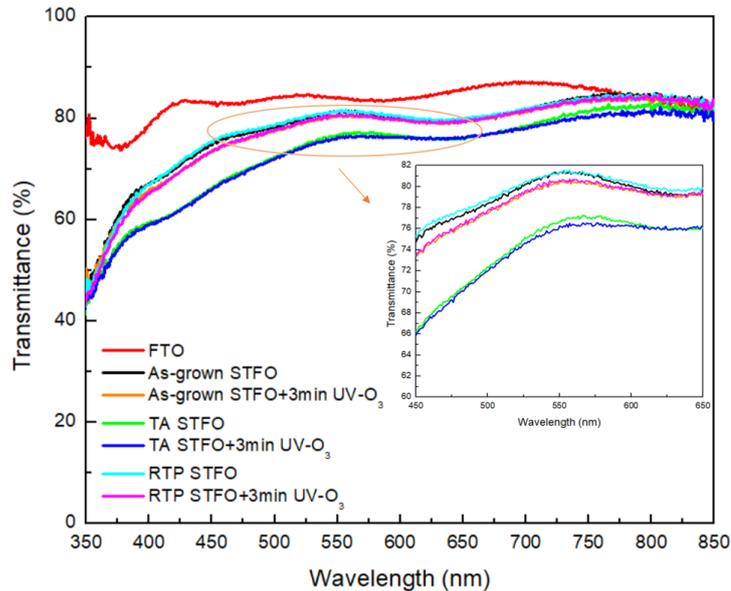
Figure V.4: The effect of UV-O<sub>3</sub> treatment (3 minutes) on the optical transparency of as-grown, RTP, and TA STFO thin films
