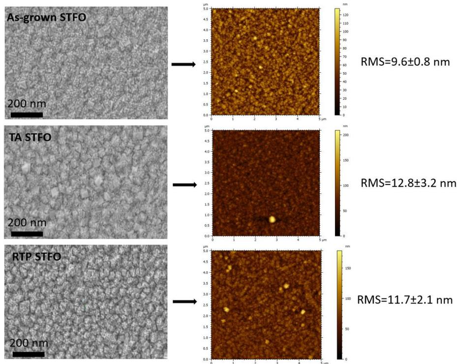
Figure III.10: SEM and AFM images in terms of the effect of additional thermal treatment on the STFO
