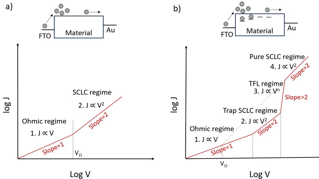
Figure III.12: Schematic statement of principle a) pure SCLC regime and b) trap-filled limited regime
