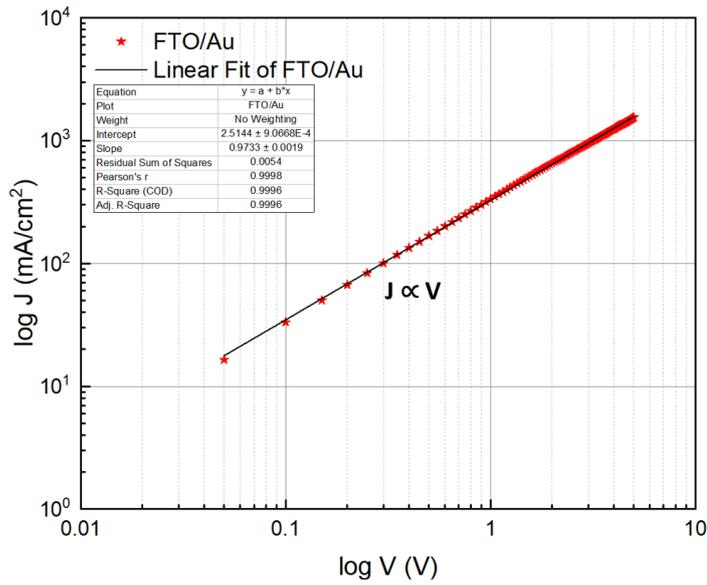
Figure III.14: Log-log scale J-V characteristics of FTO
