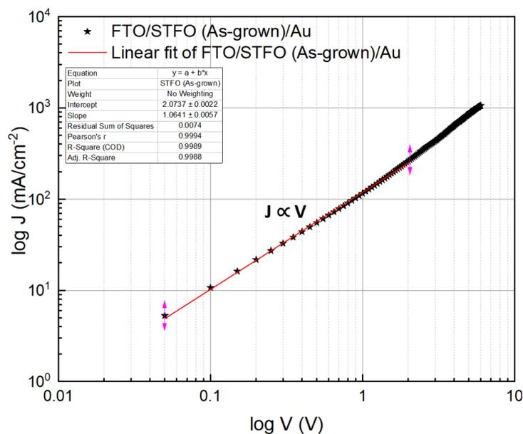
Figure III.15: Log-log scale J-V characteristics of STFO (as-grown)
