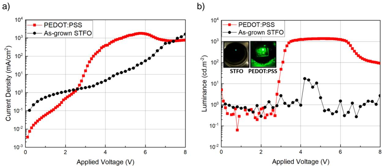
Figure V.19 : a) J-V and b) L-V curves of PeLEDs with reference PEDOT:PSS and as-grown STFO thin films (Inset: Image of operational as-grown STFO and PEDOT:PSS-based PeLED with emission at the edge of the device)
