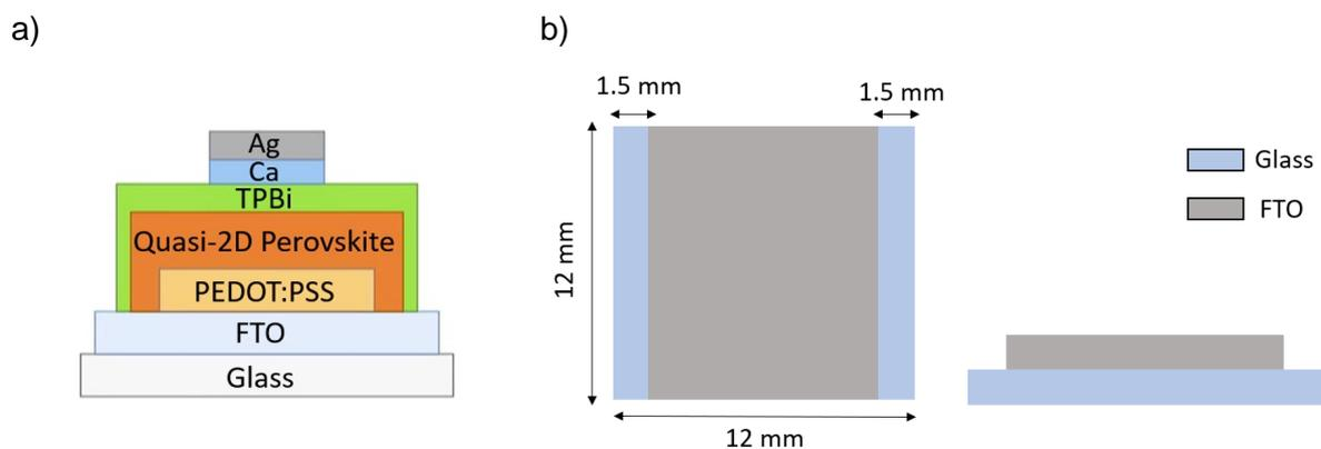
Figure IV.33 : a) Final device structure and b) the design of FTO for the wet etching process of device
