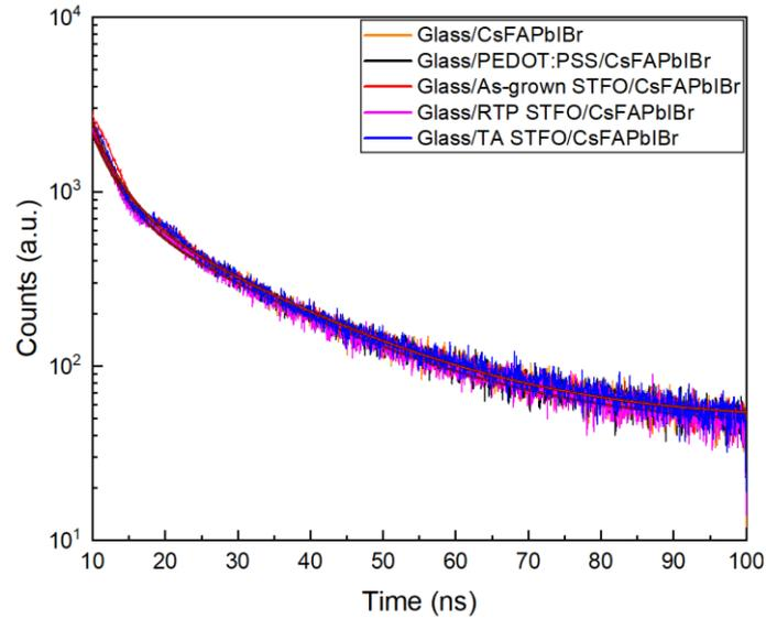
Figure V.9 : Time-resolved PL decay curves of CsFAPbI<sub>3</sub> perovskite layer alone and on PEDOT:PSS, as-grown STFO, RTP STFO, and TA STFO thin films
