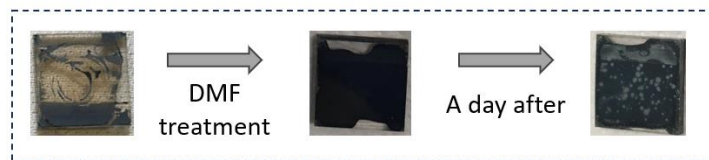
Figure IV.7 : The wettability of CuSCN and fast degradation problem of halide perovskites
