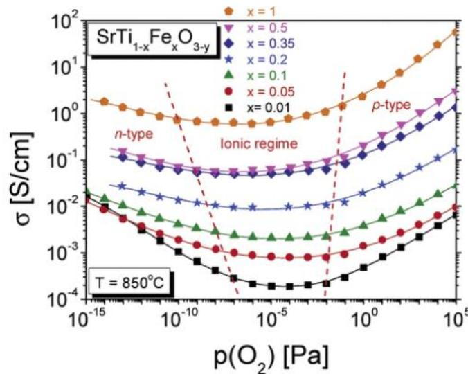
Figure II.2 : Variation of the electrical conductivity with different oxygen partial pressures for STFO compositions<sup>[202]</sup>
