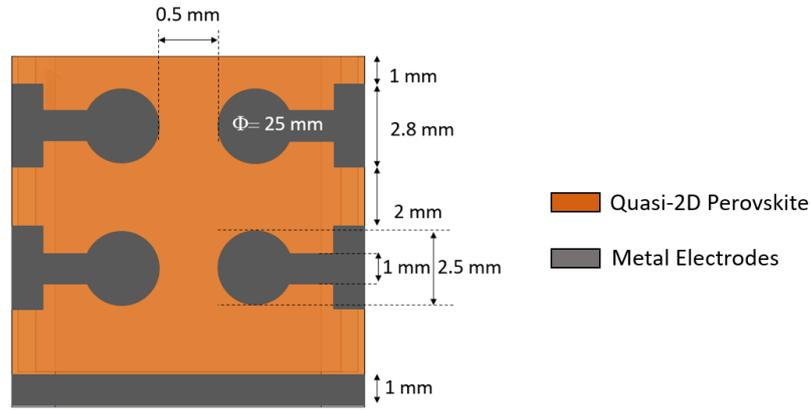
Figure IV.35 : The final design of the PeLED
