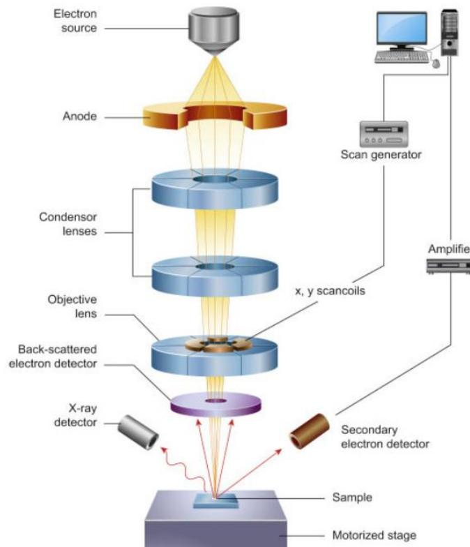
Figure A. 5: Principle of the scanning electron microscopy<sup>[354]</sup>
