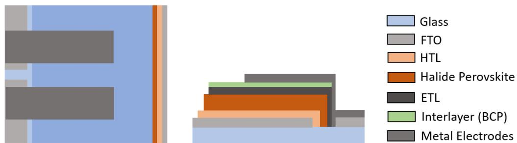
Figure IV.29 : The design of metal electrodes on the ETL
