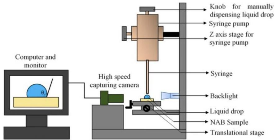
Figure A. 10: Principle of the contact angle measurement<sup>[359]</sup>
