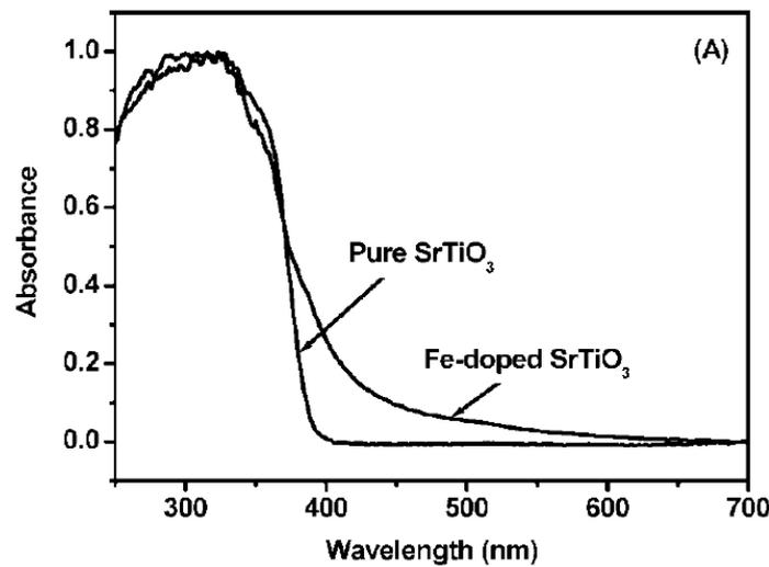
Figure II.4: The absorbance spectra of undoped and Fe-doped STO<sup>[204]</sup>
