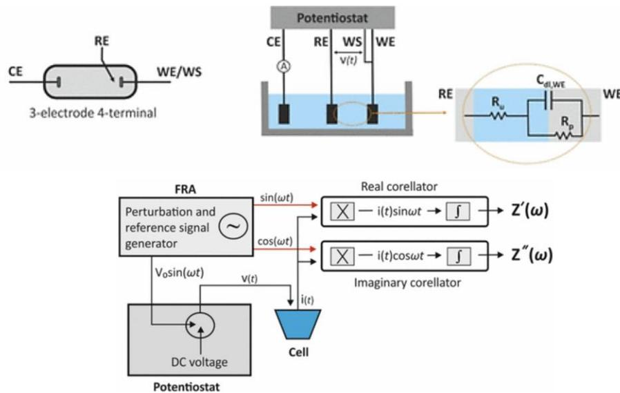
Figure A. 9: Principle of the electrochemical impedance spectrometer<sup>[358]</sup>
