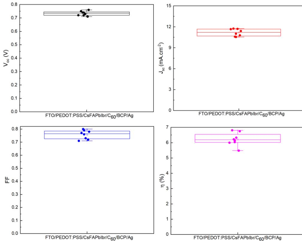
Figure IV.24 : Statistical properties of PV performance parameters in a set of 8 PSC devices
