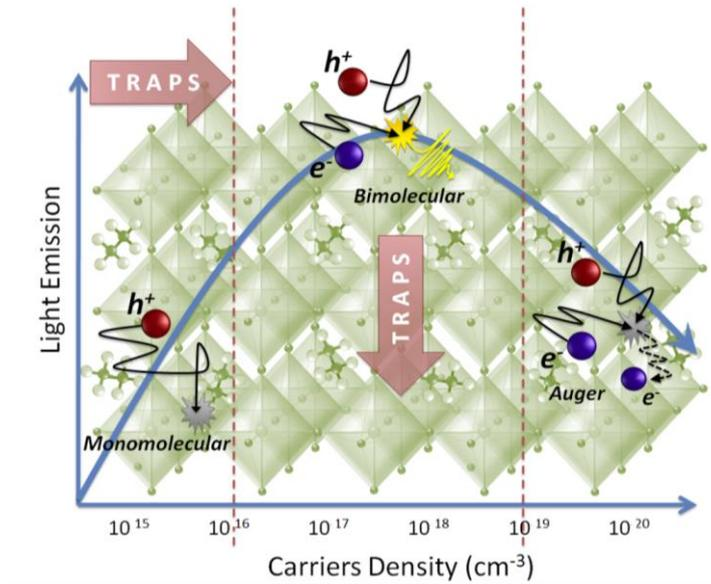
Figure I.13: Schematic representation of charge carrier regimes<sup>[55]</sup> SRH, bimolecular, and Auger recombination
