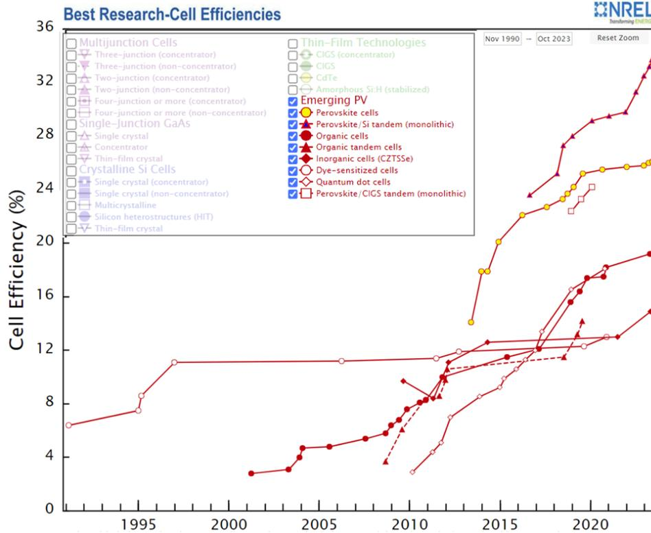
Figure I.5: The performance variation of perovskite solar cells<sup>[40]</sup>
