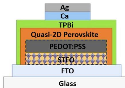
Figure V.21 : PeLED device structure using STFO/PEDOT:PSS as HTL
