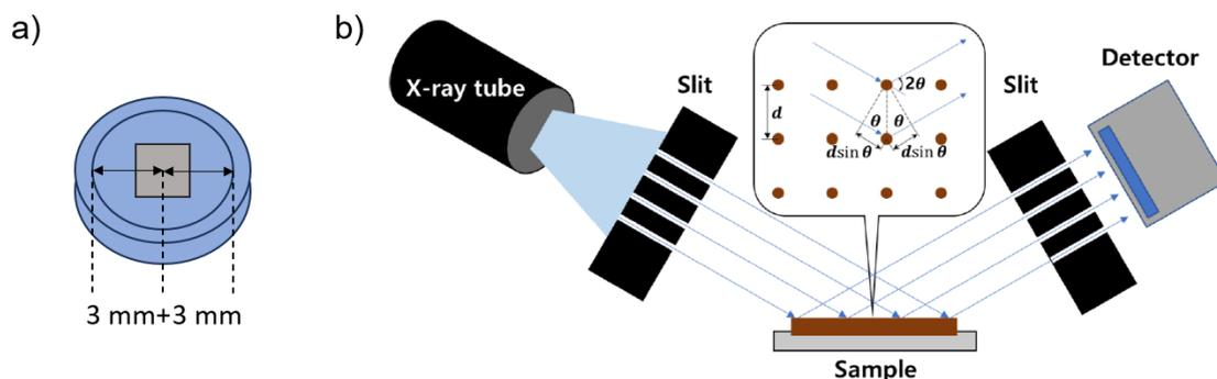
Figure A. 4: XRD analysis of a) the sample preparation on a holder b)  $2\theta$ - $\theta$  scan<sup>[353]</sup>
