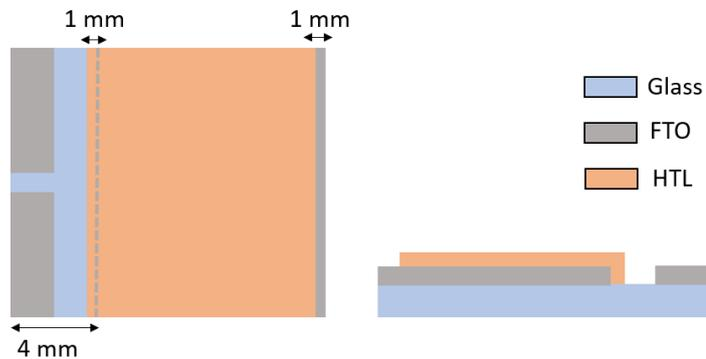
Figure IV.26 : The design of HTL for the etching process on the FTO substrate
