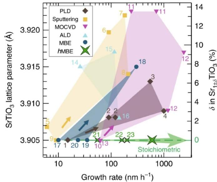
Figure II.6: Growth rate and stoichiometry control of STO for different deposition methods (the numbers serve as references utilized in the research)<sup>[223]</sup>
