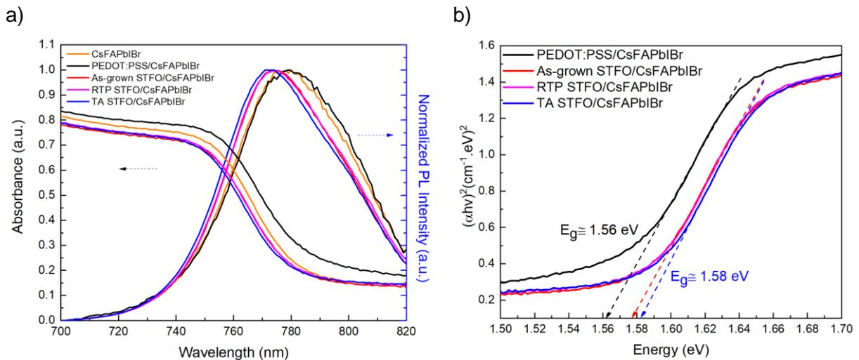
Figure V.8 : a) UV-Vis absorbance and normalized steady-state PL spectra and b) Tauc's plot of CsFAPbI<sub>3</sub> perovskite layer on PEDOT:PSS, as-grown STFO, RTP STFO, and TA STFO
