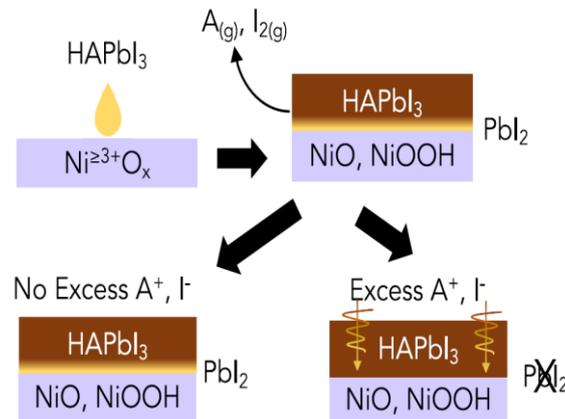
Figure I.24: The redox reaction between the NiO<sub>x</sub> and perovskite precursor<sup>[140]</sup>
