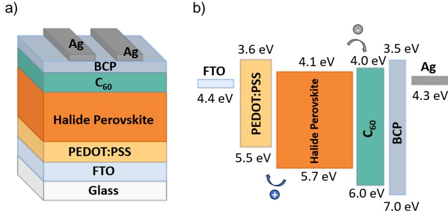
Figure IV.22 : PSC's a) device architecture with C<sub>60</sub> as the ETL and b) energy-band diagram
