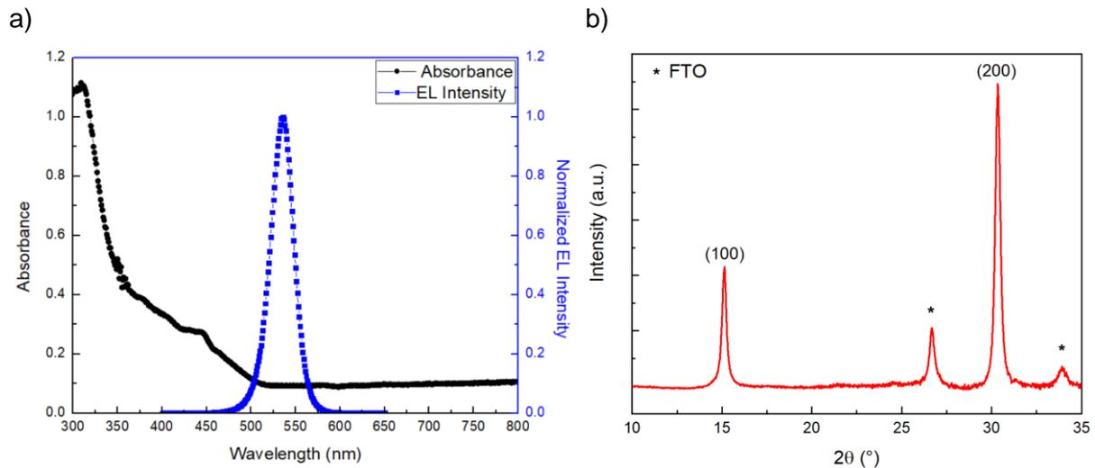
Figure IV.30 : (PEA)<sub>2</sub>(MA)PbBr<sub>4</sub> type quasi-2D perovskite a) absorbance spectra and EL spectra and b) XRD pattern on FTO
