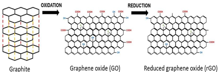
Figure I.27: Oxidation and reduction process of graphene<sup>[178]</sup>
