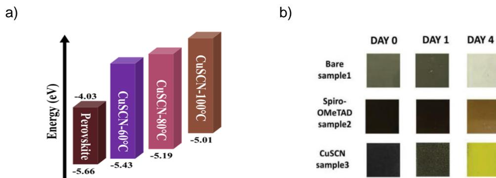
Figure I.25: a) The temperature affects the energy diagram<sup>[117]</sup> and b) degradation of CuSCN<sup>[151]</sup>
