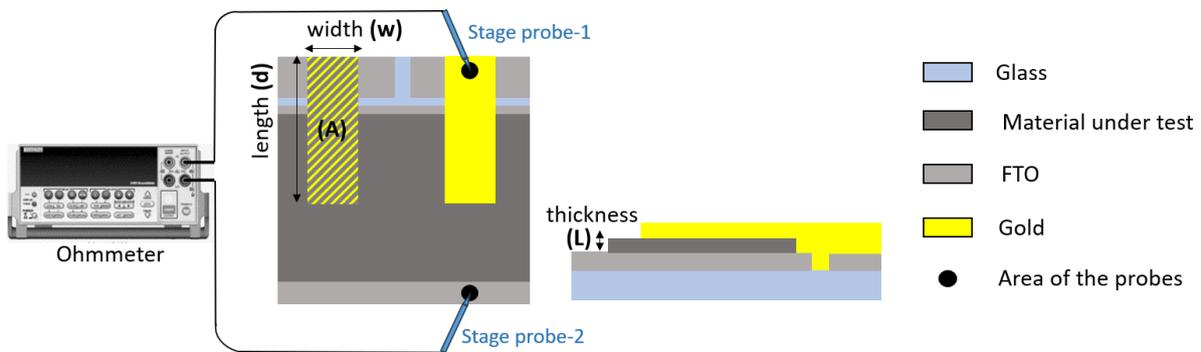
Figure III.13: The processing of two-probe method measurement with the sandwich structure configuration
