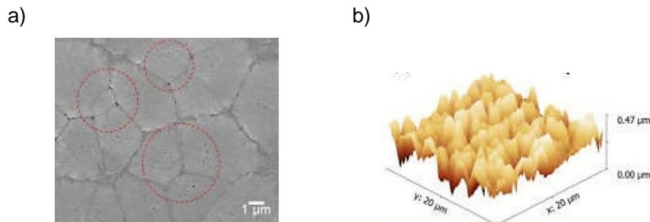
Figure I.26: The morphology of  $\text{VO}_x$ <sup>[169]</sup> with a) pin-holes and b) high roughness
