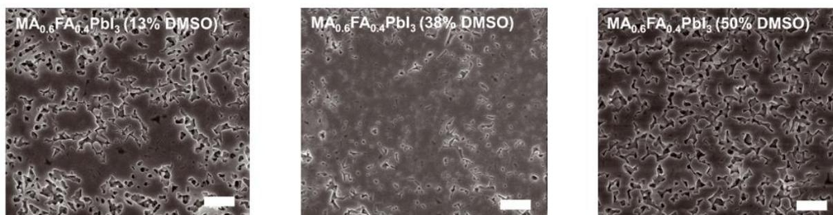
Figure I.20: Top-view SEM images of perovskite on PTAA with varying concentrations of DMSO<sup>[102]</sup>
