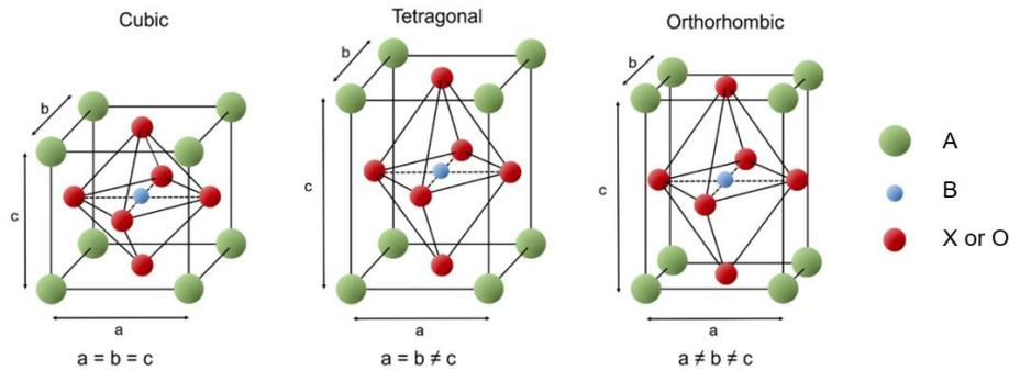
Figure I.1: Crystal structures of  $ABX_3$  perovskite<sup>[6]</sup>
