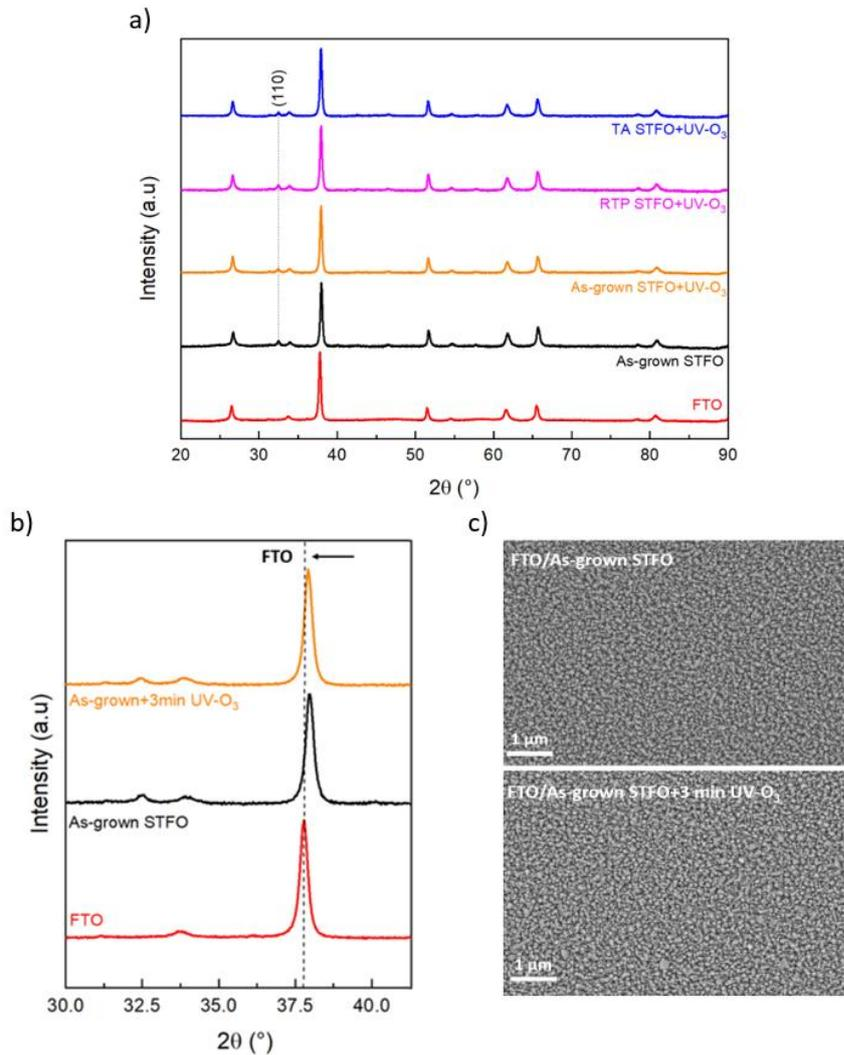
Figure V.5: a) XRD analysis of as-grown, RTP, and TA STFO thin films, b) FTO peak shift on as-grown STFO, and c) SEM images in-plane for as-grown STFO before and after UV-O<sub>3</sub>
