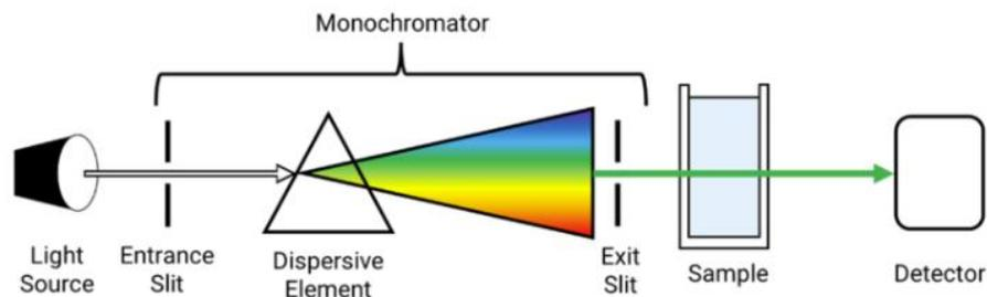
Figure A. 7: Principle of the UV-Vis spectrometer<sup>[356]</sup>
