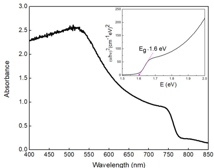
Figure IV.2 : Absorbance spectra of FA<sub>0.85</sub>Cs<sub>0.15</sub>Pb(I<sub>0.85</sub>Br<sub>0.15</sub>)<sub>3</sub> perovskite (or CsFAPbIBr) and its Tauc's plot in inset
