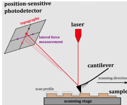
Figure A. 6: Principle of the atomic force microscopy<sup>[355]</sup>
