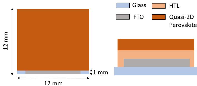
Figure IV.34 : The design and etching for quasi-2D perovskite and HTL
