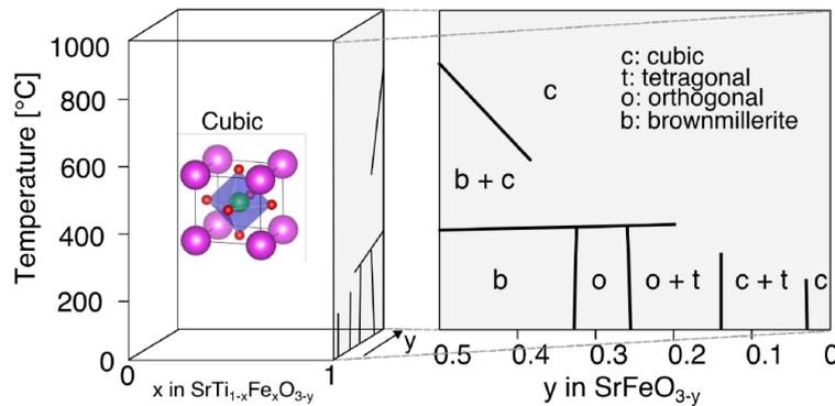
Figure II.5 :  $\text{SrTi}_{1-x}\text{Fe}_x\text{O}_{3-\delta}$ 's phase diagram with variations in temperature and composition<sup>[203]</sup>
