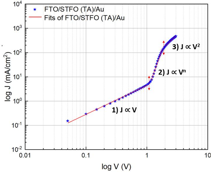
Figure III.17: Log-log scale J-V characteristics of STFO (TA)
