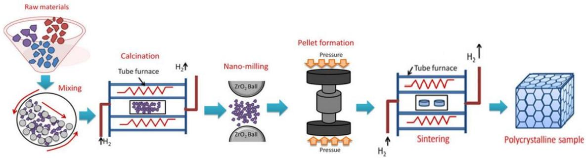
Figure II.7: The process of solid-state target synthesis<sup>[227]</sup>
