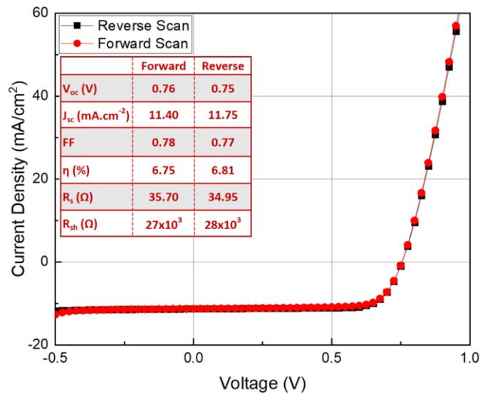
Figure IV.23: J-V characteristics of device with C<sub>60</sub> as the ETL
