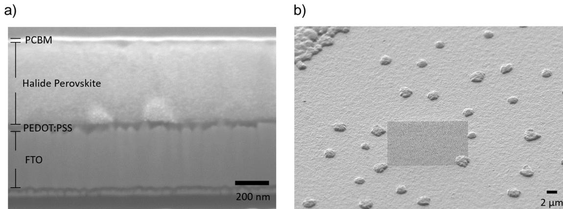
Figure IV.16 : The image of a) device with layers without top electrode and b) PC<sub>61</sub>BM surface
