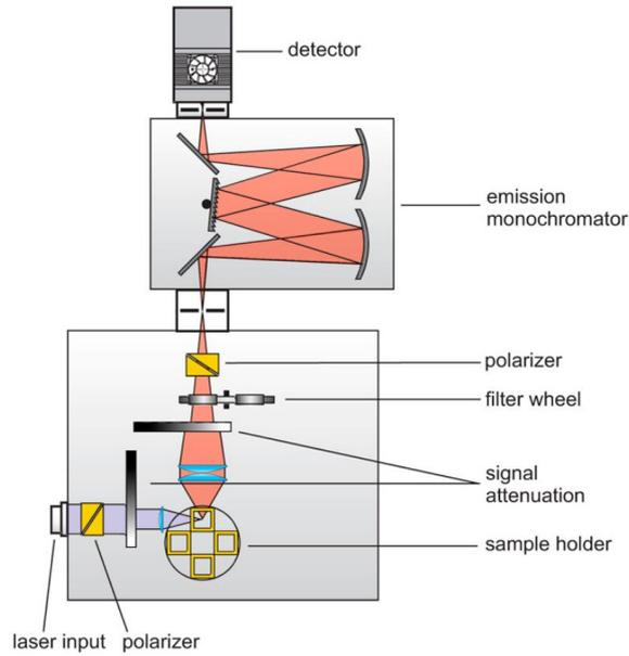
Figure A. 8: Principle of the photoluminescence spectrometer<sup>[357]</sup>
