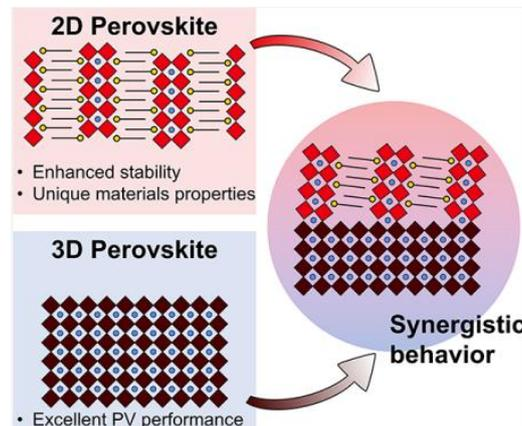
Figure I.3: The schematic of combination of favorable properties of 2D and 3D perovskites<sup>[28]</sup>
