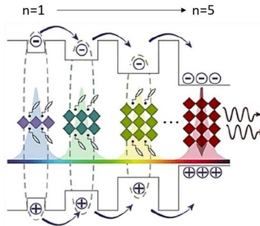
Figure I.4: Energy funneling effect in mixed phase low dimensional perovskites<sup>[33]</sup>
