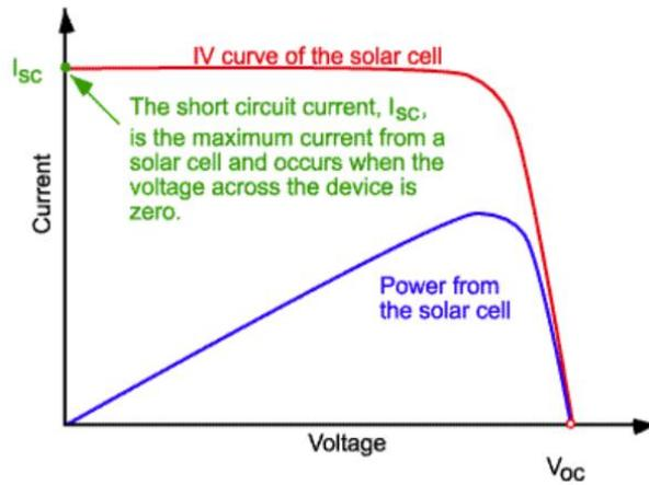
Figure I.9: Short-circuit current representing in I-V curve of the solar cell<sup>[51]</sup>
