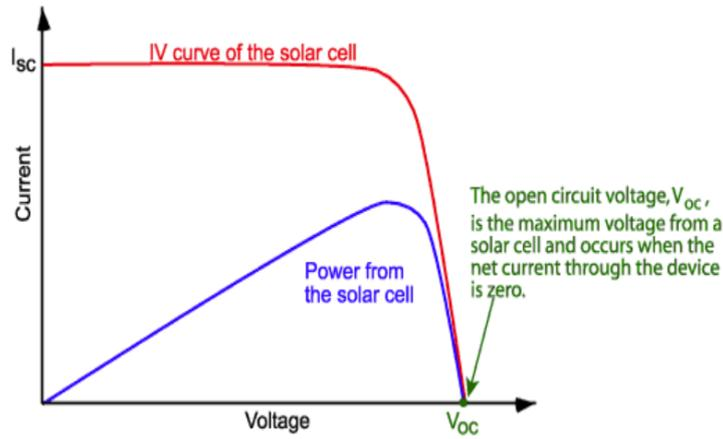
Figure I.10: Open circuit voltage representing in I-V curve of the solar cell<sup>[51]</sup>
