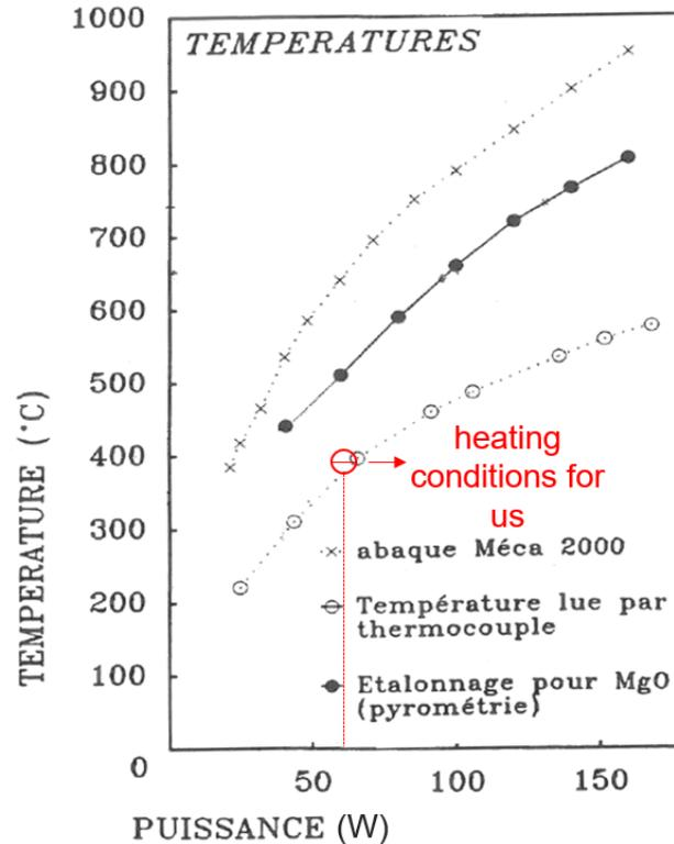
Figure A. 2: Temperature-power relation in PLD process
