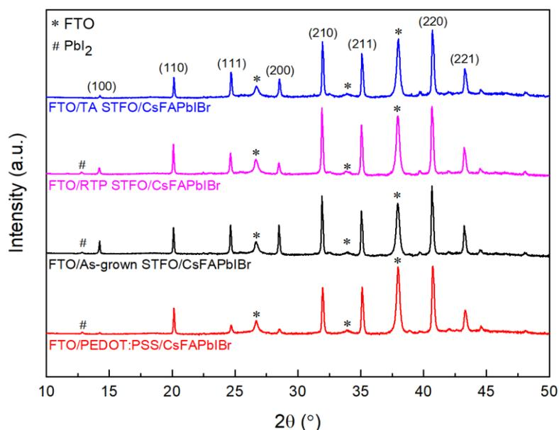
Figure V.6 : XRD pattern of CsFAPbI<sub>3</sub> perovskite layer on PEDOT:PSS, as-grown STFO, RTP STFO, and TA STFO
