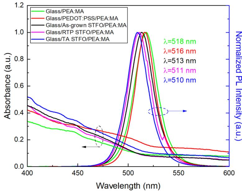
Figure V.15: UV-Vis absorbance and PL spectra of quasi-2D perovskite (PEA:MA) on PEDOT:PSS and STFO films
