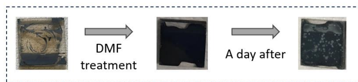
Figure IV.7 : The wettability of CuSCN and fast degradation problem of halide perovskites
