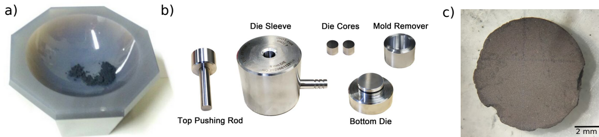
Figure 3.4 – a) Polycrystalline powder in the mortar to grind into fine powder b) Parts of the pellet die in which a small amount of powder is added and then pressed under the hydraulic press to form the pellets c) The resulting pellet of Ti_3O_5 under microscope.
