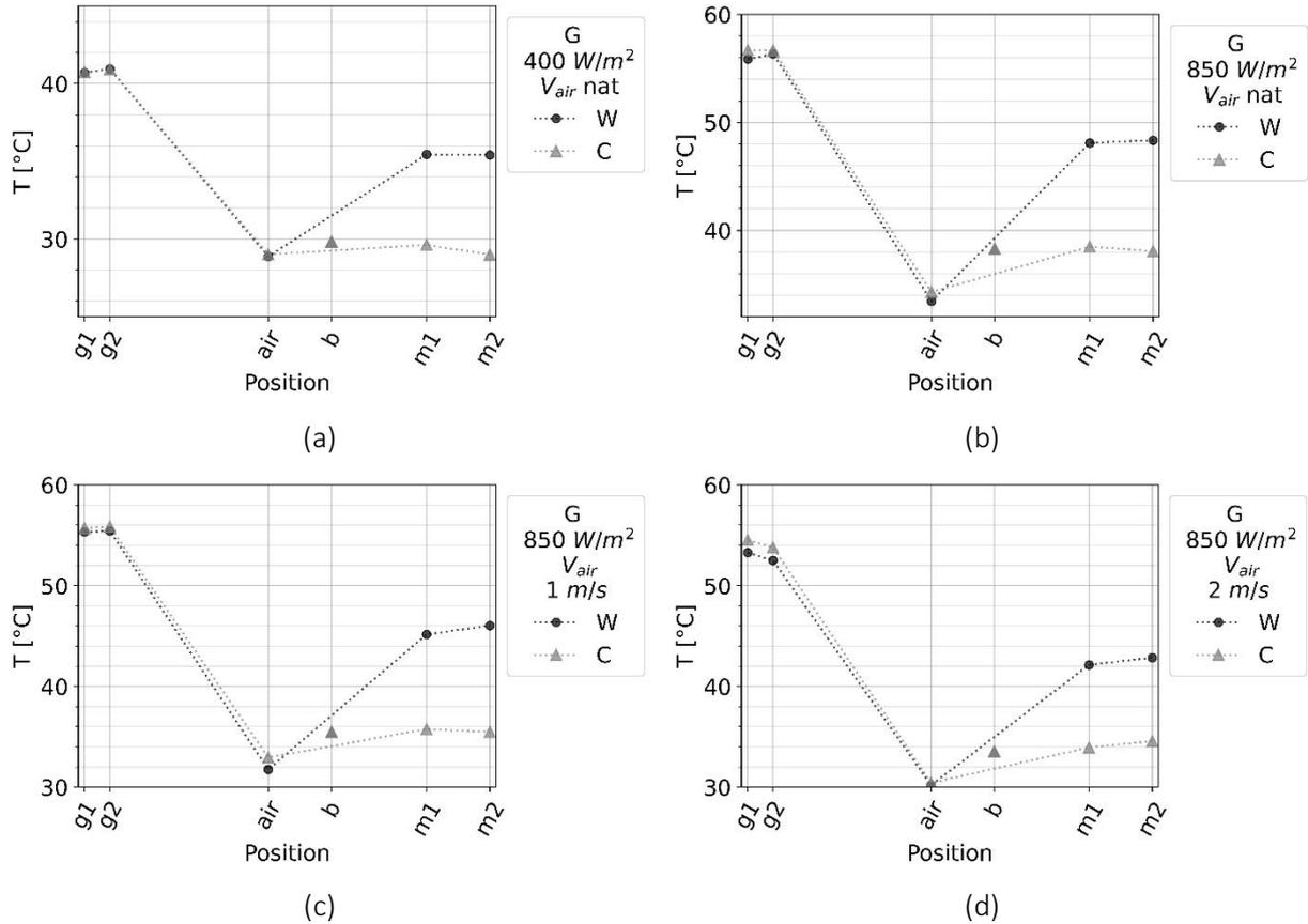
Figure IV-19: Temperatures in prototype 2 considering the configurations without bilayers (W) and with bilayers arranged in line (C) (a) with  $G = 400 \text{ W/m}^2$  and naturally ventilated air gap (b-c-d)  $G = 850 \text{ W/m}^2$  (b) and natural ventilation, (c)  $V_{air} = 1 \text{ m/s}$  (d) and  $V_{air} = 2 \text{ m/s}$
