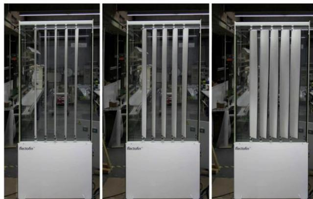
Figure I-17: Prototype of the facade shading system Flectofin® (Lienhard et al., 2011)
