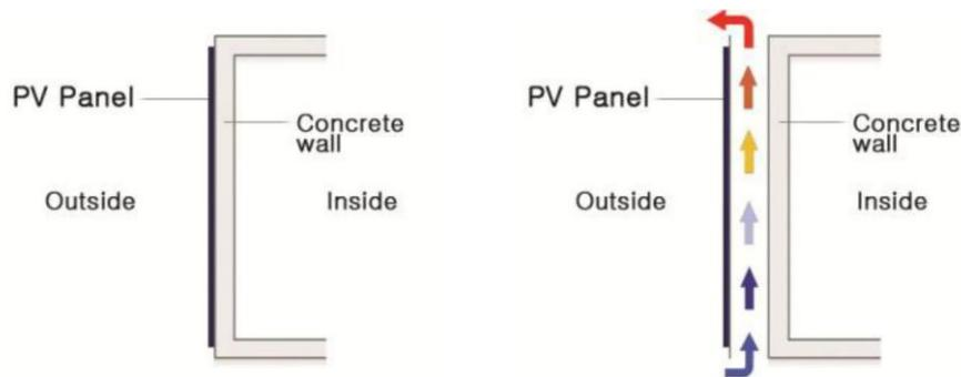
Figure I-8: Illustration of the PV facade without and with a ventilated air layer
