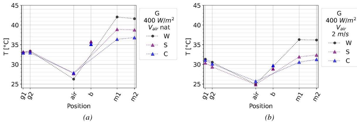
Figure IV-11: Temperatures in prototype 1 according to the bilayers arrangement for  $G = 400 \text{ W/m}^2$  (a) naturally ventilated air gap (b) air velocity at the entrance is  $V_{air} = 2 \text{ m/s}$
