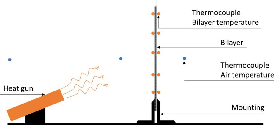
Figure III-4: Illustration of the experimental setup for the heating with a heat gun
