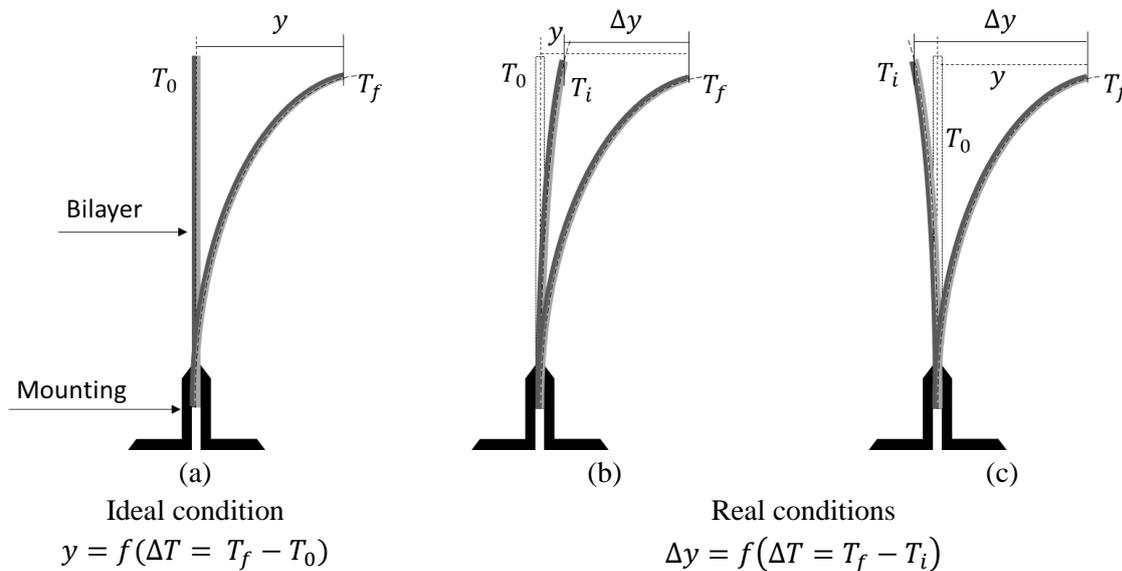
Figure III-1: Illustration of the bilayer sample with its mounting and its deformation during the experiment
