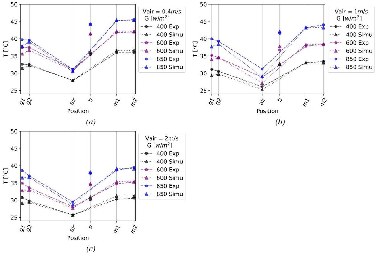
Figure V-21: Measured and simulated temperatures evolution in prototype 1 with bilayers (a) for natural ventilation in the air gap (b) for  $V_{\text{air}} = 1 \text{ m/s}$  (c) for  $V_{\text{air}} = 2 \text{ m/s}$  at the air gap entrance
