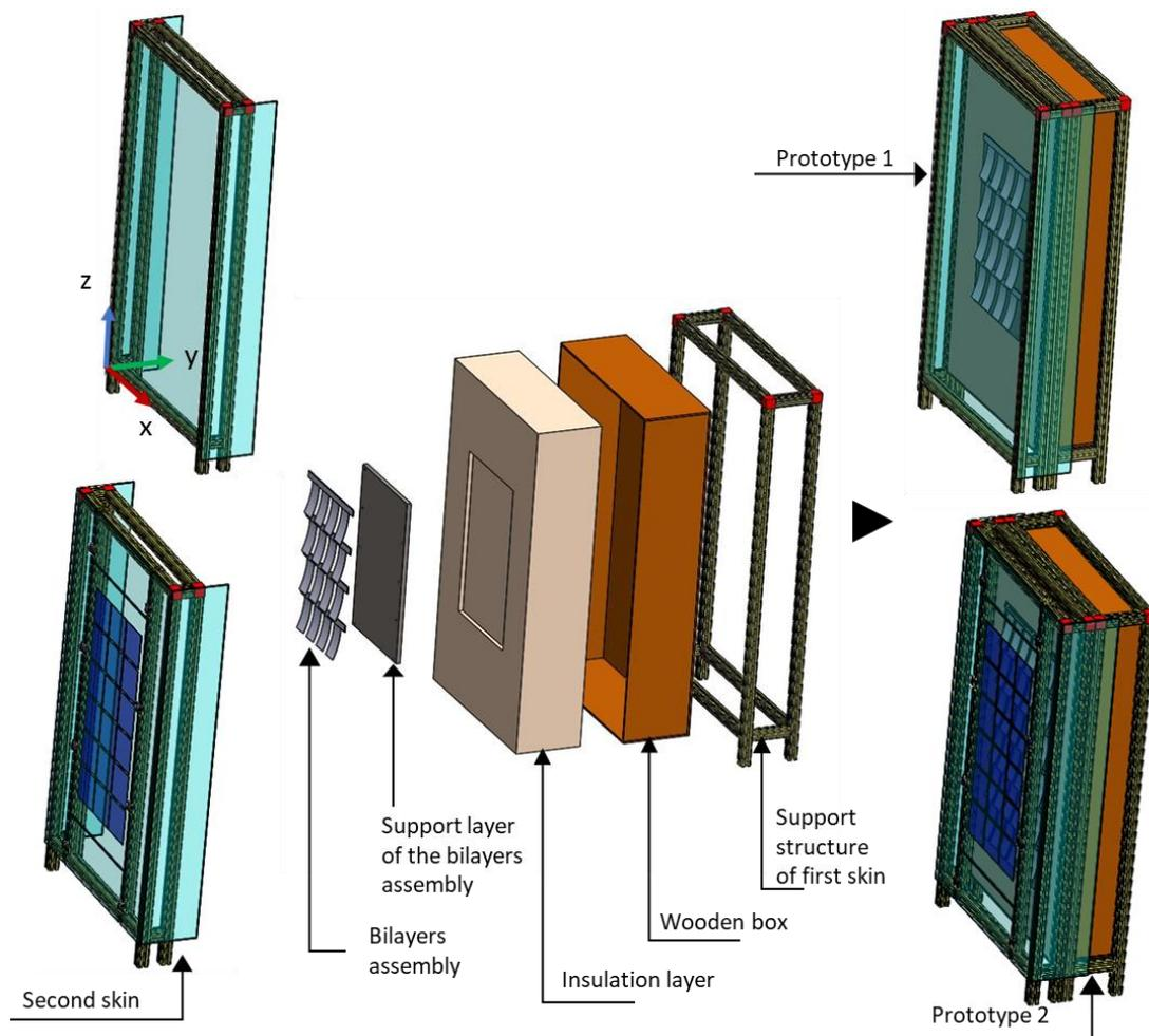
Figure IV-1: Composition of the prototypes
