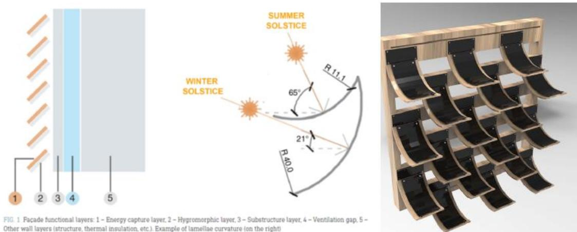
Figure I-15: Working principle of adaptive photovoltaic facade using hygromorph material (Mazzucchelli et al., 2018)
