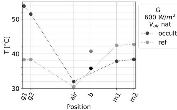
Figure IV-18: Temperatures in prototype 1 with and without dummy PV cells (occultations) for  $G = 600 \text{ W/m}^2$  and naturally ventilated air gap of 15 cm thick
