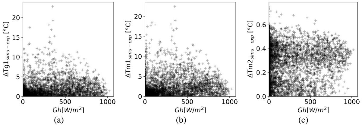
Figure V-17: Plotting of absolute difference between simulated and measured temperatures against global horizontal solar radiation (a) on the front glass of the module  $T_{g1}$  (b) on the exterior surface of the wall  $T_{M1}$  (c) on the interior surface of the wall  $T_{M2}$
