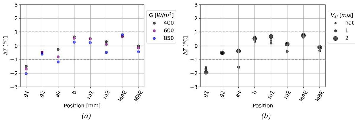
Figure V-22: Difference between the measured and simulated temperatures on the nodes of prototype 1 with bilayers (a) according to the irradiance of the solar simulator (b) according to the air velocity in the gap
