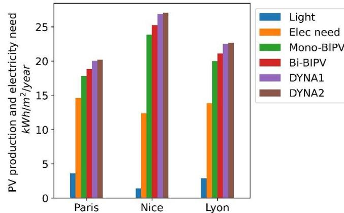
Figure VI-6: Yearly specific electricity need of the building and the PV production per conditioned area according to the facade configuration and the building implementation
