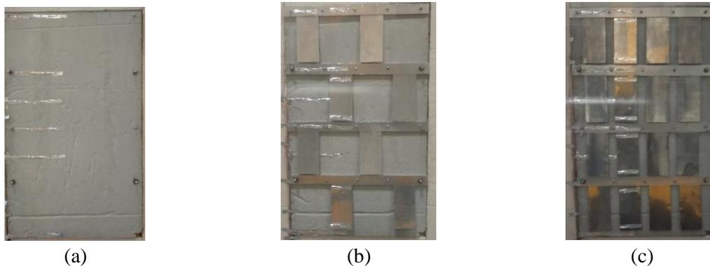
Figure IV-4: Photograph of the concrete support layer (a) without bilayers (W) (b) with the staggered arrangement (S) (c) with the in line arrangement (C)
