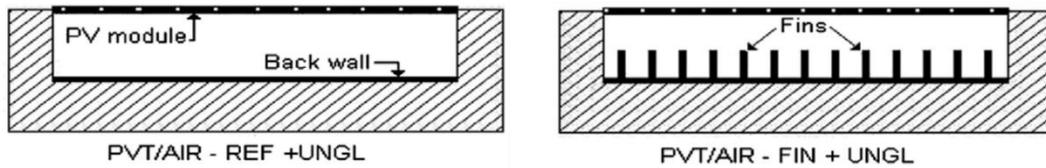
Figure I-12: Illustration of PV air-type unglazed thermal collectors with regular and optimised configuration with fins (Tonui & Tripanagnostopoulos, 2007)
