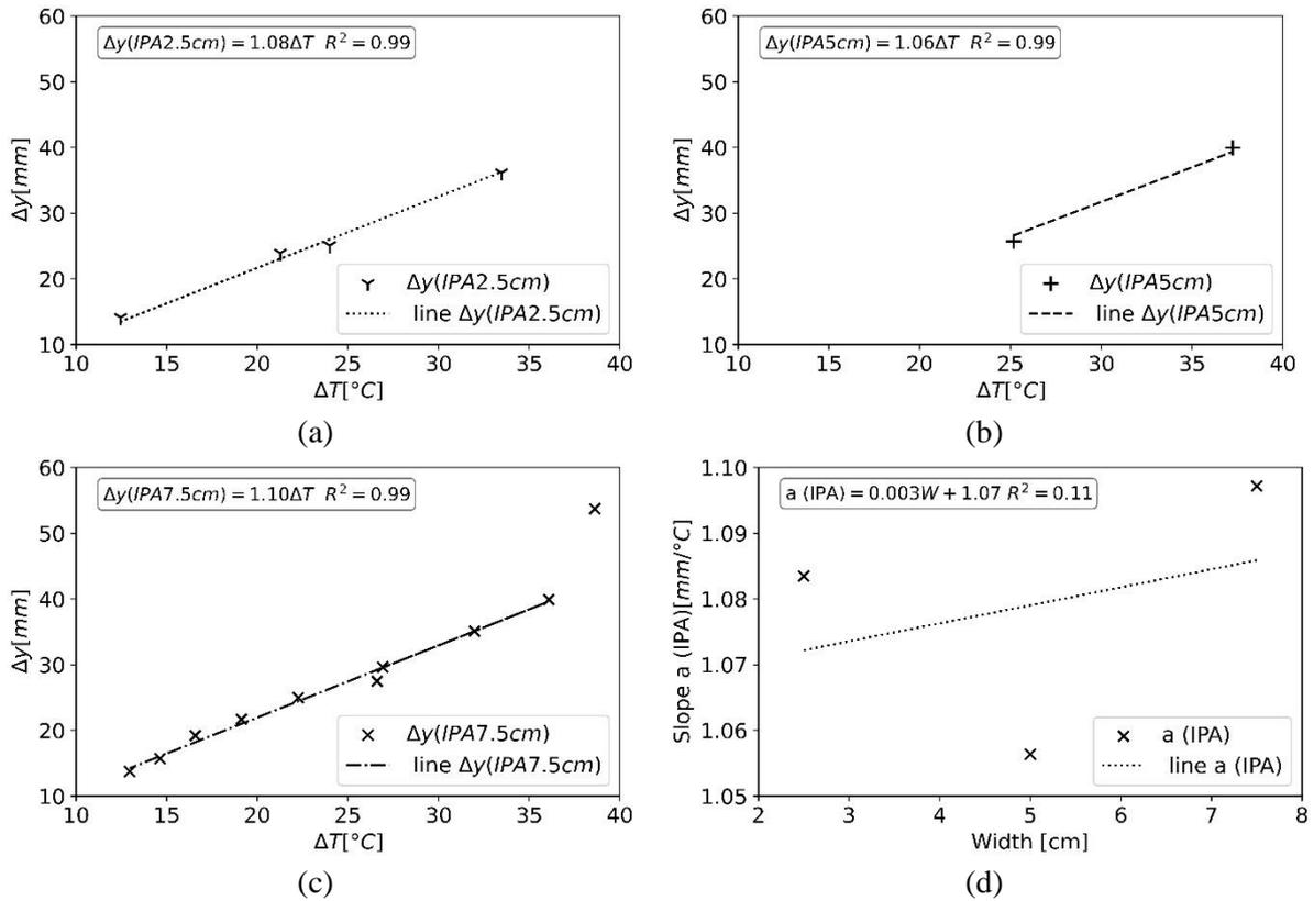
Figure III-14: Analysis of the effect of the width of the Invar-PMMA (IPA) bilayer - Displacements and their linear regression of samples of (a) 2.5 cm in width (b) 5 cm in width, and (c) 7.5 cm in width – (d) Variation of the slope according to the width of the bilayer
