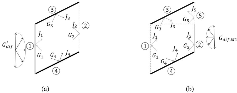
Figure V-11: Illustration of the enclosure radiation balance for the determination of (a) the front diffuse-to-diffuse (b) and the back diffuse-to-diffuse optical properties of the shading layer
