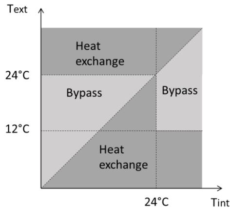
Figure VI-3: Principle of the dual flow ventilation operation
