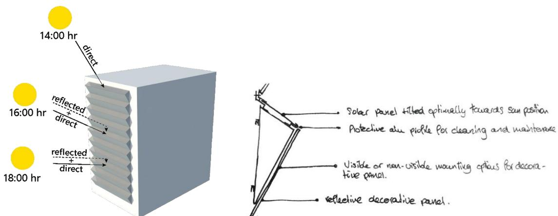
Figure I-13: Working principle of ZigZagSolar® - Source: zigzagsolar.com
