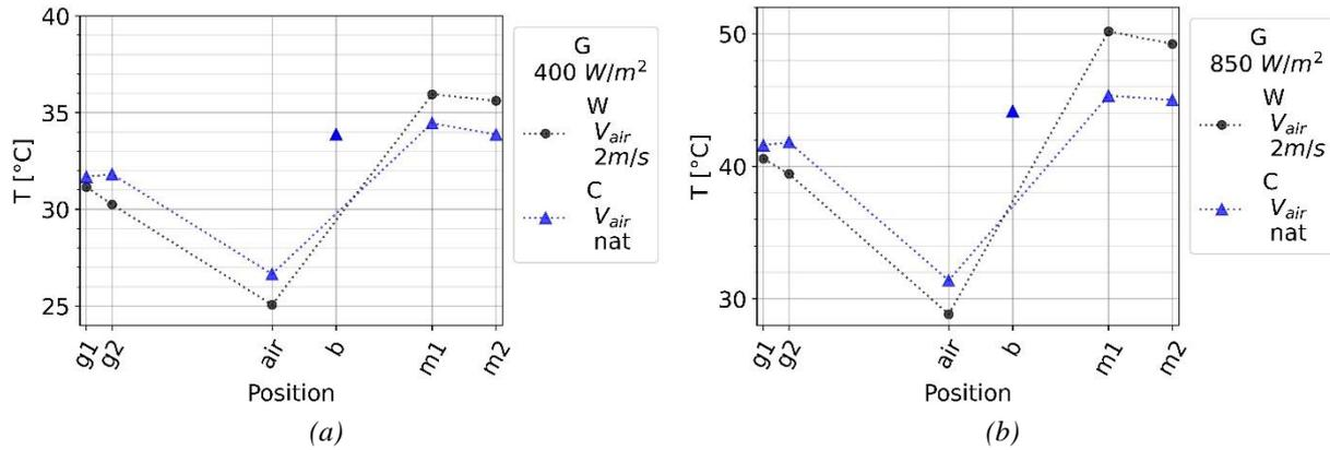
Figure IV-13: Temperatures in prototype W (without bilayers) at  $V_{air} = 2 \text{ m/s}$  and the prototype C (with bilayers arranged in line) at natural ventilation with a wooden support layer (a) for  $G = 400 \text{ W/m}^2$  (b) for  $G = 850 \text{ W/m}^2$
