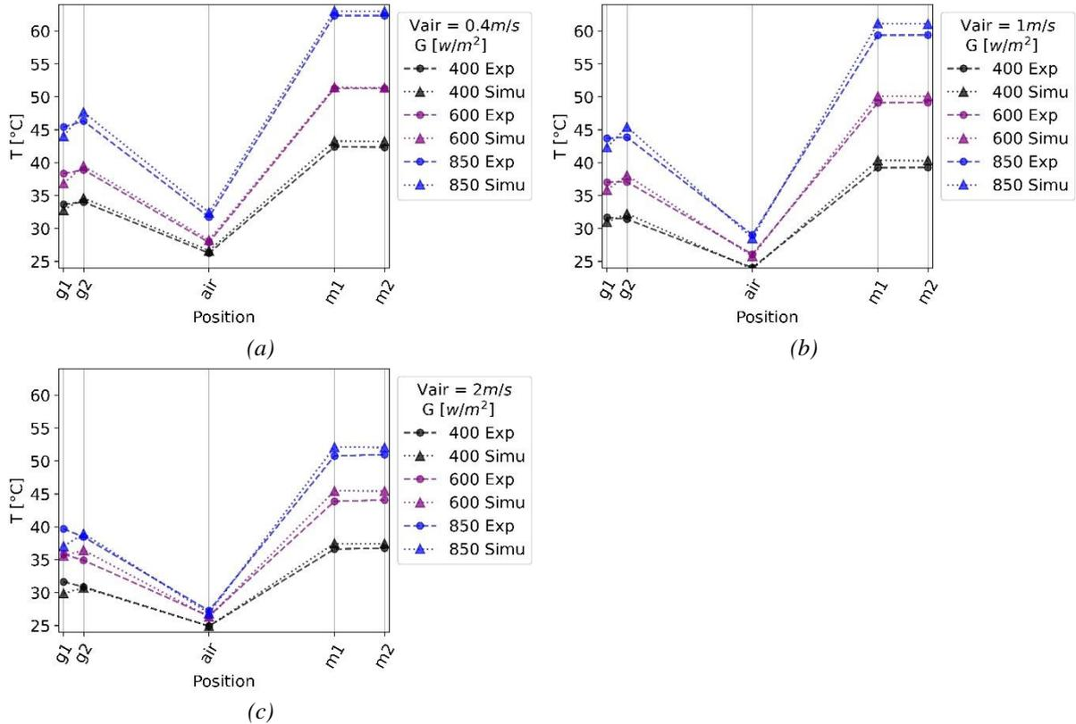
Figure V-19: Measured and simulated temperatures evolution in prototype 1 without bilayers (a) for natural ventilation in the air gap (b) for  $V_{air} = 1 \text{ m/s}$  (c) for  $V_{air} = 2 \text{ m/s}$  at the air gap entrance
