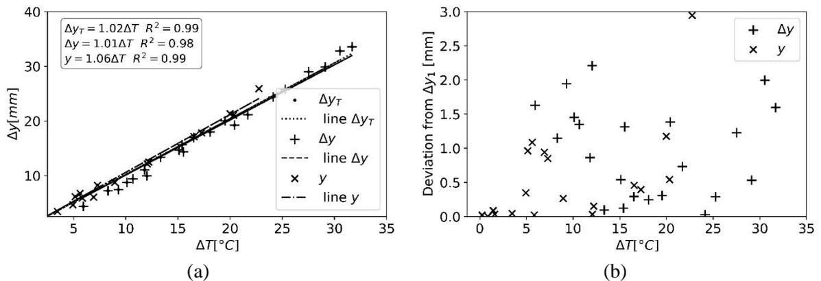
Figure III-11: Analysis of displacements of the bilayer against the temperature variation depending on the initial state of the sample with  $\Delta y_T$  for overall data –  $\Delta y$  for the measurement of the total displacement –  $y$  for the measurement of the deflection (a) Displacements and their linear regression (b) Deviation of the displacements from the predicted line of the total displacement data  $\Delta y$
