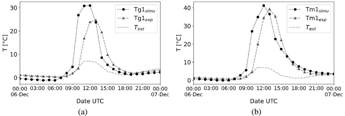
Figure V-15: Plotting of the simulated, measured and outdoor air temperatures during the day when the maximum errors occur (a) Temperature on the front glass of the module  $T_{g1}$  (b) Temperature of the exterior surface of the wall  $T_{M1}$
