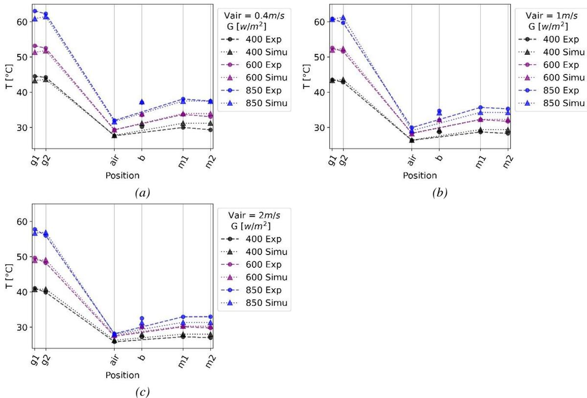
Figure V-23: Measured and simulated temperatures evolution in prototype 2 without bilayers (a) for natural ventilation in the air gap (b) for  $V_{air} = 1 m/s$  (c) for  $V_{air} = 2 m/s$  at the air gap entrance
