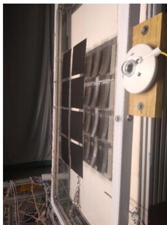
Figure IV-17: Photograph of prototype 1 with dummy PV cells
