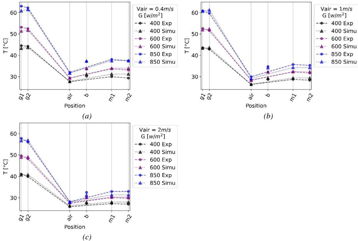
Figure V-25: Measured and simulated temperatures evolution in prototype 2 with bilayers (a) for natural ventilation in the air gap (b) for  $V_{\text{air}} = 1\text{ m/s}$  (c) for  $V_{\text{air}} = 2\text{ m/s}$  at the air gap entrance
