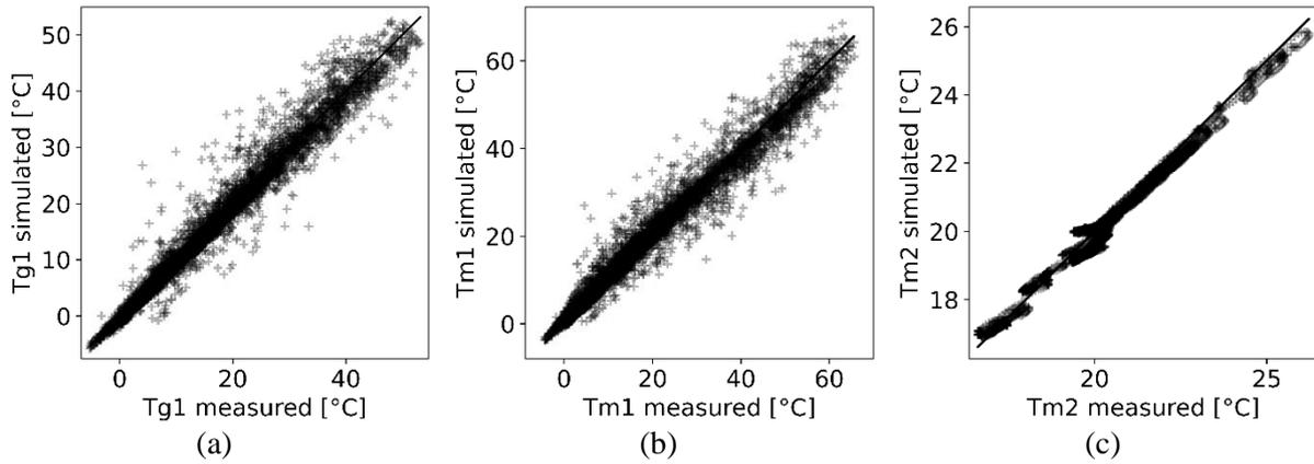
Figure V-14: Plotting of the simulated temperature against the measured temperature (a) Temperature on the front glass of the PV module  $T_{g1}$  (b) Temperature of the exterior surface of the wall  $T_{M1}$  (c) Temperature of the interior surface of the wall  $T_{M2}$
