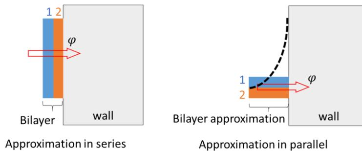
Figure II-17: Illustration of the approximation of the effective thermal conductivity of the bilayers according to the direction of the heat flow  $\varphi$  in the wall – Approximation in series for flat bilayer and approximation in parallel for deformed bilayer assumed as rectangular fin
