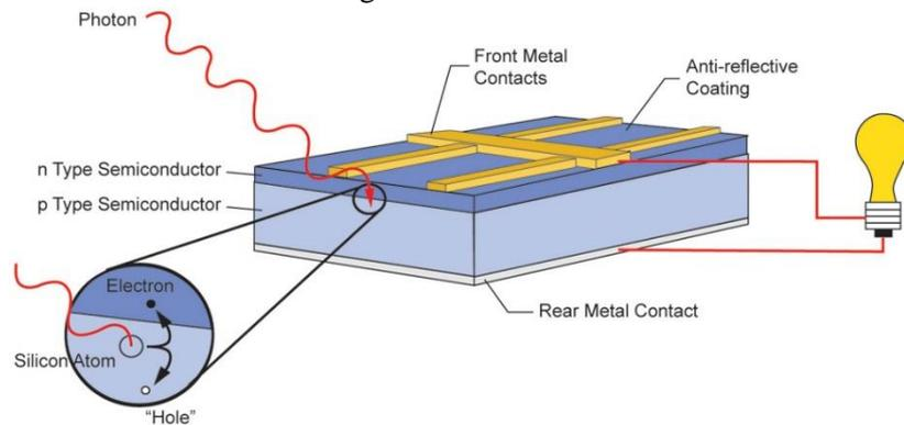
Figure I-2: Photovoltaic effect - silicon solar cell - [Source: viridiansolar.co.uk](http://viridiansolar.co.uk)
