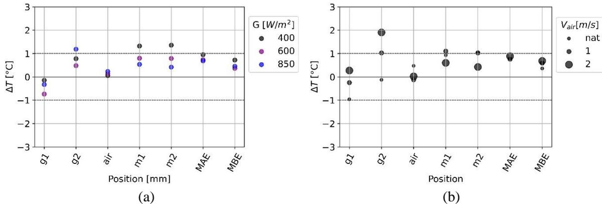
Figure V-24: Difference between the measured and simulated temperatures on the nodes of prototype 2 without bilayers (a) according to the irradiance of the solar simulator (b) according to the air velocity in the gap
