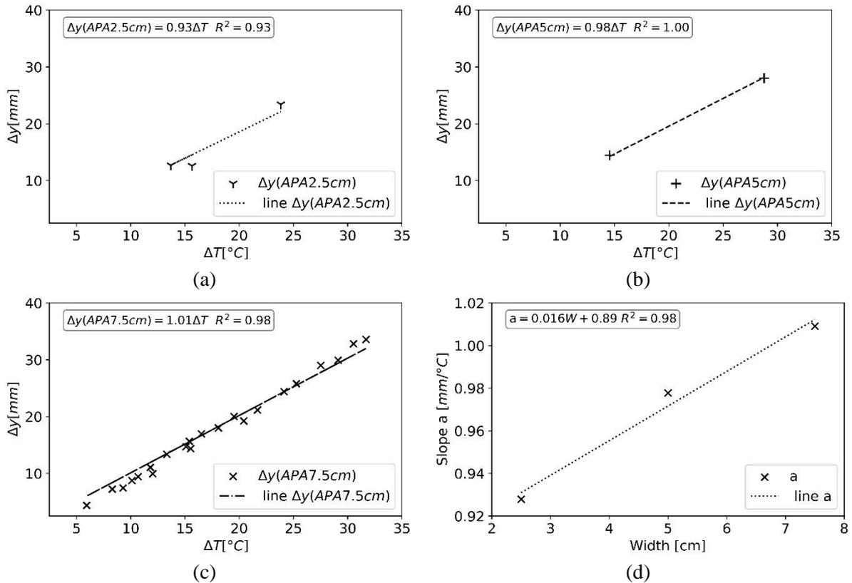
Figure III-12: Analysis of the effect of the width of the Aluminium-PMMA (APA) bilayer - Displacements and their linear regression of samples of (a) 2.5 cm in width (b) 5 cm in width, and (c) 7.5 cm in width – (d) Variation of the slope according to the width of the bilayer
