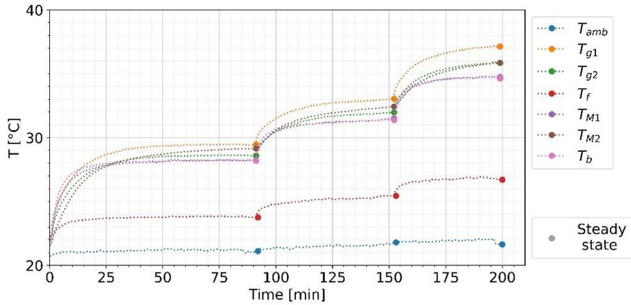
Figure IV-9: Staircase mean temperature evolution at each surface with the value at steady state - series of tests on prototype 1 with insulation support layer at  $V_{air} = 2 \text{ m/s}$  and  $G = 400 \text{ W/m}^2$ ,  $600 \text{ W/m}^2$ ,  $850 \text{ W/m}^2$  on each step
