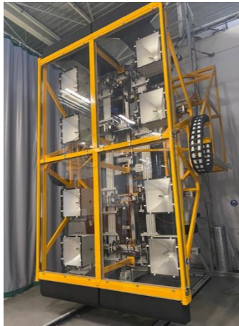
Figure IV-6: Photograph of the vertical position of the solar simulator set for the test campaign
