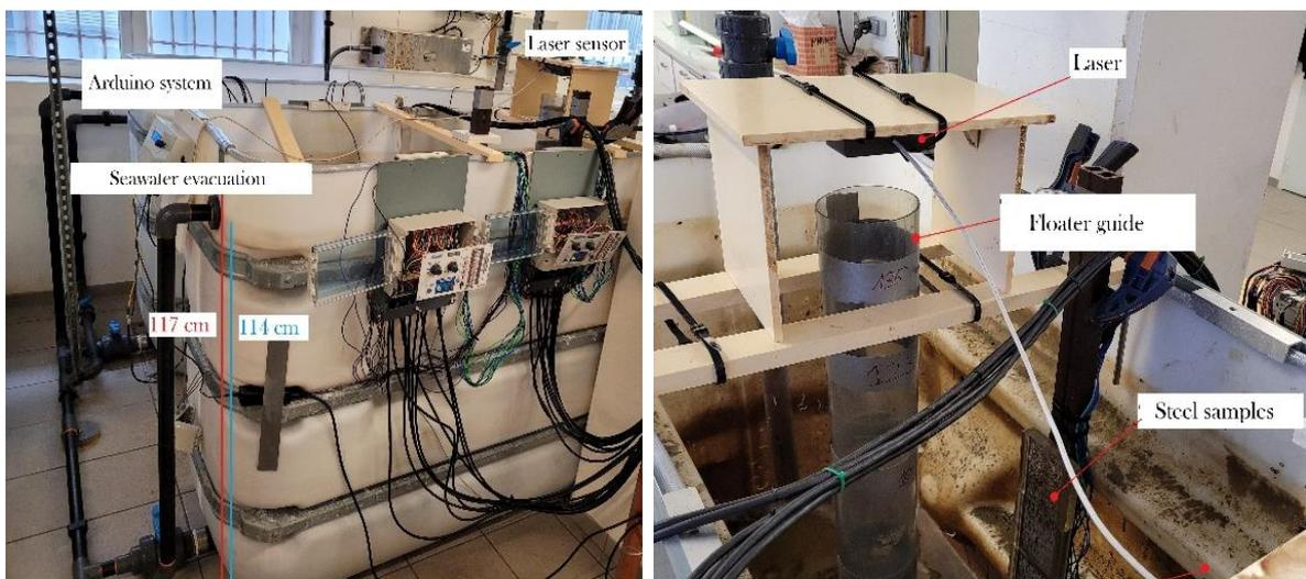
Figure V.3: Photographs of the experimental set up
