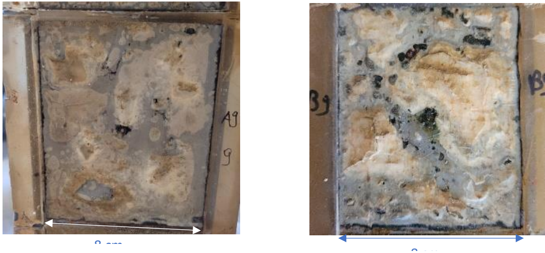
Figure V. 21: Visual observation of the lower coupon from column A (on the left) and B (on the right)
