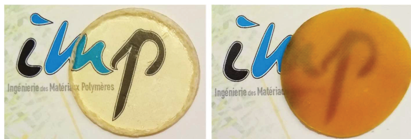
Figure 3. Photographs of C1608/T403 (left) and C67/T403 (right) compounds in the form of 1 mm-thick discs
