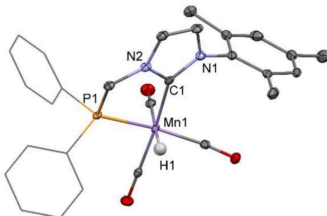
**Figure 3.** Structure moléculaire du complexe *fac*-**C1.a** (30% probability ellipsoïds, aryl groups represented as a wireframe for clarity). Selected bond lengths (Å) and angles (°): Mn1–C1 2.034(3), Mn1–P1 2.2371(9), Mn1–H1 1.63(4), C1–Mn1–P1 79.95(9), C1–Mn1–H1 81.0(14), P1–Mn1–H1 78.5(14).
