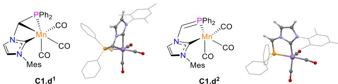
**Figure 6.** Structures and DFT optimized geometries of complexes **C1.d**<sup>1</sup> and *fac*-**C1.d**<sup>2</sup> (BP86/def2-TZVP, toluene SMD model).
