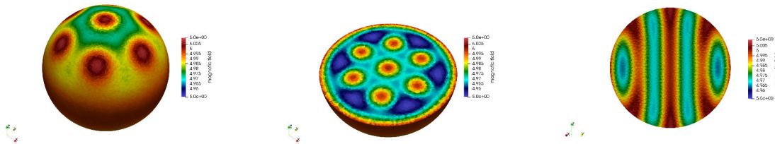
Figure 3.26. Example 3. Magnetic field \nabla \times \mathbf{A} (left), section of the magnetic field along the equatorial plane (middle), magnetic field \nabla \times \mathbf{A} along the z -axis (right).
