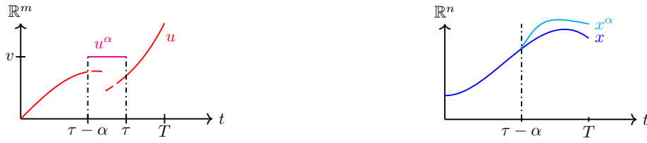
Figure 2.4: Illustrations of a needle-like perturbation (left) and the corresponding perturbed trajectory (right).
