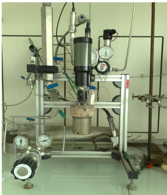
**Figure 1.** Hastelloy<sup>®</sup> B2 100 mL reactor for batch experiments (TOP INDUSTRIE).
