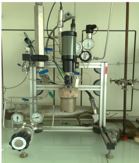
Figure 1. Hastelloy ® B2 100 mL reactor for batch experiments (TOP INDUSTRIE).
